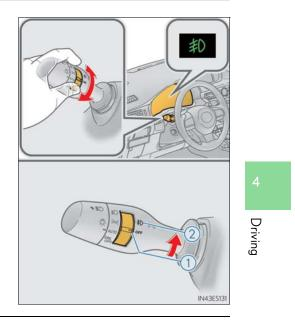
■ Fog lights can be used when The headlights are on in low beam.
