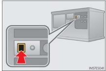
Press and hold the desired HomeLink<sup>®</sup> button (inside the vehicle) for 2 seconds and release it. Repeat this sequence (press/hold/release) up to 3 times to complete programming.
