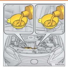
**6** Start the hybrid system and turn the air conditioning system on to check that the radiator cooling fans operate and to check for coolant leaks from the radiator or hoses.
