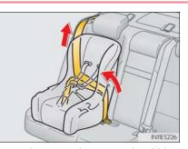
**6** If the child restraint has a top tether strap, the top tether strap should be latched onto the top tether strap anchor.  $(\rightarrow P. 63)$
