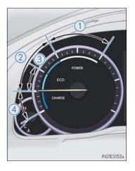
Hybrid System Indicator is displayed when the driving mode is other than the sport mode.
