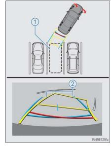
3 When the rear position of the vehicle has entered the parking space, turn the steering wheel so that the vehicle width guide lines are within the left and right dividing lines of the parking space.
