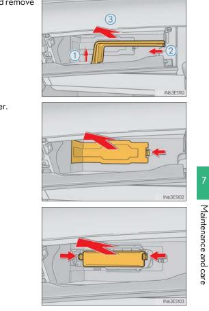
**5** Slide and pull out the filter. Replace it with a new one.
