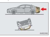
The SRS curtain shield airbags do not generally inflate if the vehicle is involved in a rear collision, if it pitches end over end, or if it is involved in a low-speed side or low-speed frontal collision.
