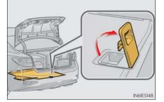
**2** The lever can be hooked on the edge of the trunk.
