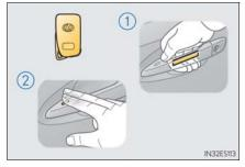
② Touch the lock sensor (the indentation on the upper part of the door handle) to lock all the doors.
