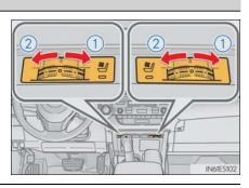
The seat heaters and ventilators can be used when the power switch is in ON mode.
