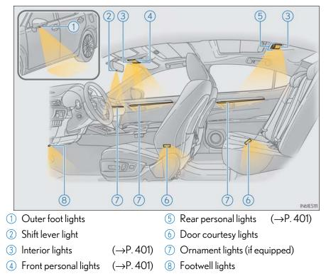
When the instrument panel light control switch is turned to minimum and the tail lights are on, the ornament lights and the footwell lights will turn off. ( $\rightarrow$ P. 87)
