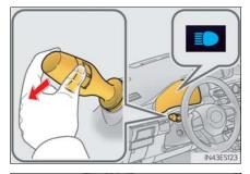
**2** Press the Automatic High Beam switch.
