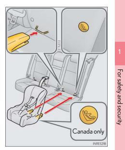
Installing child restraints using a seat belt (child restraint lock function belt)
