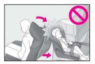
Adjust the front passenger seat so that it does not interfere with the child restraint system.
