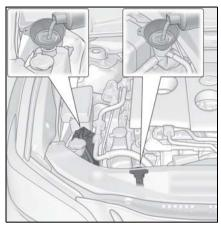
Start the hybrid system and turn the air conditioning system on to check that the radiator cooling fan operates and to check for coolant leaks from the radiator or hoses.
