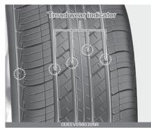
This shows there is less than 1.6 mm of tread left on the tire. Replace the tire when this happens.
