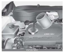
Check if the oil level is between the F-L line and refill it if the oil level is near the L line.
