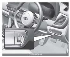
To adjust the headlight beam level according to the number of the pas<sup>-</sup> sengers and loading weight in the luggage area, turn the beam leveling switch.
