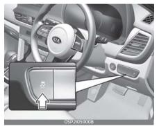
ESC applies the brakes on individual wheels and intervenes with the vehicle management system to sta<sup>-</sup> bilize the vehicle.
