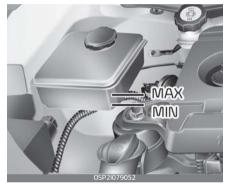
8. If the coolant level is low, add enough specified coolant to provide protection against freezing and corrosion. Bring the level to F, but do not overfill.
