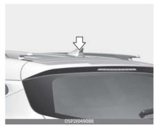
The shark fin antenna will receive the transmitted data.
