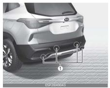
This system is a supplemental sys<sup>-</sup> tem and it is not intended to nor does it replace the need for extreme care and attention of the driver. The sensing range and objects detect<sup>-</sup> able by the back sensors (1) are lim<sup>-</sup> ited. Whenever backing-up, pay as much attention to what is behind you as you would in a vehicle with<sup>-</sup> out a Reverse Parking Distance Warning.
