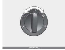
Air can be directed to the floor, dashboard outlets, or windshield. Five symbols are used to represent Face, Bi-Level, Floor, Floor-Defrost and Defrost air position.
