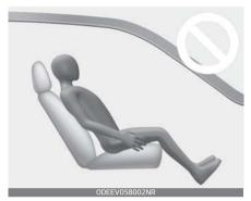
Riding in a vehicle with a front seat<sup>-</sup> back reclined could lead to serious or fatal injury in an accident. If a front seat is reclined during an accident, the occupant's hips may slide under the lap portion of the seat belt applying great force to the unpro<sup>-</sup> tected abdomen. Serious or fatal internal injuries could result. The driver must advise the front pas<sup>-</sup> senger to keep the seatback in an upright position whenever the vehi<sup>-</sup> cle is in motion.
