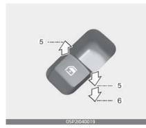
Pressing the power window switch momentarily to the second detent position (6) completely lowers the window even when the switch is released. To stop the window at the desired position while the window is in operation, pull up the switch briefly to the opposite direction of the window movement.
