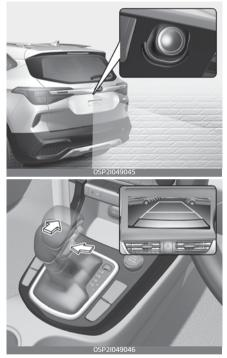
Rear View Monitor with parking guidance will activate when the engine is running and the shift lever is in the R (Reverse) position.
