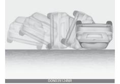
Air bags may not inflate if the vehicle collides with objects such as utility poles or trees, where the point of impact is concentrated to one area and the full force of the impact is not delivered to the sensor.
