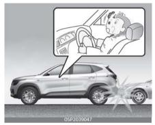
Front air bags may not inflate in side impact collisions, because occupants move to the direction of the collision, and thus in side impacts, frontal air bag deploy<sup>-</sup> ment would not provide additional occupant protection.
