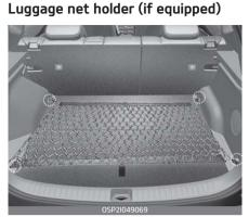
To keep items from shifting in the cargo area, you can use the 4 hold<sup>-</sup> ers located in the cargo area to attach the luggage net.
