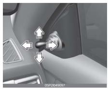
To adjust an outside mirror, move the control lever located at the forward inside area of the window frame.
