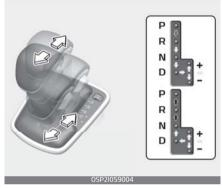
Depress the brake pedal and the lock release button when shift<sup>-</sup> ing.
