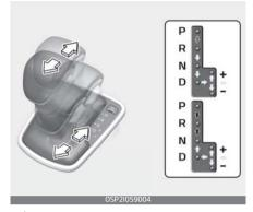
✓ Depress the brake pedal and the lock release button when shift<sup>−</sup> ing.
