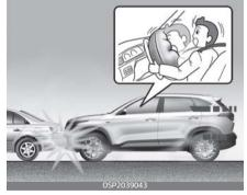
Front air bags are designed to inflate in a frontal collision depending on the intensity, speed or angles of impact of the front collision.
