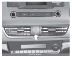
It should be used whenever emergency repairs are being made or when the vehicle is stopped near the edge of a roadway. Depress the flasher switch with the ignition switch in any position. The flasher switch is located in the cen<sup>-</sup> ter console switch panel. All turn signal lights will flash simultane<sup>-</sup> ously.
