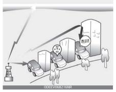
AM and FM radio signals are broad<sup>-</sup> cast from transmitter towers located around your city. They are intercepted by the radio antenna on your vehicle. This signal is then pro<sup>-</sup> cessed by the radio and sent to your vehicle speakers.
