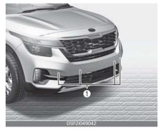
The sensing range and objects detectable by the sensors (1) are limited. Whenever moving while using Forward/Reverse Parking Dis<sup>-</sup> tance Warning, pay as much atten<sup>-</sup> tion to what is in front and behind you as you would in a vehicle with<sup>-</sup> out Forward/Reverse Parking Dis<sup>-</sup> tance Warning.
