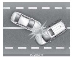
Just before impact, drivers often brake heavily. Such heavy braking lowers the front portion of the vehicle causing it to "ride" under a vehicle with a higher ground clearance. Air bags may not inflate in this "under-ride" situa<sup>-</sup> tion because deceleration forces that are detected by sensor may be significantly reduced by such "under-ride" collisions.
