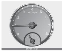
The tachometer indicates the approximate number of engine rev<sup>-</sup> olutions per minute (rpm).
