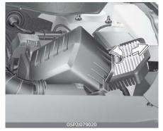
Lock the cover with the cover attaching clips.
