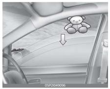
If the upward movement of the window is blocked by an object or part of the body, the window will detect the resistance and will stop upward movement. The window will then lower approximately 30 cm (11.8 in) to allow the object to be cleared.
