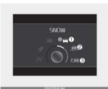
If you press the "DRIVE/TRACTION" mode button, the driving mode is changed from Driving control to Traction control. You can select SNOW (1), MUD (2) or SAND (3) mode by rotation the knob. If you press the "DRIVE/TRACTION" mode button again, the driving mode is changed from Traction Control to previous driving control. The driving mode will be set to Driving control when the restarted, If it is in Traction Control.
