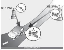
Multi-Path Cancellation – Radio signals being received from sev<sup>-</sup> eral directions can cause distor<sup>-</sup> tion or fluttering. This can be caused by a direct and reflected signal from the same station, or by signals from two stations with close frequencies. If this occurs, select another station until the condition has passed.
