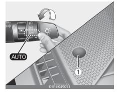
When the light switch is in the AUTO light position, the taillights and headlights will turn ON or OFF auto<sup>-</sup> matically depending on the amount of light outside the vehicle.
