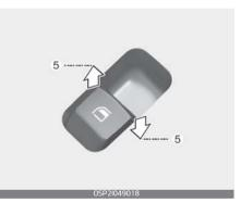
To open or close a window, press down or pull up the front portion of the corresponding switch to the first detent position (5).
