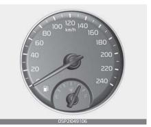
The speedometer indicates the speed of the vehicle and is cali<sup>-</sup>
