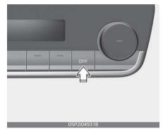
Press the OFF button to turn off the air climate control system.
