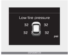
The low tire pressure position tell<sup>-</sup> tale light will indicate which tire is significantly under-inflated by illu<sup>-</sup> minating the corresponding position light.
