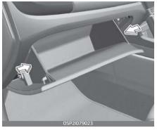
3. Remove the climate control air filter cover by pulling out right side of the cover.
