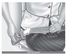
• When you want to release the seat belt, press the button (1) in the locking buckle.
