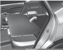
2. Make sure the seatback is locked in place. When you return the seatback to its upright position, always be sure it has locked into position by pushing on the top of the seatback.
