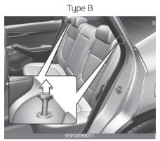
1. Pull up both sides of the seatback folding lever.
