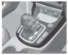
Whether the vehicle is stationary or in motion, sports mode is selected by pushing the shift lever from the D (Drive) position into the manual gate. To return to D (Drive) range operation, push the shift lever back into the main gate. SPORT mode manages the driving dynamics by automatically adjusting the steering effort, and the engine and transmission control logic for enhanced driver performance.
