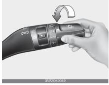
When the light switch is in the position lamp position, the front position lamp and auxiliary lamp (if equipped), tail, license light will turn ON.
