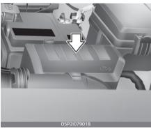
You can clean the filter when inspecting the air cleaner compart<sup>-</sup> ment. Clean the filter by using com<sup>-</sup> pressed air.
