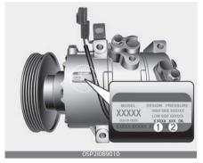
A compressor label informs you the type of compressor your vehicle is equipped with such as model, sup<sup>-</sup> plier part number, production num<sup>-</sup> ber, refrigerant (1) and refrigerant oil (2).
