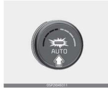
Turn the temperature control switch to the desired tempera<sup>-</sup> ture.
