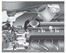
Do not overfill. Use a funnel to help prevent oil from being spilled on engine components. Use only the **specified engine oil.** (Refer to "Recommended lubricants and capacities" on page 9–7.)
