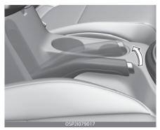
Check the stroke of the parking brake by counting the number of "clicks" heard while fully applying it from the released position.
