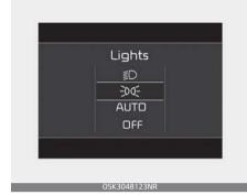
This indicator displays which exte rior light is selected using the light<sup>-</sup> ing control.
