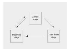
This system is operated in three stages:
