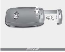
To pull out the mechanical key:
