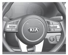
The horn will operate only when this area is pressed. Check the horn reg<sup>-</sup> ularly to be sure it operates prop<sup>-</sup> erly.
