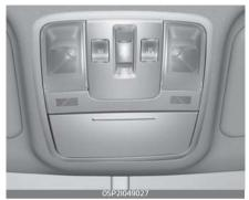
The sunroof can be operated for approximately 10 minutes after the ENGINE START/STOP button is turned to the ACC or LOCK position. However, if the front doors are opened, the sunroof cannot be opened even within the 10 minutes period.
