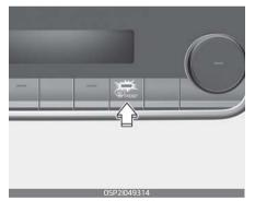
Most of the air flow is directed to the windshield with a small amount of air directed to the side window defrosters and side air vents.
