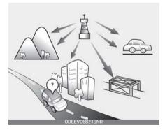
FM broadcasts are transmitted at high frequencies and do not bend to follow the earth's surface. Because of this, FM broadcasts generally begin to fade within short distances from the station. Also, FM signals are easily affected by buildings, mountains, and obstructions. This can lead to undesirable or unpleas<sup>-</sup> ant listening conditions which might lead you to believe a problem exists with your radio.
