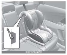
1. Route the Child Restraint System top-tether strap over the seat<sup>-</sup> back. Placing the top tether strap, please follow the instructions of the Child Restraint System manu<sup>-</sup> facturer. 2. Connect the top-tether strap to the top-tether anchorage, then tighten the top-tether strap according to the instructions of your Child Restraint System's manufacturer to firmly attach the Child Restraint System to the seat.
