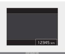
The odometer Indicates the total distance that the vehicle has been driven and should be used to deter<sup>-</sup> mine when periodic maintenance should be performed.
