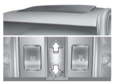
To open the sunroof, push the sunroof control lever upward until the sunroof moves to the desired position.
