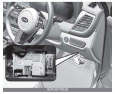
3. Pull the suspected fuse straight out. Use the removal tool pro<sup>-</sup> vided on the engine fuse panel cover.
