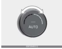
The temperature will increase to the maximum (HI) by rotating the knob clockwise direction.
