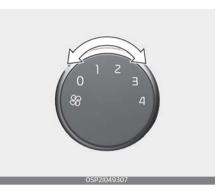
• Setting the fan speed control knob to the "O" position turns off the fan.
