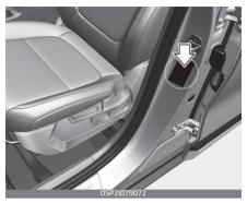
The vehicle certification label attached on the driver's (or front passenger's) side center pillar gives the vehicle identification number (VIN).
