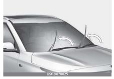
To replace wiper blade, lift the arm first and replace the wiper blade as per procedure.
