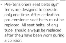
The pre-tensioner seat belt assembly mechanisms become hot during activation. Do not touch the pre-tensioner seat belt assemblies for several minutes after they have been activated.
