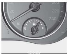
This gauge indicates the approxi<sup>-</sup> mate amount of fuel remaining in the fuel tank.
