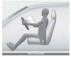
Upon deployment, tear seams molded directly into the pad covers will separate under pressure from the expansion of the air bags. Fur<sup>-</sup> ther opening of the covers then allows full inflation of the air bags.
