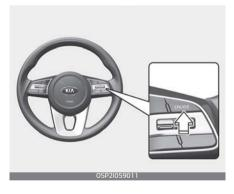
2. Accelerate to the desired speed, which must be more than 30 km/ h.
