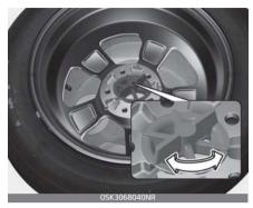
Turn the tire hold-down wing bolt counterclockwise to remove.
