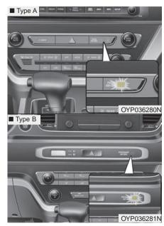
Your vehicle is equipped with an occupant detection system in the front passenger's seat.
