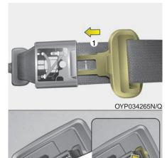
3. Insert the tongue plate into the holder (1) in seat belt and then insert the mini tongue into the hole on the belt assembly cover.
