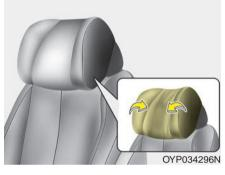
For rear outboard passenger's comfort, the ends of the headrest can be adjusted inward.
