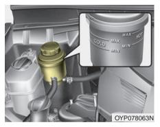
With the vehicle on level ground, check the fluid level in the power steering reservoir periodically. The fluid should be between MAX and MIN marks on the side of the reservoir at the normal temperature.
