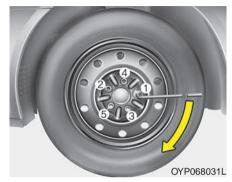
Then position the tool as shown in the drawing and tighten the wheel nuts. Be sure the socket is seated completely over the nut. Do not stand on the tool handle or use an extension pipe over the tool handle. Go around the wheel tightening every nut following the numerical sequence shown in the image until they are all tight. Then double-check each nut for tightness. After changing wheels, have an authorized Kia dealer tighten the wheel nuts to their proper torque as soon as possible.
