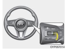
Move the lever down (to SET-), and release it at the desired speed. The SET indicator light in the instrument cluster will illuminate. Release the accelerator at the same time. The desired speed will automatically be maintained.
