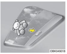
If an object or part of the body is detected while the sunroof is closing automatically, it will reverse direction, and then stop.
