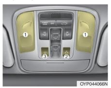
Press the lens (1) to turn the map lamp on or off.
