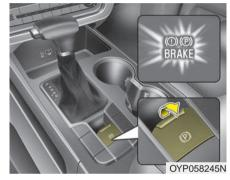
To apply the EPB (electronic parking brake):
