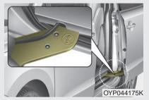
When getting in and out of the sliding door, do not step on the sliding door hinge or drop or put heavy objects on the hinge. The door may not open or close normally if the door hinge or wire is damaged.
