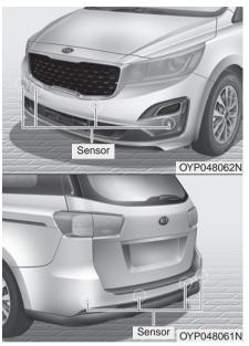
The parking distance warning assists the driver during movement of the vehicle by chiming if any object is sensed within the distance of 100 cm (39 in) in front or behind the vehicle. The sensing range and objects detectable by the sensors are limited. Whenever moving, pay as much attention to what is in front and behind of you as you would in a vehicle without a parking distance warning.
