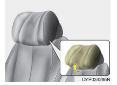
The headrest may be adjusted forward or backward by pulling the lower part of the headrest forward or backward to the desired detent in the direction of the arrow. Adjust the headrest so that it properly supports the head and neck. Wing-out (2nd row seat for SXL package)
