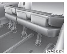
Make sure the catches are locked in position by moving the seat forward and backward or lifting the front portion of the seat. If the seat moves, it is not locked properly.
