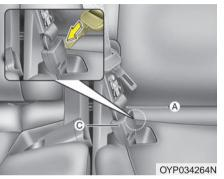
2. To retract the rear center seatbelt, insert the tongue plate or similar small rigid device into the web release hole (C). Pull up on the seat belt web (A) and allow the webbing to retract automatically.
