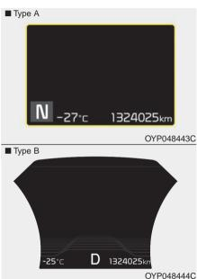
The current outside temperature is displayed in 1°C (1°F) increments. The temperature range is between -  $40^{\circ}$ C ~  $60^{\circ}$ C (- $40^{\circ}$ F ~  $140^{\circ}$ F).
