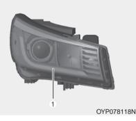
If the position lamp (LED) (1) does not operate, have the vehicle checked by an authorized Kia dealer.
