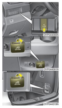
The AC inverter supplies 115V/100W electric power to operate electric accessories or equipments.
