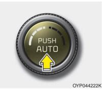
1. Press the AUTO button. The modes, fan speeds, air intake and air-conditioning will be controlled automatically by setting the temperature.
