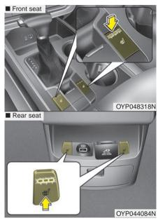
The seat warmer is provided to warm the front seats during cold weather. With the ignition switch in the ON position, push either of the switches to warm the driver's seat or the front passenger's seat. During mild weather or under conditions where the operation of the seat warmer is not needed, keep the switches in the "OFF" position.
