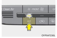
Press the A/C button to turn the air conditioning system on (indicator light will illuminate).
