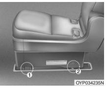
If the rear catches of the seat are locked into the rear anchors (2) while the front catches are not locked into the front anchors (1), do the following to release the rear catches from the rear anchors.
