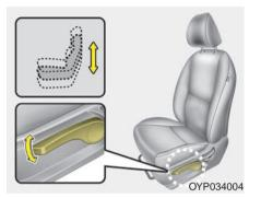
To change the height of the seat, push the lever upwards or downwards.
