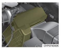
It must be replaced when necessary according to the Maintenance Schedule, and should not be washed.
