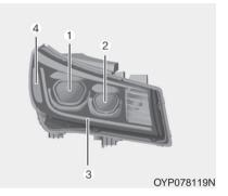
If the Low/High beam lamp (1), Low assist beam lamp (2), Position lamp (3) and Side marker (front) (4) does not operate, have the vehicle checked by an authorized Kia dealer.
