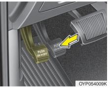
Check whether the stroke is within specification when the parking brake pedal is depressed with 66 lb, 294 N (30 kg) of force. Also, the parking brake alone should securely hold the vehicle on a fairly steep grade. If the stroke is more or less than specified, have the parking brake adjusted by an authorized Kia dealer.
