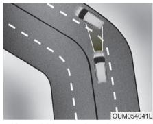
• Your vehicle speed can be reduced due to a vehicle in the adjacent lane. Adjust your speed by depressing the brake pedal or applying the accelerator pedal according to road and driving conditions ahead. Check to be sure that the road conditions permit safe operation of the smart cruise control. On inclines
