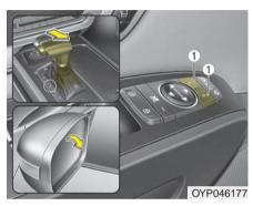
While the vehicle is moving rearward, the outside rearview mirror(s) will move downward to aid reverse parking. According to the position of the outside rearview mirror switch (1), the outside rearview mirror(s) will operate as follows:
