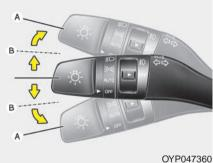
To signal a lane change, move the turn signal lever slightly and hold it in position (B). The lever will return to the OFF position when released.
