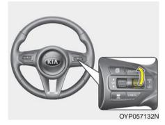
If any method other than the CRUISE button was used to cancel cruising speed and the system is still activated, the cruising speed will automatically resume when you move the lever up/down (to RES+ or SET-).
