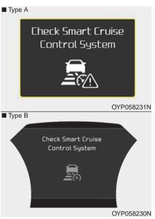
The message will appear when the vehicle to vehicle distance control system is not functioning normally.
