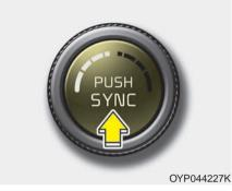
Adjusting the driver and passenger side temperature equally
