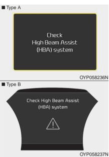
When the High Beam Assist is not working properly, the warning message will come on for a few second. After the message disappears, the master warning light ( ) will illuminate. Take your vehicle to an authorized Kia dealer and have the system checked.
