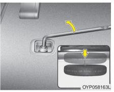
3. Use the tool to loosen the bolt enough to lower the spare tire.
