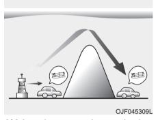
AM broadcasts can be received at greater distances than FM broadcasts. This is because AM radio waves are transmitted at low frequencies. These long distance,low frequency radio waves can follow the curvature of the earth rather than travelling straight. In addition, they curve around obstructions resulting in better signal coverage. FM radio station
