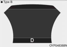
This indicator displays which automatic transmission shift lever is selected.
