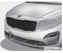
The sensor detects distance to the vehicle ahead.
