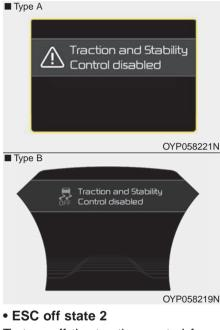
To turn off the traction control function and the brake control function of the ESC, press the ESC OFF button (ESC OFF  $\frac{1}{2}$ ) for more than 3 seconds. ESC OFF indicator light (ESC OFF  $\frac{1}{2}$ ) illuminates and ESC OFF warning chime will sound. At this state, the car stability control function does not operate.
