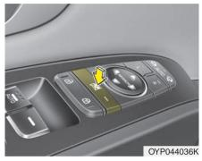
• The driver can disable the power window switches on a rear passenger door and the rear sunroof switch on a rear passenger room lamp by depressing the power window and rear sunroof lock switch on the driver's door to LOCK (pressed).
