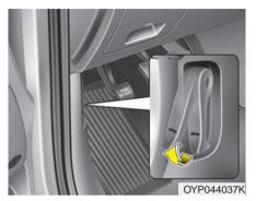
1. Pull the release lever to unlatch the hood. The hood should pop open slightly.
