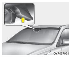
Auto defogging reduces the probability of fogging up the inside of the windshield by automatically sensing the moisture of inside the windshield.
