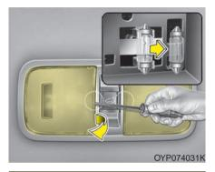
WARNING - Interior lights Prior to working on the Interior lamps, ensure that the "OFF" button is depressed to avoid burning your fingers or receiving an electric shock.
