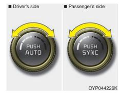
The temperature will increase to the maximum (HI) by turning the knob to the extreme right.
