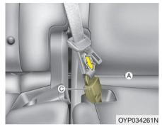
Insert the mini tongue (A) into the open end of the anchor connector (C) until an audible "click" is heard, indicating the latch is locked. Make sure the belt is not twisted.
