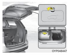
Your vehicle is equipped with an emergency liftgate safety release lever located on the bottom of the liftgate. When someone is inadvertently locked in the cargo area, the liftgate can be opened by pushing the release lever and pushing open the liftgate.
