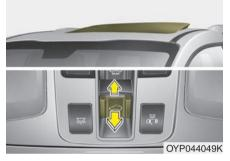
To tilt the sunroof, push the sunroof control lever upward until the sunroof moves to the desired position.
