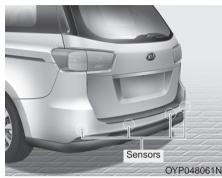
The parking distance warning-reverse assists the driver during backward movement of the vehicle by chiming if any object is sensed within a distance of 120 cm (47 in.) behind the vehicle.
