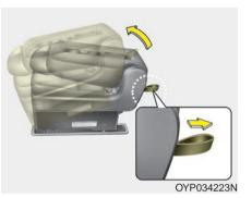
6. Pull the removal strap and lift the rear portion of the seat cushion.
