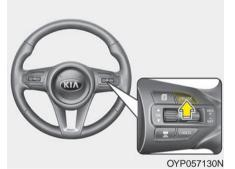
When the Smart Cruise Control System is not needed, press the [CRUISE] switch and deactivate the system.
