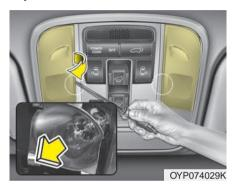
A WARNING - Interior lights Prior to working on the Interior lamps, ensure that the "OFF" button is depressed to avoid burning your fingers or receiving an electric shock.
