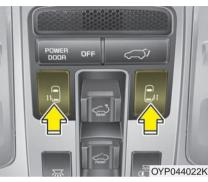
• Push the corresponding main control button on the overhead console to open or close the power sliding door.
