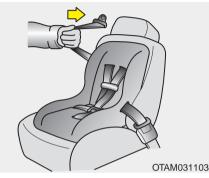
4. Slowly allow the shoulder portion of the seat belt to retract and listen for an audible "clicking" or "ratcheting" sound. This indicates that the retractor is in the "Automatic Locking" mode. If no distinct sound is heard, repeat steps 3 and 4.
