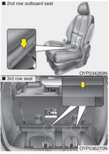
Child restraint hook holders are located on the back of the rear cushions.
