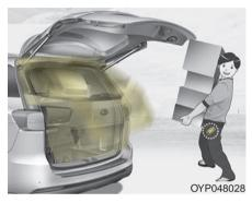
On a vehicle equipped with a smart key, the liftgate can be opened using the Smart liftgate system.
