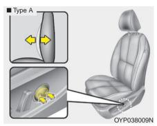
The lumbar support can be adjusted by pressing the lumbar support switch on the side of the driver's seat.
