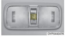
If your vehicle is equipped with a sunroof, you can slide or tilt your sunroof with the sunroof control lever located on the overhead console.
