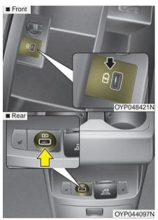
The USB charger is designed to recharge batteries of small size electrical devices using a USB cable. The electrical devices can be recharged when the Engine Start/Stop button is in ACC/ON/START position.
