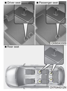
When using a floor mat on the front floor carpet, make sure it attaches to the floor mat anchor(s) in your vehicle. This keeps the floor mat from sliding forward. The following must be observed when installing ANY floor mat to the vehicle.
