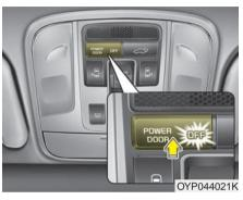
When the power door ON/OFF button is ON (not depressed), the power sliding door and power liftgate can be controlled with the sub control buttons on the center pillar trim or liftgate. Also, the doors can be opened and closed automatically by pulling the inside or outside door handles.
