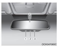
The electric rearview mirror automatically controls the glare from the headlights of the vehicles behind you in nighttime or low light driving conditions. The sensor (4) mounted in the mirror senses the light level around the vehicle, and automatically conrols the headlight glare from the vehicles behind you.
