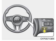
This function allows you to program the vehicle to maintain a predetermined distance to the vehicle ahead without depressing the accelerator pedal or brake pedal. The vehicle to vehicle distance will automatically activate when the smart cruise control system is on.
