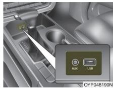
If your vehicle has an AUX and/or USB(universal serial bus) port, you can use an AUX port to connect audio devices and an USB and also an iPod<sup>®</sup>.
