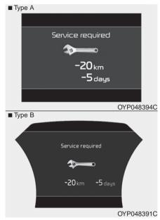
When Service Required is set, the remaining distance/period to drive before service is required appears on the LCD screen.
