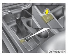
Active ECO helps improve fuel efficiency by controlling the engine and transmission. But fuel-efficiency can be affected by the driver's driving habits and road conditions.
