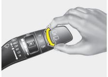
The rear window wiper is switched on automatically when the ignition is in OFF and the gear is shifted to R (Reverse) while the wiper is in motion.
