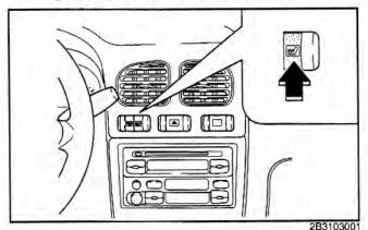
The front seats are electrically heated when the corresponding switch(shown above) is depressed and the vehicle ignition is ON. A thermostat regulates seat temperature when the switch is depressed. To deacti-
