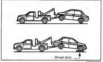
As a general rule, towed vehicles should be pulled with the driving wheels off the ground. If excessive damage or other conditions prevent towing the vehicle with the driving wheels off the ground, use wheel dollies.
