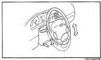
To tilt the wheel, hold the steering wheel and pull the lock release lever down. Move the steering wheel to a comfortable level, then push the lock release lever up to lock the steering wheel in place.
