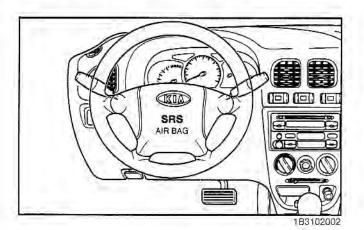
To indicate that your vehicle is equipped with air bags, the air bag covers on the steering wheel and on the dashboard are marked with "SRS AIR BAG."
