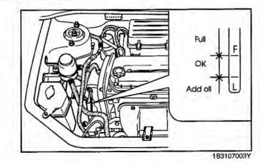
Use only the specified engine oil. (Refer to "Recommended Lubricants" in the Index.)
