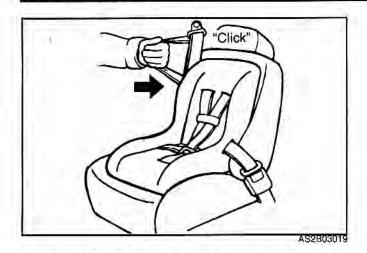
4. Slowly allow the belt to retract. Pull up on the shoulder webbing. A "clicking" or "ratcheting" sound will be heard as the belt retracts. This indicates the retractor is now in the automatic locking mode. Push down on the child restraint while you pull up on the belt in order to remove any slack in the belt.
