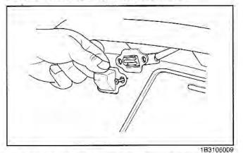
1. Using a Phillips screwdriver, remove the two (2) lens mounting screws and the lens.
