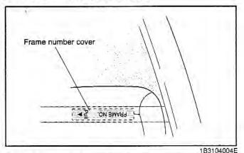
Frame Number is located under the front passenger seat. Please detach the plastic cover to see the frame number.
