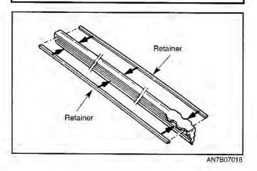
Carefully insert a new rubber blade and re-install the blade assembly in the reverse order of removal.
