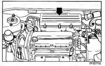
2. Wipe the inside of the air cleaner housing with a clean, damp cloth.
