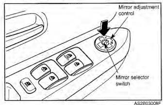
This switch controls the adjustments for both right and left outside mirrors. To adjust the position of either mirror:
