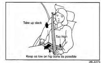
4. Position the lap portion of the belt across your lap as LOW ON THE HIPS as possible to reduce the risk of sliding under it during an accident. Adjust the belt to a SNUG FIT by pulling up on the shoulder portion of the safety belt. The belt retractor is designed to take up excess webbing automatically and to maintain tension on the belt. This is for your safety. Do not put excess slack into the safety belt.
