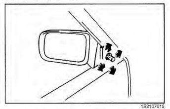
To adjust an outside mirror, move the control lever which is located at the forward inside area of the window frame. Outside Rearview Mirror Electric Remote Control (If Equipped)
