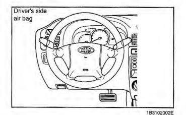
To indicate that your vehicle is equipped with air bags, the air bag covers on the steering wheel and on the dashboard are marked with "SRS AIR BAG."
