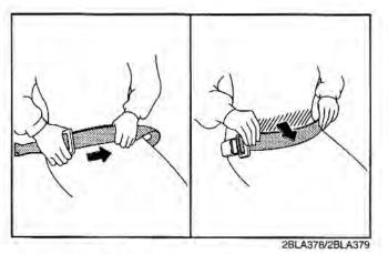
5. Make sure that the belt is placed as LOW ON THE HIPS as possible.
