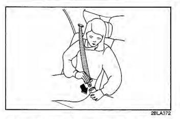
Insert the tongue plate into the open end of the buckle until an audible "click" is heard, indicating the belt is locked.
