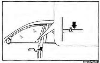
To lock any door without the key, push the inside door lock button down and close the door.
