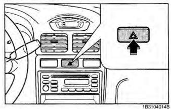
The hazard warning flasher causes the rear tail lights and front turn signal lights to flash on and off, which serves as a warning to other drivers to exercise caution when approaching or passing your vehicle.
