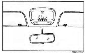
The lights are switched ON or OFF by pressing the correpoiding switches.
