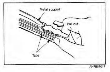
3. Remove the metal retainers from the rubber blade and install them in the new rubber blade.
