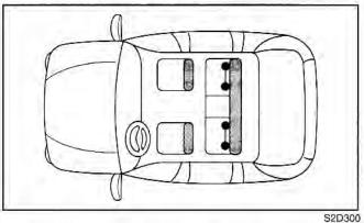
The lower anchors are located between rear seat cushion and seatback.
