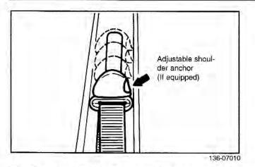
5. Adjust the shoulder anchor position to your size. To raise the anchor position, pull the knob and push the anchor up. To lower the anchor position, pull the knob and slide the anchor down. After adjustment, make sure the anchor is locked in position.
