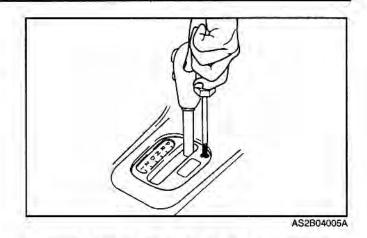
Insert a screwdriver (cross or flat blade) into the access hole, then depress the screwdriver.
