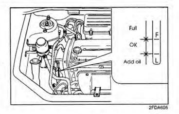
Use only the specified engine oil. (Refer to "Recommended Lubricants" later in this section.)
