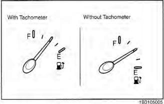
The fuel gauge indicates the approximate amount of fuel remaining in the fuel tank.
