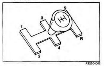
Press the clutch pedal down fully while shifting, then release it slowly.
