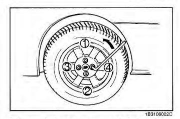
Loosen the four lug nuts counterclockwise one turn each, but do not remove any nut until the tire has been raised off the ground.
