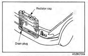
3. With the drain plug loose, flush the system with running water.
