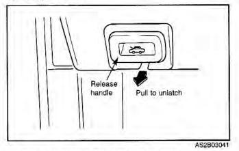
1. Inside the vehicle, pull the hood release handle located at the bottom left corner of the instrument panel.
