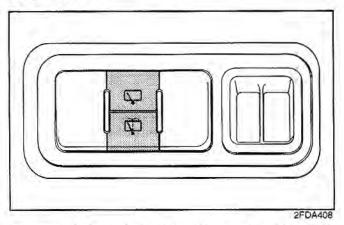
The rear window wiper and washer can be activated by depressing the corresponding switch.
