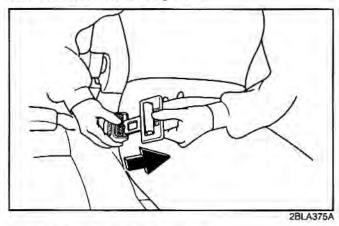
Press the release button on buckle.
