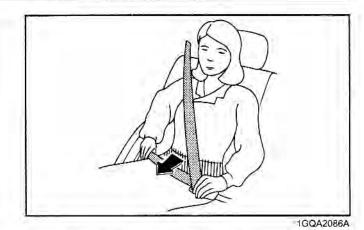
4. Position the lap portion of the belt across your lap as LOW ON THE HIPS as possible to reduce the risk of sliding under it during an accident. Adjust the belt to a SNUG FIT by pulling up on the shoulder portion of the safety belt. The belt retractor applies tension to the belt in order to take up excess webbing automatically and to maintain tension on the belt. For maximum safety, do not put any excess slack into the safety belt.
