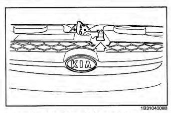
2. Go to the front of the vehicle, raise the hood until the secondary latch catches, then lift the secondary latch up (located under the hood at the center of the vehicle).
