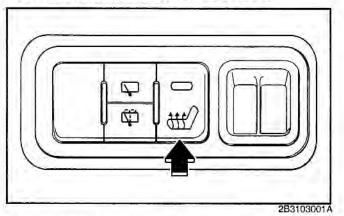
The driver's seat is electrically heated when the corresponding switch(shown above) is depressed and the vehicle ignition is ON. A thermostat regulates seat temperature when the switch is depressed. To deactivate the driver's seat heating system, depress the switch again.
