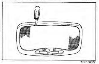
Using a flat-blade screwdriver, gently pry the lens from the dome light housing.
