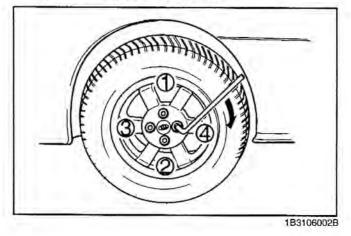
Once the lug nuts have been tightened, lower the vehicle fully to the ground and continue to tighten the lug nuts until they are completely secured.
