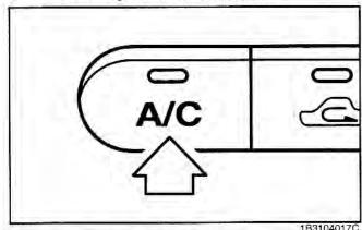
Depress the switch to turn the air conditioning system on. An indicator light in the switch will illuminate when the fan switch is ON indicating air conditioning system operation. Depress the switch again to turn the air conditioning system OFF.
