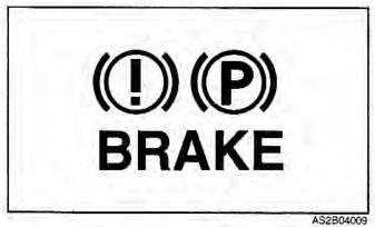
Check the brake warning light each time you start the engine. The light is located in the instrument panel. This warning light will be illuminated when the ignition switch in ON or START and the parking brake is set.
