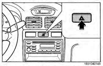
The hazard warning flasher serves as a warning to other drivers to exercise extreme caution when approaching, overtaking, or passing your vehicle. It should be used whenever emergency repairs are being made or when the vehicle is stopped near the edge of a roadway. Depress the flasher switch with the ignition switch in any position. The flasher switch is located in the center console. All turn signal lights will flash simultaneously.
