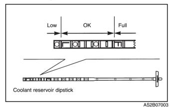
If the coolant level is low, add enough specified coolant to provide protection against freezing and corrosion and to bring the level to F in the coolant reservoir. Do not overfill. If frequent additions are required, see an Authorized Kia Dealer for a cooling system inspection.
