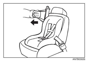
3. Grasp the shoulder portion of the belt and pull downward until the entire belt is extracted. When the belt is fully extracted, the retractor changes to the automatic locking mode (child restraint mode).
