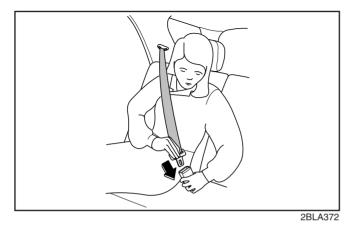
3. Insert the tongue plate into the open end of the buckle until an audible "click" is heard, indicating the belt is locked.
