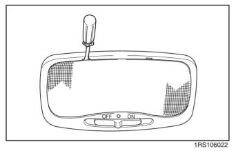
1. Using a flat-blade screwdriver, gently pry the lens from the dome light housing.
