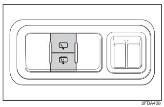
The rear window wiper and washer can be activated by depressing the corresponding switch.
