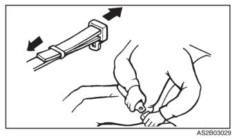
4. Grasp the free portion of the belt webbing and pull until the belt is snug over the hips and as low on the abdomen as possible.
