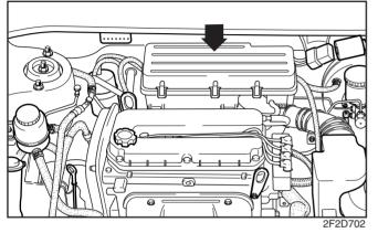
2. Wipe the inside of the air cleaner housing with a clean, damp cloth.
