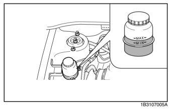
Before adding power steering fluid, thoroughly clean the area around the reservoir cap to prevent power steering fluid contamination.
