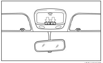
1BC102003D The lights are switched ON or OFF by pressing the correpoiding switches.
