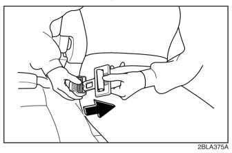
Press the release button on buckle.
