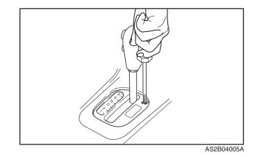
2. Insert a screwdriver (cross or flat blade) into the access hole, then depress the screwdriver.
