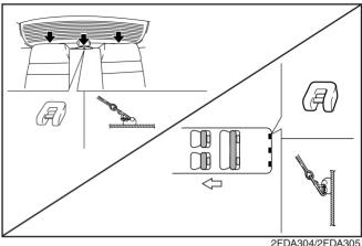
Your vehicle is equipped with an anchor for securing the tether strap of a child restraint system (child seat). The child restraint anchor fittings are installed on the shelf behind the rear seat or in the trunk on the inboard side of the rear bumper in the 5-door hatchback.
