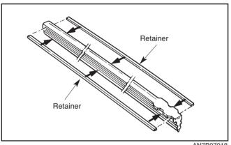
4. Carefully insert a new rubber blade and re-install the blade assembly in the reverse order of removal.
