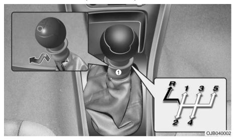
The shift lever can be moved without pulling the ring (1).
