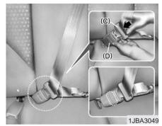
Pull the tongue plate (C) and insert the tongue plate (C) into the open end of the buckle (D) until an audible "click" is heard, indicating the latch is locked.
