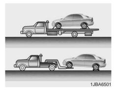
If emergency towing is necessary, we recommend having it done by an authorized Kia dealer or a commercial tow-truck service. Proper lifting and towing procedures are necessary to prevent damage to the vehicle. The use of wheel dollies or flatbed equipment is recommended.
