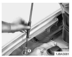
3. Lift the hood and hold it open with the support rod by inserting the free end of the rod into the slot (1).
