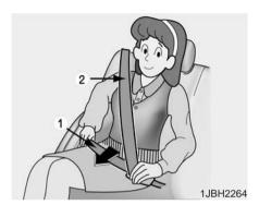
4. Position the lap portion (1) of the belt across your lap as LOW ON THE HIPS as possible to reduce the risk of sliding under it during an accident. Adjust the belt to a SNUG FIT by pulling up on the shoulder portion (2) of the safety belt. The belt retractor is designed to take up excess webbing automatically and to maintain tension on the belt. For your safety, do not put any excess slack into the safety belt at any location.
