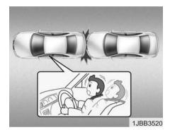
Frontal air bags are not designed to inflate in rear collisions, because occupants are moved backward by the force of the impact. In this case, the air bags do not provide protection.
