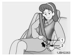
Insert the tongue plate (1) into the open end of the buckle (2) until an audible "click" is heard, indicating the belt is locked in the buckle.
