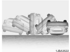
Air bags may not inflate in rollover accidents because air bag deployment would not provide proper protection to the occupants.
