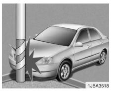
Air bags may not inflate if the vehicle collides with objects such as utility poles or trees, where the point of impact is concentrated to one area and the full force of the impact is not transmitted to the sensors.
