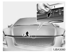
Go to the front of the vehicle, raise the hood slightly, pull the secondary latch (1) inside of the hood center and lift (2) the hood.
