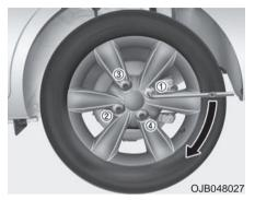
12. Once the wheel lug nuts have been tightened, lower the vehicle fully to the ground and continue to tighten the lug nuts until they are fully secured. Tighten the wheel lug nuts firmly in a "X" pattern.
