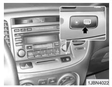
The defroster heats the window to remove frost, fog and thin ice from the interior and exterior of the rear window, while engine is running.
