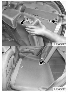
5. Move the rear lap/shoulder belt to the outside (2) so that they don't interfere with the seatback when lowering (3).
