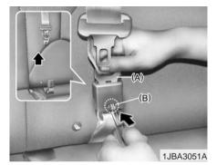
To retract the rear center seatbelt, insert the key or similar small rigid device into the web release button (B) on the anchor connector. Pull up on the seat belt web (A) and allow the webbing to retract automatically. (4Door, if equipped)
