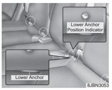
Child restraint symbols are located on the left and right rear seat backs to indicate the position of the lower anchors for child restraints
