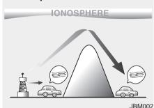
This is because AM radio waves are transmitted at low frequencies. These long, low frequency radio waves can follow the curvature of the earth rather than travelling straight out into the atmosphere. In addition, they curve around obstructions so that they can provide better signal coverage.
