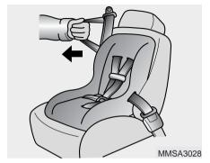
Pull the shoulder portion of the safety belt all the way out. When the shoulder portion of the safety belt is fully extended, it will shift the retractor to the "Auto Lock" (child restraint) mode.
