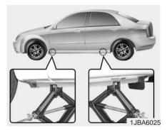
8. Place the jack at the front or rear jacking position closest to the tire you are changing. Place the jack at the designated locations under the frame. The jacking positions are plates welded to the frame with two tabs and a raised dot to index with the jack.
