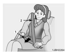
4. Position the lap portion (1) of the belt across your lap as LOW ON THE HIPS as possible to reduce the risk of sliding under it during an accident. Adjust the belt to a SNUG FIT by pulling up on the shoulder portion (2) of the safety belt. The belt retractor is designed to take up excess webbing automatically and to maintain tension on the belt. For your safety do not put any excess slack into the safety belt.
