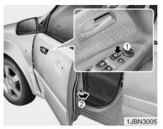
To lock a door without the key, push down on the front portion of the inside door lock switch (1, if equipped) to the "LOCK" position and close the door (2).
