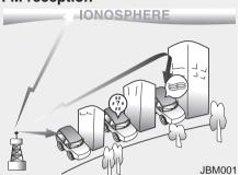
AM and FM radio signals are broadcast from transmitter towers located around your city. They are intercepted by the radio antenna on your car. This signal is then received by the radio and sent to your car speakers.
