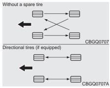
Disc brake pads should be inspected for wear whenever tires are rotated. Rotate radial tires that have an asymmetric tread pattern only from front to rear and not from right to left.
