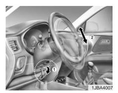
To change the steering wheel angle, pull down (1) the lock release lever, adjust the steering wheel to the desired angle (2), then pull up the lock-release lever to lock the steering wheel in place.
