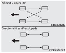
Disc brake pads should be inspected for wear whenever tires are rotated. Rotate radial tires that have an asymmetric tread pattern only from front to rear and not from right to left.
