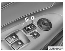
With central door lock switch (if equipped)
