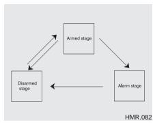
Theft alarm system will not operate when the ignition key is in the ignition switch.
