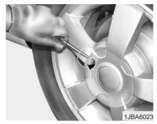
Wrap a piece of cloth around the tip of the screwdriver to avoid scratching.
