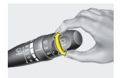
Rear window wiper and washer switch (if equipped)
