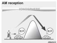
This is because AM radio waves are transmitted at low frequencies. These long, low frequency radio waves can follow the curvature of the earth rather than travelling straight out into the atmosphere. In addition, they curve around obstructions so that they can provide better signal coverage.
