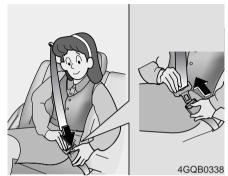
**To unfasten:**Press the release button on the buckle and allow the belt to slowly retract.
