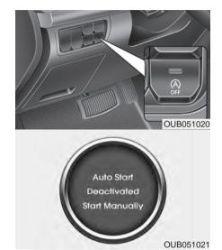
If you open the engine hood in auto stop mode, the light on the ISG OFF button will illuminate and ISG system is deactivated. If your vehicle is equipped with the type B cluster, the notice will illuminate on the LCD display.
