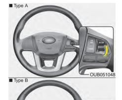
3. Move the lever (1) down (to SET-), and release it at the desired speed. The SET indicator light in the instrument cluster will illuminate. Release the accelerator at the same time. The desired speed will automatically be maintained.
