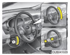
To change the steering wheel angle, pull down the lock release lever (1), adjust the steering wheel to the desired angle (2) and height (if equipped) (3), then pull up the lock-release lever to lock the steering wheel in place. Be sure to adjust the steering wheel to the desired position before driving.
