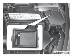
Engine compartment fuse panel
