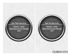
If you would like to reset or inactivate the maintenance system press the RESET button for more than 1 second. The display will change to "Engine Oil Service Message" mode.
