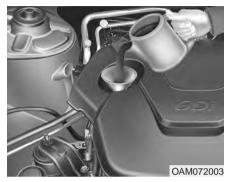
If it is near or at L, add enough oil to bring the level to F. **Do not overfill.**
