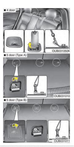
Securing a child restraint seat with tether anchorage system
