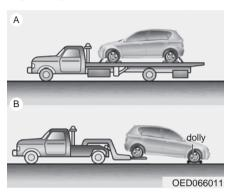
When being towed by a commercial tow truck and wheel dollies are not used, the front of the vehicle should always be lifted, not the rear.
