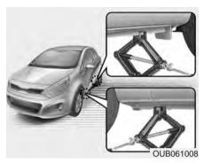
7. Place the jack at the front or rear jacking position closest to the tire you are changing. Place the jack at the designated locations under the frame. The jacking positions are plates welded to the frame with two tabs and a raised dot to index with the jack.
