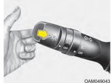
To flash the headlights, pull the lever towards you. It will return to the normal (low-beam) position when released. The headlight switch does not need to be on to use this flashing feature.
