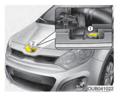
Go to the front of the vehicle, raise the hood slightly, push the secondary latch (1) inside of the hood center and lift the hood (2).
