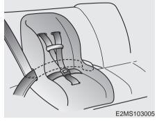
Lacing a passenger seat belt into the auto lock mode
