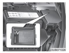
Engine compartment fuse panel
