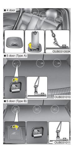
Securing a child restraint seat with tether anchorage system
