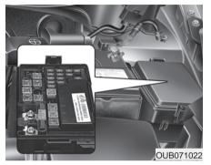
Engine compartment panel fuse replacement
