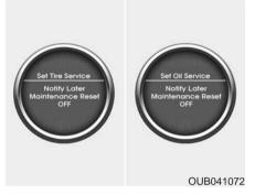
2. If you would like to reset or inactivate the maintenance system press the RESET button for more than 1 second. The display will change to "Engine Oil Service Message" mode.
