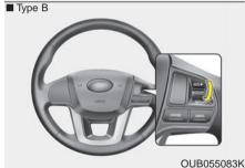
Move the lever (1) down (to SET-), and release it at the desired speed. The SET indicator light in the instrument cluster will illuminate. Release the accelerator at the same time. The desired speed will automatically be maintained.
