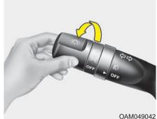
Headlight position ( [0]) When the light switch is in the headlight position (2nd position) the head, tail, position, license and instrument panel lights will turn ON.
