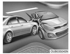
Front air bags may not inflate in side impact collisions, because occupants move to the direction of the collision, and thus in side impacts, front air bag deployment would not provide additional occupant protection.
