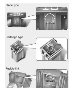
A vehicle's electrical system is protected from electrical overload damage by fuses.
