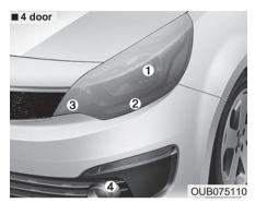
Headlight, position light, turn signal light, side marker light and front fog light bulb replacement
