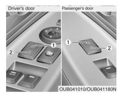
With central door lock switch (if equipped)
