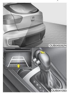
The Rear-Camera Display will activate when the back-up light is ON with the ignition switch ON and the shift lever in the R (Reverse) position.
