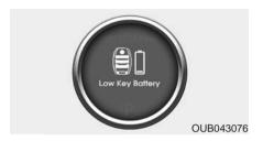
If the engine start/stop button changes to the OFF position when the smart key in the vehicle discharges, the warning illuminates on the LCD display for about 10 seconds. Also, the warning chime sounds once.
