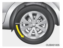
Loosen the wheel lug nuts counterclockwise one turn each, but do not remove any nut until the tire has been raised off the ground.
