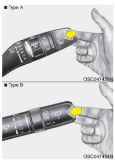
In the OFF position, pull the lever gently toward you to spray washer fluid on the windshield and to run the wipers 1-3 cycles.
