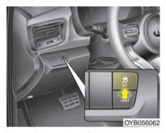
The Electronic Stability control (ESC) system is designed to stabilize the vehicle during cornering maneuvers. ESC checks where you are steering and where the vehicle is actually going. ESC applies the brakes on individual wheels and intervenes with the engine management system to stabilize the vehicle.
