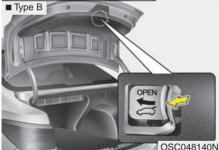
Your vehicle is equipped with an emergency trunk release lever located inside the trunk. If someone is inadvertently locked in the trunk, moving the handle in the direction of the arrow will release the trunk latch mechanism and open the trunk.
