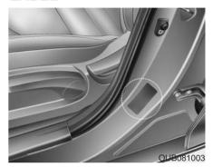
vehicle certification label attatched on the driver's side center pillar gives the vehicle identification number (VIN).
