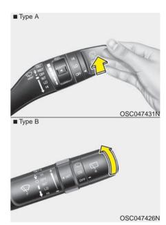
Push the lever away from you or turn the wiper lever switch upwards fully to spray rear washer fluid and to run the rear wipers 1~3 cycle. The spray and wiper operation will continue until you release the lever.
