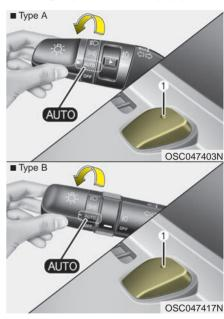
When the light switch is in the AUTO light position, the taillights and headlights will turn ON or OFF automatically depending on the amount of light outside the vehicle.
