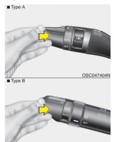
To turn on the high beam headlights, push the lever away from you. Pull it back for normal (low beam) position.
