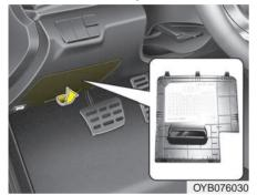
Inside the fuse/relay panel covers, you can find the fuse/relay label describing fuse/relay name and capacity.
