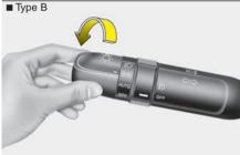
When the light switch is in the parking light position (3rd position), the tail, position, license and instrument panel lights will turn ON.
