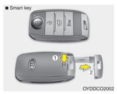
To remove the mechanical key, press and hold the release button and remove the mechanical key.
