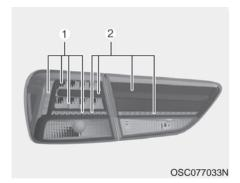
If the stop and tail lamp (LED) (1,2) does not operate, have the vehicle checked by an authorized Kia dealer. The LED lamps cannot be replaced as a single component because it is part of an integrated unit. The LED lamps have to be replaced with the unit.
