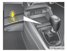
With the ignition switch in the ON position, pressing the heated steering wheel button warms the steering wheel. The indicator on the button will illuminate
