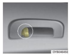
The clothes hanger is located on the roof of the rear seats
