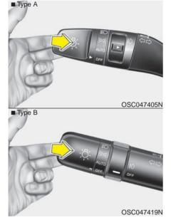
To flash the headlights, pull the lever towards you. It will return to the normal (low-beam) position when released. The headlight switch does not need to be on to use this flashing feature.
