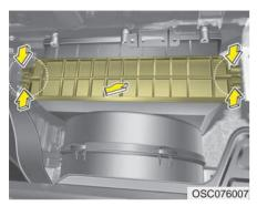
3. Remove the climate control air filter cover while pressing the lock on the both sides of the cover.
