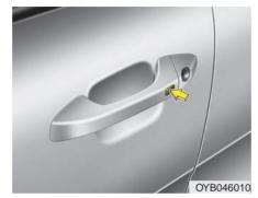
Pressing the button of the front outside door handles with all doors closed and any door unlocked, locks all the doors (and hood, trunk/tailgate).
