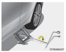
8. Insert the jack handle into the jack and turn it clockwise, raising the vehicle until the tire just clears the ground. This measurement is approximately 30 mm (1 in). Before removing the wheel lug nuts, make sure the vehicle is stable and that there is no chance for movement or slippage.
