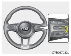
Move the lever down (to SET-), and release it at the desired speed. The SET indicator light in the instrument cluster will illuminate. Release the accelerator pedal at the same time. The desired speed will automatically be maintained.
