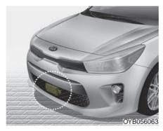
The sensor is to maintain a certain distance from the vehicle in front. However, a sensor covered or dirty with foreign substances, such as snow and rain, adversely affects the sensing performance. It may even temporarily cancel the FCA. Always keep the sensor clean.
