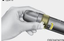
Fog lights are used to provide improved visibility when visibility is poor due to fog, rain or snow, etc. The fog lights will turn on when the fog light switch (1) is turned to the on position after the headlights are turned on.
