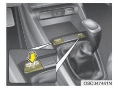
The seat warmer is provided to warm the front seats during cold weather. With the ignition switch in the ON position, push either of the switches to warm the driver's seat or the front passenger's seat.
