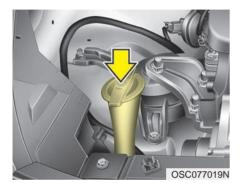
The reservoir is translucent so that you can check the level with a quick visual inspection.
