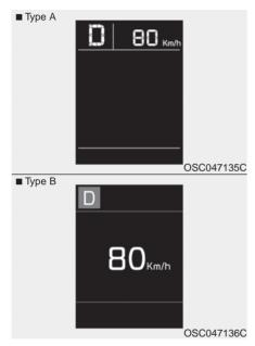
This mode displays the current speed of the vehicle.
