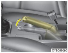
To engage the parking brake, first apply the foot brake and then without pressing the release button in, pull the parking brake lever up as far as possible. In addition it is recommended that when parking the vehicle on a gradient, the shift lever should be positioned in the appropriate low gear for Manual Transmission vehicles or in the P (Park) position for Automatic Transmission vehicles.
