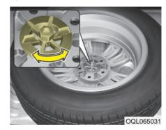
Turn the tire hold-down wing bolt counterclockwise to remove the spare tire.
