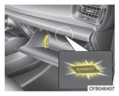
The glove box lamp comes on when the glove box is opened. To prevent unnecessary charging system drain, close the glove box securely after use.
