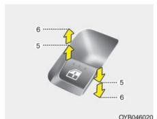
Pressing or pulling up the power window switch momentarily to the second detent position (6) completely lowers or lifts the window even when the switch is released. To stop the window at the desired position while the window is in operation, pull up or press and release the switch to the opposite direction of the movement.
