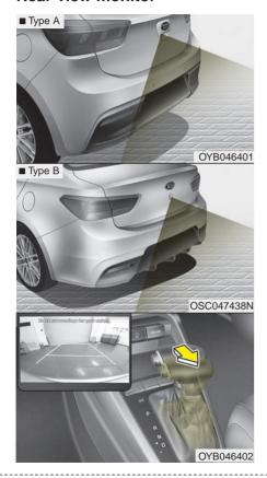
The rear view monitor will activate with the ignition switch on and the shift lever in the R (Reverse) position.
