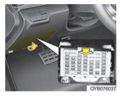
Your vehicle is equipped with the memory fuse to prevent battery discharge if your vehicle is parked without being operated for prolonged periods. Use the following procedures before parking the vehicle for prolonged periods.
