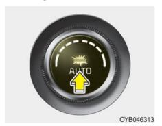
1. Push the AUTO button. The modes. fan speeds, air intake and air-conditioning will be controlled automatically by temperature setting.
