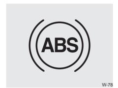
The ABS warning light will stay on for approximately 3 seconds after the ignition switch is ON. During that time, the ABS will go through self-diagnosis and the light will go off if everything is normal. If the light stays on, you may have a problem with your ABS but your regular brakes will work normally. Contact an authorized Kia dealer as soon as possible.
