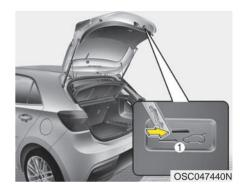
Your vehicle is equipped with the emergency tailgate safety release lever located on the bottom of the tailgate. If someone is inadvertently locked in the luggage compartment. The tailgate can be opened by doing as follows:
