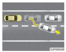
When driving in stop-and-go traffic, and a stopped vehicle in front of you merges out of the lane, the FCA system may not immediately detect the new vehicle that is now in front of you. In this case, you must maintain a safe braking distance, and if necessary, depress the brake pedal to reduce your driving speed in order to maintain a safe distance.
