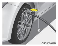
5. Unscrew the valve cap from the valve of the defective wheel and screw filling hose (3) of the sealant bottle onto the valve.
