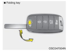
To unfold the key, press the release button then the key will unfold automatically.
