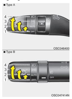
The light switch has a Headlight and a Parking light position.
