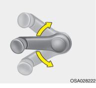
To raise or lower the window, turn the window regulator handle clockwise or counterclockwise.
