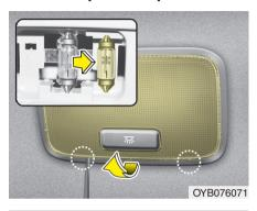
A WARNING - Interior lamps Prior to working on the Interior lamps, ensure that the "OFF" button is depressed to avoid burning your fingers or receiving an electric shock.
