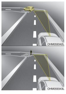
Forward Collision- Avoidance Assist may be limited when driving on a curved road.
