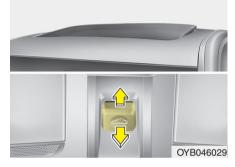
To tilt open the sunroof, push the sunroof control lever upward until the sunroof moves to the desired position.
