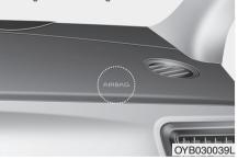
Your vehicle is equipped with an Advanced Supplemental Restraint (Air Bag) System and lap/shoulder belts at both the driver and passenger seating position. The indications of the system's presence are the letters "AIR BAG" embossed on the air bag pad cover in the steering wheel and the passenger's side front panel pad above the glove box.
