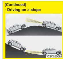
Blind-Spot Safety system may not operate properly when driving on a slope. The function may not detect the vehicle in the next lane or may incorrectly detect the ground or structure. Always pay attention to road
