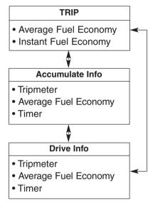
To change the trip mode, scroll the MOVE scroll switch  $(\wedge/\vee)$  in the trip computer mode.
