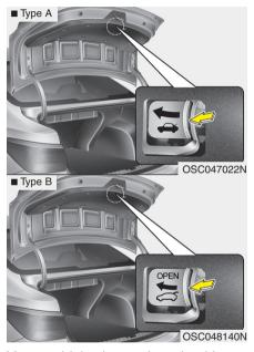
Your vehicle is equipped with an emergency trunk release lever located inside the trunk. If someone is inadvertently locked in the trunk, moving the handle in the direction of the arrow will release the trunk latch mechanism and open the trunk.
