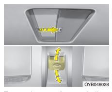
To open the sunroof automatically: Pull the sunroof control lever backward to the second detent position and then release it. The sunroof will slide all the way open.
