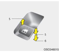
Pressing the power window switch momentarily to the second detent position (6) completely lowers the driver's window even when the switch is released. To stop the window at the desired position while the window is in operation, briefly pull up the switch to the opposite direction of the window movement. Auto up/down window (if equipped) (Driver's window)
