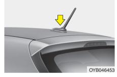
The micro pole antenna receives data transmitted from base stations and satellites (e.g. AM/FM, SXM, GPS, LTE) and also transmits to base stations (e.g. LTE). The antenna pole is removable type.
