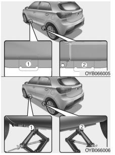
7. Place the jack at the front (1) or rear (2) jacking position closest to the tire you are changing. Place the jack at the designated locations under the frame. The jacking positions are plates welded to the frame with two tabs and a raised dot to index with the jack. SC PE CAN (ENG) 6.qxp 10/23/2020 8:17 PM Page 31
