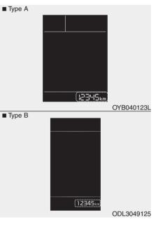
The odometer indicates the total distance the vehicle has been driven.
