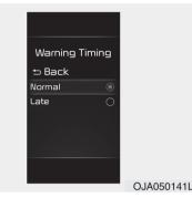
The driver can select the initial warning activation time in the User Settings in the LCD display by selecting "User Settings  $\rightarrow$  Driver Assistance  $\rightarrow$  Warning Timing". When the vehicle is first delivered, warning timing is set to 'Normal'. If you change the warning timing, the warning time of other Driver Assistance functions may change. Make sure to check the warning timing before changing it.
