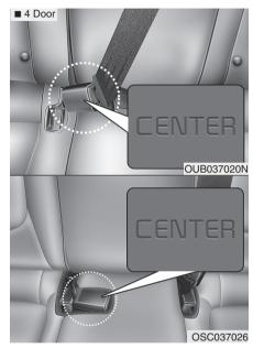
When using the rear center seat belt, the buckle with the "CENTER" mark must be used.
