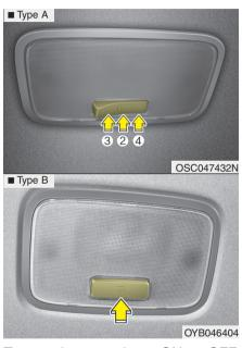
To turn the room lamp ON or OFF, push the switch.
