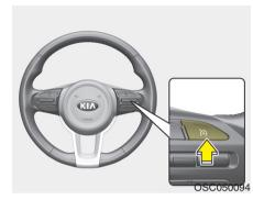
Press the Driving Assist (\*) button to turn Cruise Control off. The Cruise (\*) CRUISE) indicator will go off. Always press the Driving Assist but-
