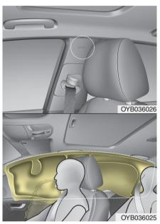
\* The actual air bags in the vehicle may differ from the illustration. Curtain air bags are located along both sides of the roof rails above the front and rear doors.
