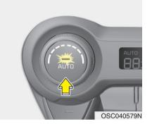
1. Push the AUTO button. The modes, fan speeds, air intake and air-conditioning will be controlled automatically by temperature setting.
