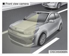
The front view camera is used as a detecting sensor to detect driving patterns and front vehicle departure while vehicle is being driven.
