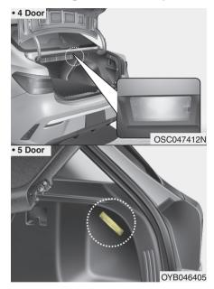
The trunk/liftgate room lamp comes on when the trunk/liftgate is opened.
