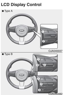
The LCD Display modes can be changed by using the control buttons on the steering wheel.
