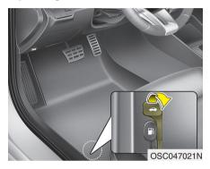
• To open the trunk from inside the vehicle, pull the trunk lid release lever.
