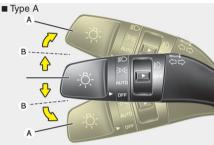
They will self-cancel after a turn is completed. If the indicator continues to flash after a turn, manually return the lever to the OFF position.
