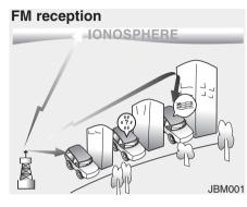
This can be due to many factors, such as the distance from the radio station, closeness of other strong radio stations or the presence of buildings, bridges or other large obstructions in the area.
