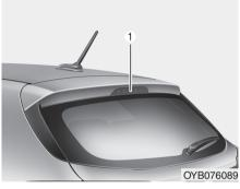
If the high mounted stop lamp (1) does not operate, have the vehicle checked by an authorized Kia dealer.
