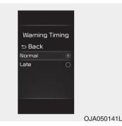
The driver can select the initial warning activation time in the User Settings in the instrument cluster LCD display.
