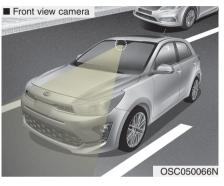
The front view camera is used as a detecting sensor to detect lane markings.
