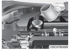
Check if the oil level is between the F-L line and refill it if the oil level is near the L line.
