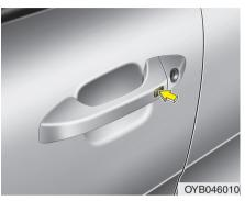
Pressing the button of the front outside door handles with all doors (and trunk, liftgate) closed and any door unlocked, locks all the doors (and trunk, liftgate).
