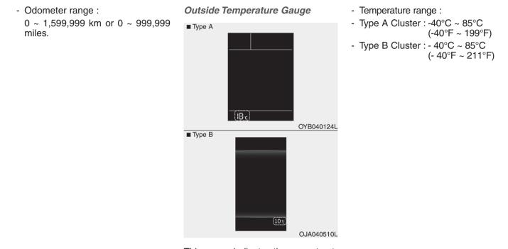
This gauge indicates the current outside air temperatures by 1°C (1°F).
