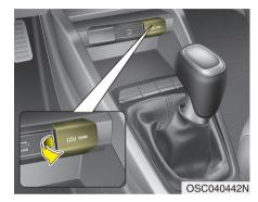
The power outlet is designed to provide power for mobile telephones or other devices designed to operate with vehicle electrical systems. The devices should draw less than 12V, 15A with the engine running.
