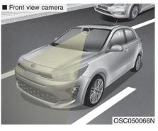
The front view camera is used as a detecting sensor to detect lane markings and front vehicles.
