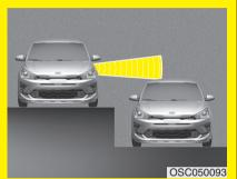
Blind-Spot Safety system may not operate properly when driving where the heights of the lanes are different. The function may not detect the vehicle on a road with different lane heights (underpass joining section, grade separated intersections, etc.).
