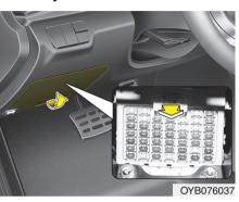
Your vehicle is equipped with the memory fuse to prevent battery discharge if your vehicle is parked without being operated for prolonged periods. Use the following procedures before parking the vehicle for prolonged periods.
