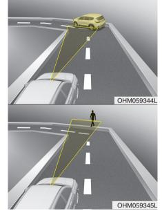
Forward Collision-Avoidance Assist may recognize a vehicle or pedestrian in the next lane or outside the lane when driving on a curved road.
