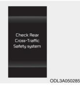
When Rear Cross-Traffic Safety is not working properly, the 'Check Rear Cross-Traffic Safety system' warning message will appear on the cluster, and the function will turn off automatically, or the function will be limited. In this case, have your vehicle inspected by an authorized Kia dealer.
