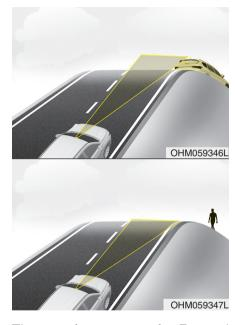
The performance of Forward Collision-Avoidance Assist may be decreased while driving upward or downward on a slope.
