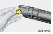
To turn on the high beam headlights, push the lever away from you. Pull it back for normal (low beam) position.
