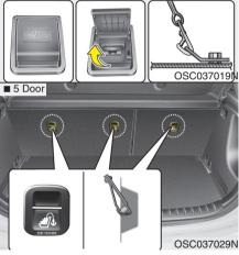
Child restraint hook holders are located on the package tray (4 Door) or the floor behind the rear seat (5 Door).
