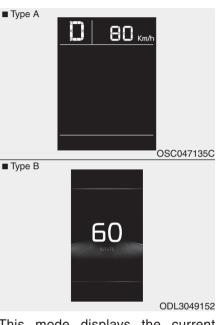
This mode displays the current speed of the vehicle.
