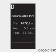
Displays accumulated information starting from a mileage/fuel efficiency/time default point.
