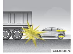
Just before impact, drivers often brake heavily. Such heavy braking lowers the front portion of the vehicle causing it to "ride" under a vehicle with a higher ground clearance. Air bags may not inflate in this "under-ride" situation because deceleration forces that are detected by sensors may be significantly replaced by such "under-ride" collisions.
