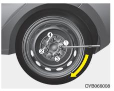
Then position the wrench as shown in the drawing and tighten the wheel nuts. Be sure the socket is seated completely over the nut. Do not stand on the wrench handle or use an extension pipe over the wrench handle.
