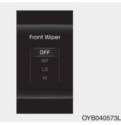
This indicator displays which wiper speed is selected using the wiper control.
