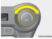
The fan speed can be set to the desired speed by operating the fan speed control knob.
