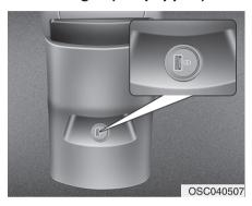
The USB charger is designed to recharge batteries of small size electrical devices using a USB cable. The electrical devices can be recharged when the ignition switch is in ACC/ON/START position.
