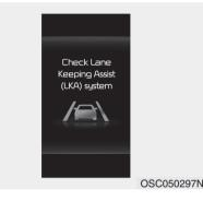
When Lane Keeping Assist is not working properly, the 'Check Lane Keeping Assist (LKA) system', warning message will appear and the yellow (/ ) indicator light will illuminate on the cluster. In this case, have your vehicle inspected by an authorized Kia dealer.
