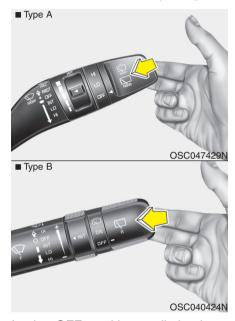
In the OFF position, pull the lever gently toward you to spray washer fluid on the windshield and to run the wipers 1-3 cycles.
