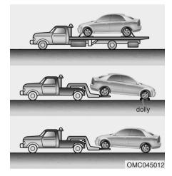
If emergency towing is necessary, we recommend having it done by an authorized Kia dealer or a commercial tow-truck service. Proper lifting and towing procedures are necessary to prevent damage to the vehicle. The use of wheel dollies or flatbed is recommended. It is acceptable to tow the vehicle with the rear wheels on the ground (without dollies) and the front wheels off the ground.
