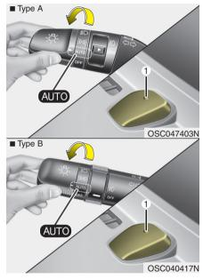
When the light switch is in the AUTO light position, the taillights and head-lights will turn ON or OFF automatically depending on the amount of light outside the vehicle.
