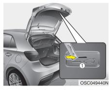
Your vehicle is equipped with the emergency liftgate safety release lever located on the bottom of the liftgate. If someone is inadvertently locked in the luggage compartment. The liftgate can be opened by doing as follows:
