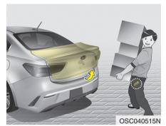
On a vehicle equipped with a smart key, the trunk can be opened with no-touch activation using the Smart Trunk Release system. How to use the Smart Trunk Release
