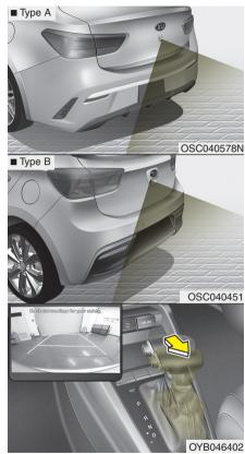
Rear View Monitor will show the area behind the vehicle to assist you when parking or backing up.
