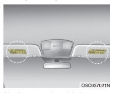
Air bag warning labels, some required by the Canada Motor Vehicle Safety Standards (CMVSS), are attached to the sun visor to alert the driver and passengers of potential risks of the air bag system.
