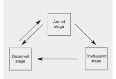
This system is designed to provide protection from unauthorized entry into the vehicle. This system is operated in three stages: the first is the "Armed" stage, the second is the "Theft-alarm" stage, and the third is the "Disarmed" stage. If triggered, the system provides an audible alarm with blinking of the hazard warning lights.
