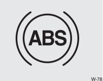
The ABS warning light will stay on for approximately 3 seconds after the ignition switch or ENGINE START/STOP button is ON. During that time, the ABS will go through self-diagnosis and the light will go off if everything is normal. If the light stays on, you may have a problem with your ABS but your regular brakes will work normally. Contact an authorized Kia dealer as soon as possible.
