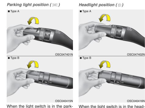
When the light switch is in the parking light position (3rd position), the tail, position, license and instrument panel lights will turn ON. When the light switch is in the headlight position (4th position) the head, tail, position, license and instrument panel lights will turn ON.
