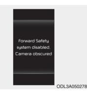
In this case, a warning message will appear to notify the driver. Remove the foreign substances to allow FCA to function normally.
