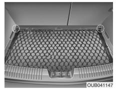
To keep items from shifting in the cargo area, you can use the 4 holders located in the cargo area to attach the luggage net (if equipped).
