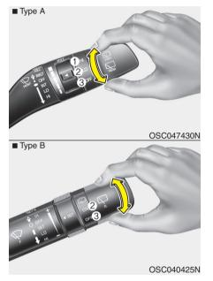
The rear window wiper and washer switch is located at the end of the wiper and washer switch lever. Turn the switch to operate the rear wiper and washer.
