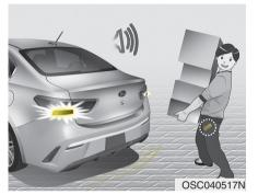
3. Automatic opening The hazard warning lights will blink and chime will sound 2 times and then the trunk will open.
