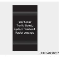
When the rear bumper around the rear-side radar or sensor is covered with foreign matters, such as snow or rain, or installing a trailer or carrier, it can reduce the detecting performance and temporarily limit or disable Rear Cross-Traffic Safety.
