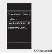
If 'Leading Vehicle Departure Alert's is selected, the function will inform the driver when the front vehicle departs from a stop.
