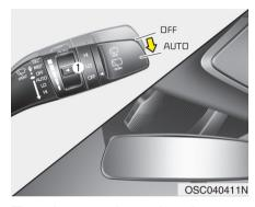
The rain sensor located on the upper end of the windshield glass senses the amount of rainfall and controls the wiping cycle for the proper interval. The more it rains, the faster the wiper operates. When the rain stops, the wiper stops.
