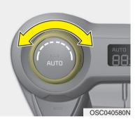
2. Turn the temperature control knob to set the desired temperature.
