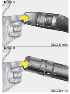
To flash the headlights, pull the lever towards you. It will return to the normal (low-beam) position when released. The headlight switch does not need to be on to use this flashing feature.
