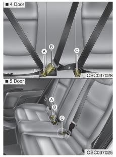
The seat belt should be locked into the buckle on each seat cushion to be properly fastened.
