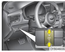
The instrument panel illumination intensity can be adjusted by pressing the control switch with the headlight switch in any position when the ignition switch or ENGINE START/STOP button is in the ON position.
