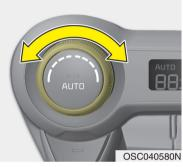
The temperature control knob allows you to control the temperature of the air flowing from the ventilation system. To change the air temperature in the passenger compartment, turn the knob to the right for warm air or left for cooler air. Air intake control
