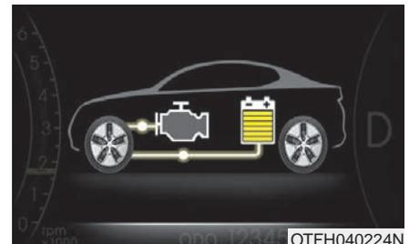
The engine friction is used to vehicle brake system and the regenerative brake charges the hybrid battery.
