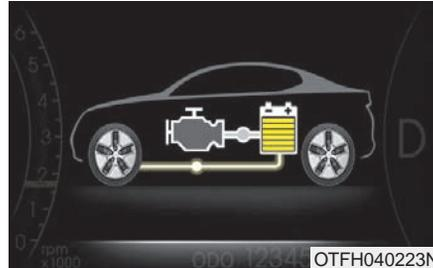
The vehicle is being slowed by engine compression and regenerative braking. The hybrid battery is being charged by regenerative braking.
