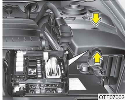
***Engine compartment panel fuse replacement***
