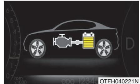
Vehicle is stopped with the Engine charging the hybrid battery. (Engine → Battery)
