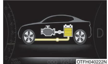
The engine and regenerative brake system charges the hybrid battery.
