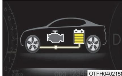
Motor power is used to move the vehicle.
