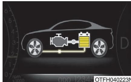
The vehicle is being slowed by engine compression and regenerative braking. The hybrid battery is being charged by regenerative braking.
