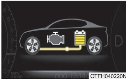
Hybrid battery is being charged by regenerative braking.
