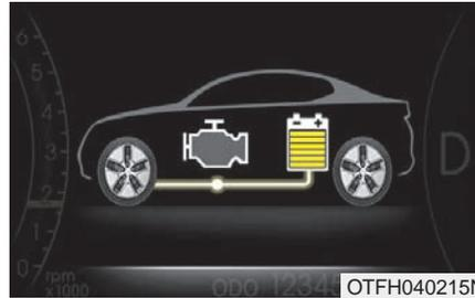
Electric power is used to move the vehicle. (Battery → Wheel)
