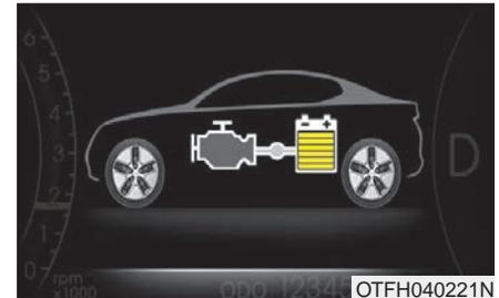
Vehicle is stopped with the Engine charging the hybrid battery.
