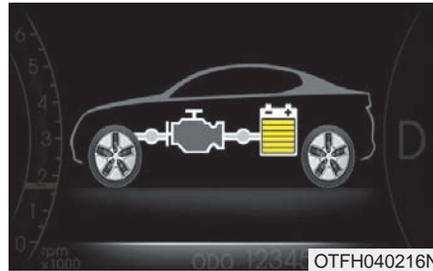
Engine is both driving the vehicle and charging the hybrid battery.
