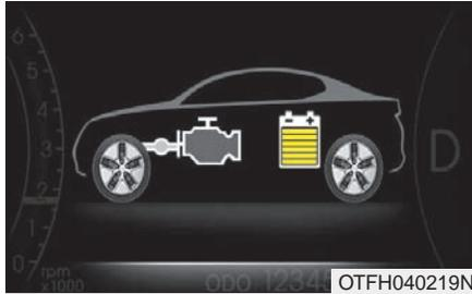
The vehicle is being slowed by engine compression.
