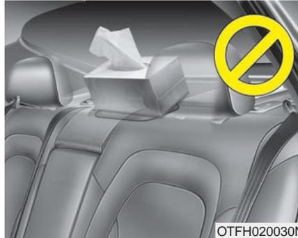
The hybrid battery air intake is located behind the rear seats. The hybrid battery air intake is used to cool the hybrid battery. If the hybrid battery air intake is blocked, the hybrid battery may overheat. Do not cover the air intake with objects.
