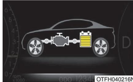
Engine is both driving the vehicle and charging the hybrid battery.
