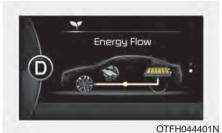
Motor power is used to move the vehicle. (Battery → Wheel)
