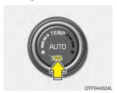
Push the AUTO button. The modes, fan speeds, air intake and air-conditioning will be controlled automatically by temperature setting.
