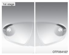
If a vehicle is detected within the boundary of the system, a warning light will illuminate on the outside rearview mirror.
