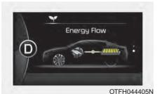
Vehicle is stopped with the Engine charging the hybrid battery. (Engine → Battery)
