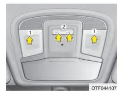
Push the lens (1) to turn the map lamp on or off. This light produces a spot beam for convenient use as a map lamp at night or as a personal lamp for the driver and front passenger.
