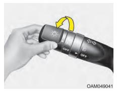
When the light switch is in the parking light position (1st position), the tail, position, license and instrument panel lights will turn ON.
