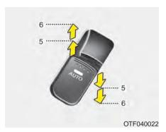
Pressing or pulling up the power window switch momentarily to the second detent position (6) completely lowers or lifts the window even when the switch is released. To stop the window at the desired position while the window is in operation, pull up or press and release the switch to the opposite direction of the movement.
