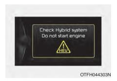
If the engine does not start and SOC (State Of Charge) is very low or vehicle defects the hybrid system's problem. a message will appear on the LCD display. Also, the chime will sound until the problem is solved.
