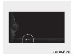
This display indicates the current outside air temperatures by 1°C (1°F).
