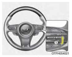
3.Move the lever (1) down (to SET-), and release it at the desired speed. The SET indicator light in the instrument cluster will illuminate. Release the accelerator at the same time. The desired speed will automatically be maintained.
