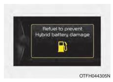
If the fuel tank is nearly empty, a message "Refuel to prevent Hybrid battery damage" will appear on the LCD display. Also, the chime will sound several times.
