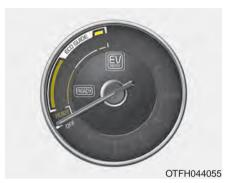
This is a gauge to let drivers know efficient the current driving conditions are. The fuel efficiency is high in the green zone but is low in the red zone.
