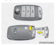
To remove the mechanical key, press and hold the release button (1) and remove the mechanical key (2).
