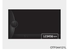
The odometer indicates the total distance the vehicle has been driven. You will also find the odometer useful to determine when periodic maintenance should be performed.
