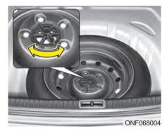
Turn the tire hold-down wing bolt counterclockwise.
