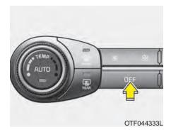
Press the OFF button to turn off the air climate control system. However you can still operate the mode and air intake buttons as long as the ignition switch is in the ON position.
