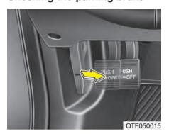
Check whether the stroke is within specification when the parking brake pedal is depressed with 20 kg (44 lb, 196 N) of force. Also, the parking brake alone should securely hold the vehicle on a fairly steep grade.
