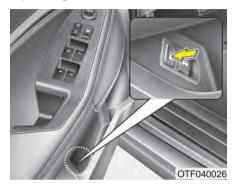
The fuel filler lid must be opened from inside the vehicle by pushing up the fuel filler lid opener.
