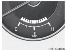
This gauge shows the temperature of the engine coolant when the ignition switch is ON
