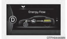
Engine is both driving the vehicle and charging the hybrid battery. (Engine → Wheel & Battery)
