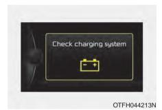
This warning illuminates when a malfunction is detected with the Charging System.
