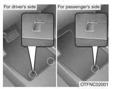
When using a floor mat on the floor carpet, make sure it attaches to the floor mat anchor(s) in your vehicle. This keeps the floor mat from sliding forward.
