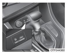
If your vehicle has an aux and/or USB(universal serial bus) port or iPod® port, you can use an aux port to connect audio devices and an USB port to plug in an USB and also an iPod® port to plug in an iPod®.
