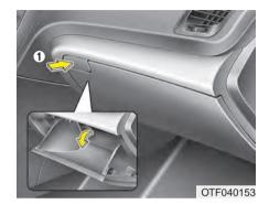
To open the glove box, push the button (1) and the glove box will automatically open. Close the glove box after use.
