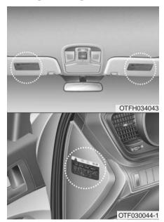
Air bag warning labels, some required by the Canada Motor Vehicle Safety Standards (CMVSS), are attached to the sunvisor to alert the driver and passengers of potential risks of the air bag system.
