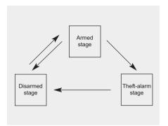
This system is designed to provide protection from unauthorized entry into the vehicle. This system is operated in three stages: the first is the "Armed" stage, the second is the "Theft-alarm" stage, and the third is the "Disarmed" stage. If triggered, the system provides an audible alarm with blinking of the hazard warning lights.
