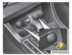
The power outlet is designed to provide power for mobile telephones or other devices designed to operate with vehicle electrical systems. The devices should draw less than 10 amps with the engine running.
