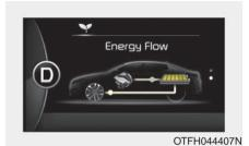
The engine and regenerative braking systems charge the hybrid battery during deceleration.
