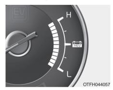
The state of charge (SOC) gauge indicates the hybrid battery's charge level. If the SOC is near L level, the vehicle automatically operates the engine to charge the battery. However, if the service indicator and MIL(Malfunction indicator lamp) turn on when the State of Charge(SOC) is near L(Low), have your vehicle checked by an authorized Kia dealer immediately.
