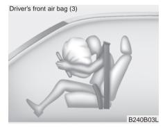
A fully inflated air bag, in combination with a properly worn seat belt, slows the driver's or the passenger's forward motion, reducing the risk of head and chest injury.
