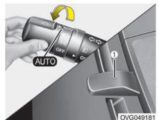
When the light switch is in the AUTO light position, the taillights and headlights will turn ON or OFF automatically depending on the amount of light outside the vehicle.
