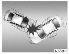
In a slant or angled collision, the force of impact may direct the occupants in a direction where the air bags would not be able to provide any additional benefit, and thus the sensors may not deploy any air bags.
