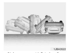
Air bags may not inflate in rollover accidents because the vehicle can not detect rollover accident.
