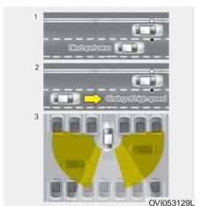
The Blind Spot Detection System (BSD) uses a radar sensor to alert the driver.
