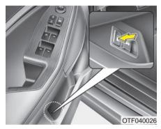
The fuel filler lid must be opened from inside the vehicle by pushing up the fuel filler lid opener.
