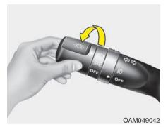
When the light switch is in the headlight position (2nd position) the head, tail, position, license and instrument panel lights will turn ON.
