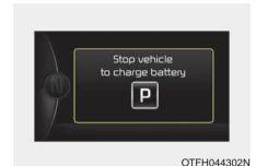
If the SOC (State Of Charge) is very low, a message Stop vehicle to charge battery will appear on the LCD display.
