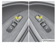
The seat warmer is provided to warm the rear seats during cold weather. With the ignition switch in the ON position, push either of the switches to warm the seat.
