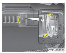
This service plug (1) located in the rear trunk as shown should always be pulled out to disconnect and turn off the hybrid system.
