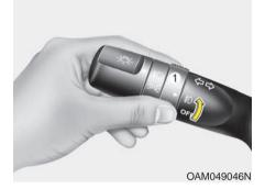
Fog lights are used to provide improved visibility when visibility is poor due to fog, rain or snow, etc. The fog lights will turn on when the fog light switch (1) is turned to the on position after the headlights are turned on.
