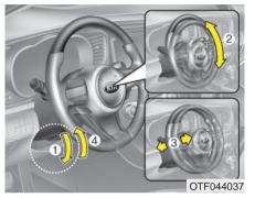
To change the steering wheel angle, pull down the lock release lever (1), adjust the steering wheel to the desired angle (2) and height (3), then pull up the lock-release lever (4) to lock the steering wheel in place. Be sure to adjust the steering wheel to the desired position before driving. Horn
