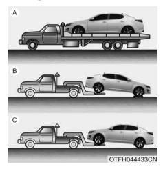
It is acceptable to tow the vehicle with the rear wheels on the ground (without dollies) and the front wheels off the ground.
