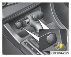
The power outlet is designed to provide power for mobile telephones or other devices designed to operate with vehicle electrical systems. The devices should draw less than 10 amps with the engine running.
