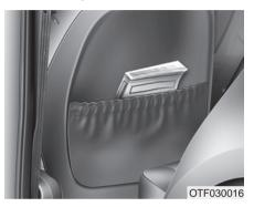
The seatback pocket is provided on the back of the front passenger's seatback.
