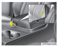
To open the center console storage, pull the lever up.
