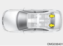
For maximum effectiveness in case of an accident, the headrest should be adjusted so the middle of the headrest is at the same height of the center of gravity of an occupant's head. Generally, the center of gravity of most people's head is similar with the height as the top of their eyes.
