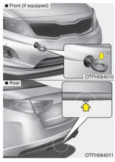
If towing is necessary, have it done by an authorized Kia dealer or a commercial tow truck service. If towing service is not available in an emergency, your vehicle may be temporarily towed using a cable or chain secured to the emergency towing hook under the rear of the vehicle. Use extreme caution when towing the vehicle. A driver must be in the vehicle to steer it and operate the brakes.
