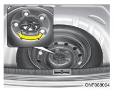
Turn the tire hold-down wing bolt counterclockwise.
