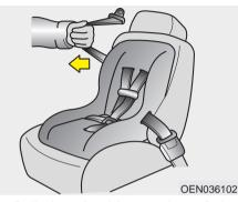
3. Pull the shoulder portion of the seat belt all the way out. When the shoulder portion of the seat belt is fully extended, it will shift the retractor to the "Auto Lock" (child restraint) mode.
