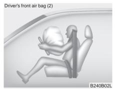
Upon deployment, tear seams molded directly into the pad covers will separate under pressure from the expansion of the air bags. Further opening of the covers then allows full inflation of the air bags. Driver's front air bag (3)
