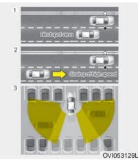
The Blind Spot Detection System (BSD) uses a radar sensor to alert the driver.
