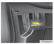
To release the parking brake, depress the parking brake pedal a second time while applying the foot brake. The pedal will automatically extend to the fully released position. WARNING - Parking brake use
