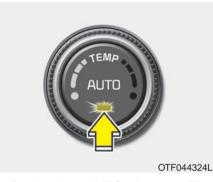
1. Push the AUTO button. The modes, fan speeds, air intake and air-conditioning will be controlled automatically by temperature setting.
