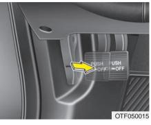
To engage the parking brake, first apply the foot brake and then depress the parking brake pedal down as far as possible. **CAUTION** - Parking brake
