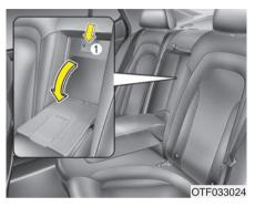
Pull the armrest down using the strap provided on the armrest. Pull the cover down while pushing the release lever down. Additional cargo space is provided to accommodate long/narrow cargo (skis, poles, lumber, etc.) not able to fit properly in the trunk when closed. Make sure the engine is off, the shift lever is in P and the parking brake is applied whenever loading or unloading cargo. The vehicle may move if the shift lever is inadvertently moved to another position.
