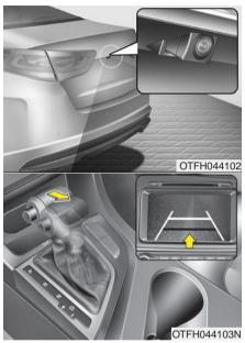
The Rear Camera Display will activate when the back-up light is ON with the ignition switch ON and the shift lever in the R (Reverse) position.
