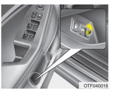
• To open the trunk from inside the vehicle, pull the trunk lid release button.
