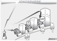
AM and FM radio signals are broadcast from transmitter towers located around your city. They are intercepted by the radio antenna on your vehicle. This signal is then processed by the radio and sent to your vehicle speakers.
