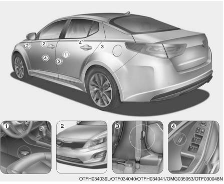
(1) SRS control module(2) Front impact sensor
