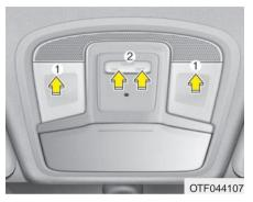
Push the lens (1) to turn the map lamp on or off. This light produces a spot beam for convenient use as a map lamp at night or as a personal lamp for the driver and front passenger. • DOOR (2) :
