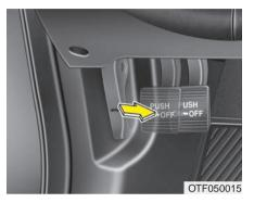
Check whether the stroke is within specification when the parking brake pedal is depressed with 20 kg (44 lb, 196 N) of force. Also, the parking brake alone should securely hold the vehicle on a fairly steep grade.
