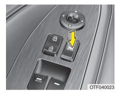
The driver can disable the power window switches on the rear passengers' doors by pressing the power window lock switch to the lock position (pressed). When the power window lock switch is pressed:
