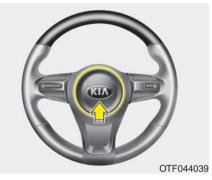
To sound the horn, press the horn symbol on your steering wheel. Check the horn regularly to be sure it operates properly.
