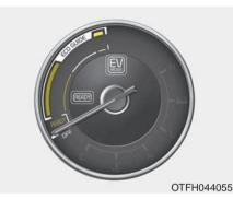
This is a gauge to let drivers know efficient the current driving conditions are. The fuel efficiency is high in the green zone but is low in the red zone.
