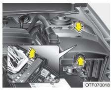
If the headlights or other electrical components do not work and the fuses are OK, check the fuse block in the engine compartment. If a fuse is blown, it must be replaced. Fuse switch
