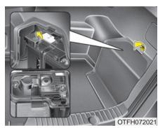
Visually inspect the battery cap for secure closing. If the battery cap is not securely latched, the electrical system may be damaged to due influx of moisture into the system. Multi fuse
