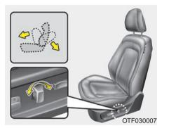
Push the control switch forward or backward to move the seatback to the desired angle. Release the switch once the seat reaches the desired position. Seat cushion height (for driver's side)
