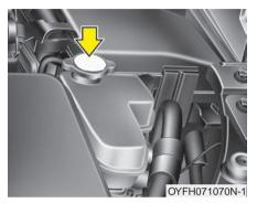
The high-pressure cooling system has a reservoir filled with year-round antifreeze coolant. The reservoir is filled at the factory.
