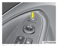
**Electric Type (if equipped)** To fold the outside rearview mirror, depress the button.
