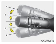
If an indicator stays on and does not flash or if it flashes abnormally, one of the turn signal bulbs may be burned out and will require replacement.
