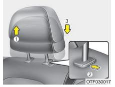
Adjusting the height up and down (if equipped)
