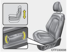
Pull the front portion of the control switch up to raise or down to lower the front part of the seat cushion. Pull the rear portion of the control switch up to raise or down to lower the rear part of the seat cushion. Release the switch once the seat reaches the desired position. Lumbar support (for driver's seat, if equipped)
