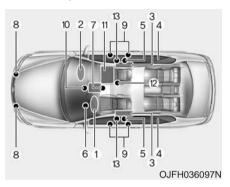
The SRS consists of the following components:
