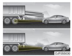
Always be cautious for vehicles that are taller with higher clearance, or vehicles carrying loads that stick out of the back of the vehicle.
