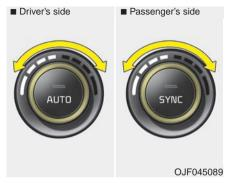
2. Turn the temperature control knob to the desired temperature.
