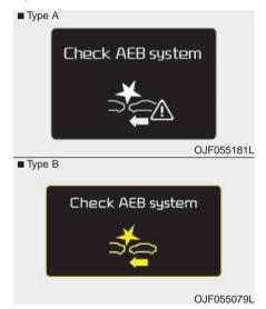
When the AEB is not working properly, the AEB warning light (♣) will illuminate and the warning message will appear for a few seconds. After the message disappears, the master warning light (⚠) will illuminate. In this case, have your vehicle inspected by an authorized Kia dealer.
