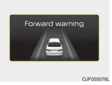
The warning message appears on the LCD display with the warning alarms.
