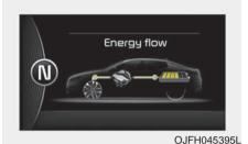
Engine is both driving the vehicle and charging the hybrid battery.
