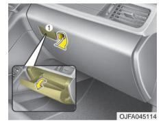
The glove box can be locked and unlocked with a master key. (if equipped)
