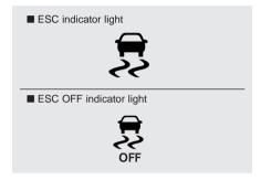
When engine start/stop button is turned to ON, the indicator light illuminates, then goes off if the ESC system is operating normally.
