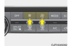
The fan speed can be set to the desired speed by operating the fan speed control button.
