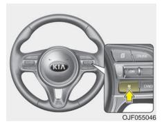
This function allows you to program the vehicle to maintain relative distance to the vehicle ahead without depressing the accelerator pedal or brake pedal. The vehicle to vehicle distance will automatically activate when the ASCC is on.
