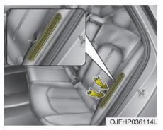
The high-voltage battery air intake is located on the left side of the rear seats. The air intake cools down the high-voltage battery.
