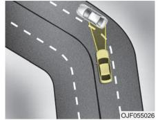
While driving on a curve, the AEB may recognize the vehicle in front in the next lane. Exercise caution, and, if necessary, depress the brake pedal.
