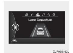
If you select this symbol, the LDWS mode on the LCD display will appear. If the system detects that your vehicle is leaving the lane when the LDWS is operating and vehicle speed exceeds 64 km/h (40 mph), the warning operates as follows:
