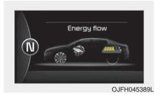
The mode means the vehicle at stop. (There is no energy flow.)
