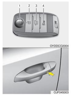
Pressing the button of the front outside door handles with all doors (and trunk) closed and any door unlocked, locks all the doors (and trunk).
