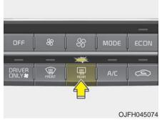
The defroster heats the window to remove frost, fog and thin ice from the rear window, while the engine is running.
