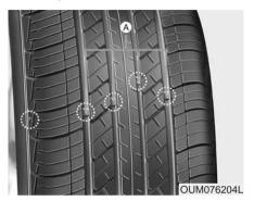
If the tire is worn evenly, a tread wear Indicator (A) will appear as a solid band across the tread. This shows there is less than 1.6 mm (1/16 inch) of tread left on the tire. Replace the tire when this happens.
