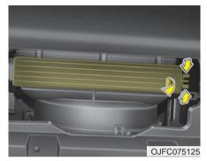
3. Remove the climate control air filter cover while pressing the lock on the right side of the cover.
