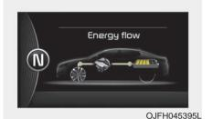
Engine is both driving the vehicle and charging the hybrid battery. (Engine → Wheel & Battery)
