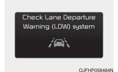
When the LDW is not working properly, the warning light will illuminate and the warning message will come on for a few second. After the message disappears, the master warning light will illuminate.
