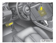
To release the EPB (electronic parking brake), press the EPB switch while doing the following:
