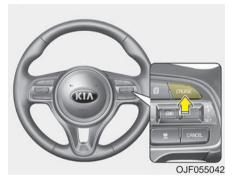
Press the CRUISE button, to turn the system on. The CRUISE indicator in the instrument cluster will illuminate.
