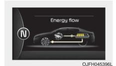
The engine and regenerative brake system charge up the high-voltage battery.
