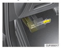
Check whether the stroke is within specification when the parking brake pedal is depressed with 30 kg, 294 N (66 lb) of force. Also, the parking brake alone should securely hold the vehicle on a fairly steep grade. If the stroke is more or less than specified, have the parking brake adjusted by an authorized Kia dealer.
