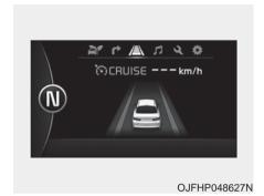
This mode displays the state of the Smart Cruise Control with Stop & Go (SCC) and Lane Departure Warning (LDW) system.
