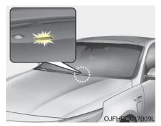
· When scheduled charging is set and the normal charger or the portable charging cable (ICCB: In-Cable Control Box) is connected for charging, the indicator lamp blinks (for 3 minutes) to indicate that scheduled charging is set.
