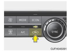
This is used to select the outside (fresh) air position or recirculated air position.
