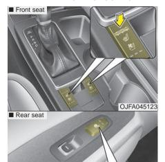
The seat warmer is provided to warm the front seats during cold weather. With the ignition switch in the ON position, push either of the switches to warm the driver's seat or the front passenger's seat.
