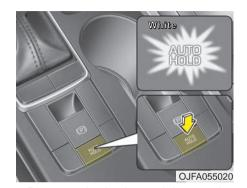
1.Depress the brake pedal, start the engine and then press the Auto Hold button. The white AUTO HOLD indicator will come on indicating the system is in standby. Before the Auto Hold will engage, the driver's door and engine hood must be closed and the driver's seat belt must be fastened.
