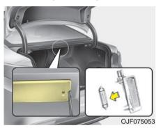
If the trunk lamp (LED) (1) does not operate, have the vehicle checked by an authorized Kia dealer.
