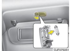
WARNING - Interior lamps Prior to working on the Interior lamps, ensure that the "OFF" button is depressed to avoid burning your fingers or receiving an electric shock.
