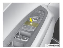
The driver can disable the power window switches on the passenger doors by pressing the power window lock button located on the driver's door to the LOCK position (pressed).
