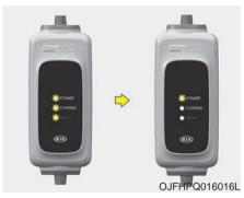
8. Charging starts automatically. Check if the power lamp and charging lamp (orange) are ON.
