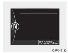
The odometer Indicates the total distance that the vehicle has been driven and should be used to determine when periodic maintenance should be performed.
