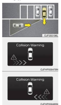
If the vehicle detected by the sensors approaches your vehicle, the warning chime will sound, the warning light on the outside rearview mirror will blink and a message will appear on the LCD display.
