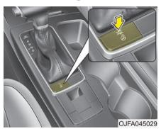
With the Engine Start/Stop button is ON position, pressing the heated steering wheel button warms the steering wheel. The indicator on the button will illuminate.
