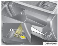
2. With the glove box open, pull the support strap (1).
