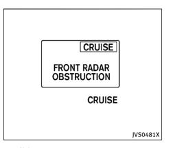
off. When the radar signal is temporarily interrupted, clean the sensor area of the front bumper and restart the engine. If the "FRONT RADAR OBSTRUCTION" warning continues to be displayed, have the ICC system checked. It is recommended you visit an INFINITI retailer for this service.
