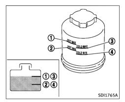
Check the fluid level in the reservoir.
