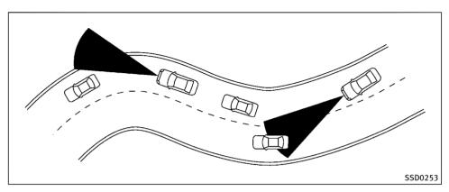
When driving on some roads, such as winding, hilly, curved, narrow roads, or roads which are under construction, the sensor may detect vehicles in a different lane, or may temporarily not detect a vehicle traveling ahead. This may cause the system to work inappropriately.
