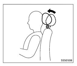
Active Head Restraints operate only in certain rear-end collisions. After the collision, the head restraints return to their original position.
