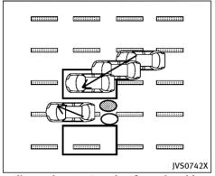
Illustration 8 - Entering from the side Illustration 8: If the driver activates the turn signal while another vehicle is in the detection zone, then the side indicator light flashes and a chime will sound twice.
