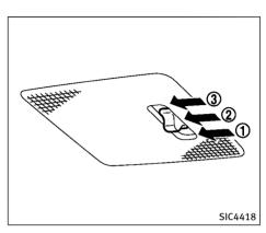
The cargo light switch has three positions: ON (1), center (2) and OFF (3).
