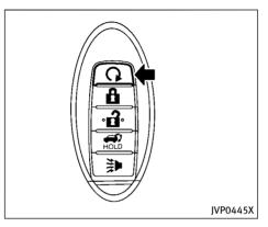
The remote engine start () button is on the Intelligent Key if the vehicle has remote engine start function. This function allows the engine to start from outside the vehicle.
