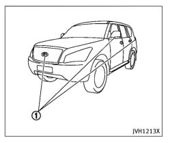
If dirt, rain or snow accumulates on any of the cameras (1), the Around View<sup>®</sup> Monitor may not display objects clearly. Clean the camera by wiping with a cloth dampened with a diluted mild cleaning agent and then wiping with a dry cloth.
