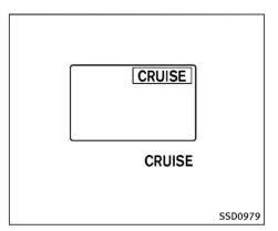
When the ignition switch is pushed to the ON position, the indicators come on as illustrated to check for a burned-out bulb, and it turns off when the engine is started.
