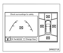
When the "\omega" icon is displayed on the screen, the camera image may be receiving temporary electronic disturbances from surrounding devices. This will not hinder normal driving operation but the system should be inspected. It is recommended vou visit an INFINITI retailer.
