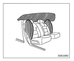
FRONT SFAT-MOUNTED SIDE-IM-PACT SUPPLEMENTAL AIR BAG AND ROOF-MOUNTED CURTAIN SIDE-IM-PACT AND ROLLOVER SUPPLEMEN-TAL AIR BAG SYSTEMS
