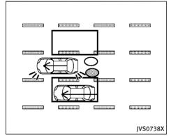
Illustration 2 - Approaching from behind Illustration 2: If the driver activates the turn signal, then the system chimes (twice) and the side indicator light flashes.
