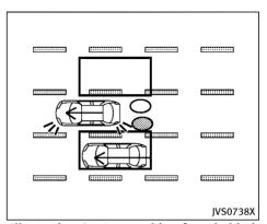
Illustration 2 - Approaching from behind Illustration 2: If the driver activates the turn signal then the system chimes (twice) and the side indicator light flashes.
