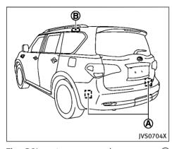
The BSI system uses radar sensors (A) installed near the rear bumper to detect other vehicles in an adjacent lane. In addition to the radar sensors, the BSI system uses a camera (B) installed behind the windshield to monitor the lane markers of your traveling lane.
