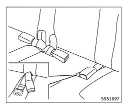
Storing 3rd row seat belt buckles Before folding down the seat, put the buckles in the storage of the seat cushion to avoid dropping it under the seat cushion.
