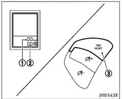
Odometer/twin trip odometer
