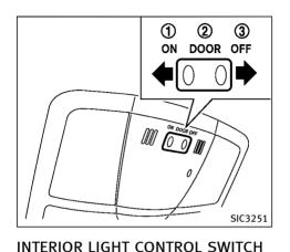
The interior light control switch has three positions: ON, DOOR and OFF.
