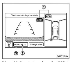
When this item is turned on, the MOD is activated. When this item is turned off (indicator turns off), the MOD system is deactivated. When the MOD system is deactivated, "MOD" (2) will disappear on the (3) and the MOD icon (1) will disappear as well. When the sonar is turned off on the setting menu as well, the (3) will disappear.
