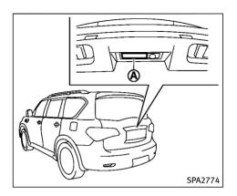
inserting the mechanical key into the driver's door key cylinder and turning it to the rear of the vehicle twice.
