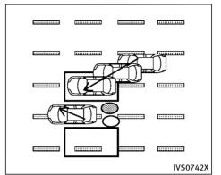
Illustration 10 - Entering from the side Illustration 10: The BSI system will not operate if your vehicle is on a lane marker when another vehicle enters the detection zone. In this case only the BSW system operates.
