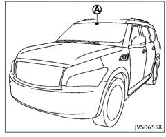
The LDW and LDP systems use a camera (A) installed behind the windshield to monitor the lane markers of your traveling lane.
