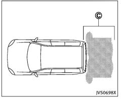
The radar sensors (A) detect an approaching vehicle from up to approximately 49 ft (15 m) away. The sonar sensors (B) detect stationary objects behind the vehicle up to approximately 4.9 ft (1.5 m). Refer to the illustration for approximate zone coverage areas (c).
