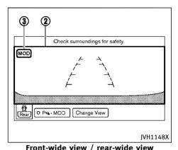
When the MOD system detects moving objects near the vehicle, the yellow frame will be displayed on the view where the objects are detected and a chime will sound once. While the MOD system continues to detect moving objects, the yellow
