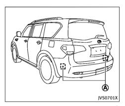
The BSW system uses radar sensors (A) installed near the rear bumper to detect other vehicles in an adjacent lane.
