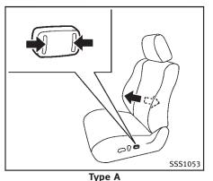
Type A Push the front or back end of the switch to adjust the seatback lumbar area.
