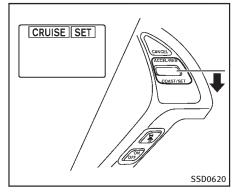
To set cruising speed, accelerate your vehicle to the desired speed, push the COAST/SET switch and release it. (The SET indicator will come on in the display.) Take your foot off the accelerator pedal. Your vehicle will maintain the set speed.
