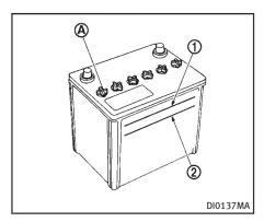
Check the fluid level in each cell (Remove the battery cover if it is necessary). It should be between the UPPER LEVEL (1) and LOWER LEVEL (2) lines.
