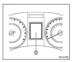
The dot matrix liquid crystal display ① is located between the tachometer and the speedometer, and it displays the automatic transmission position indicator (if so equipped), the Intelligent Cruise Control (ICC) system (if so equipped) information, the Intelligent Key operation information and other warnings and information.
