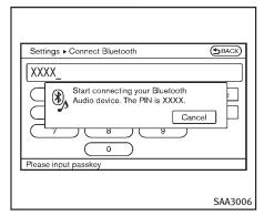
5. The standby message screen will appear. Operate the compatible Bluetooth® audio device. For the connecting procedure of the audio device, see the Bluetooth® audio instructions.
