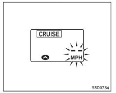
When the COAST/SET switch is pushed under the following conditions, the system cannot be set and the ICC indicators will blink for approximately 2 seconds:
