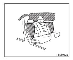
FRONT SEAT-MOUNTED SIDE-IM-PACT SUPPLEMENTAL AIR BAG AND ROOF-MOUNTED CURTAIN SIDE-IM-PACT SUPPLEMENTAL AIR BAG SYS-**TFMS**
