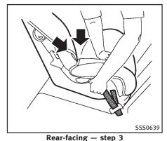
3. For child restraints that are equipped with webbing-mounted attachments, remove any additional slack from the anchor attachments. Press downward and rearward firmly in the center of the child restraint with your hand to compress the vehicle seat cushion and seatback while tightening the webbing of the anchor attachments.
