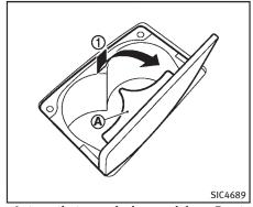
**Automatic transmission models** — Front To open the cup holder, push the lid (1). The flap (A) will be folded down when inserting a large container.
