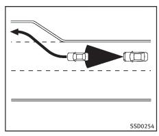
When driving on the freeway at a set speed and approaching a slower traveling vehicle ahead, the ICC will adjust the speed to maintain the distance, selected by the driver, from the vehicle ahead. If the vehicle ahead changes lanes or exits the freeway, the ICC system will accelerate and maintain the speed up to the set speed. Pay attention to the driving operation to maintain control of the vehicle as it accelerates to the set speed.
