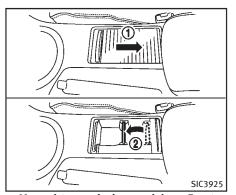
Manual transmission models — Front To open the cup holder, slide the lid (1). Install the partition plate into the slit (2).
