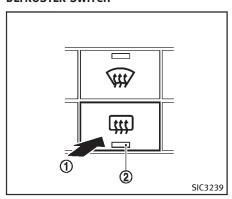
To defog/defrost the rear window glass and outside mirrors (if so equipped), start the engine and push the switch (1) on. The indicator light (2) will come on. Push the switch again to turn the defroster off.
