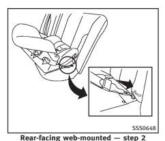
2. Secure the child restraint anchor attachments to the LATCH lower anchors. Check to make sure the LATCH attachment is properly attached to the lower
