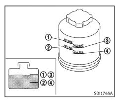
Check the fluid level in the reservoir.
