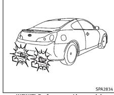
INFINITI Performance Line model The INFINITI Performance Line model has unique exhaust pipes. These parts are close to the ground and may be damaged if they contact objects such as parking blocks, etc.
