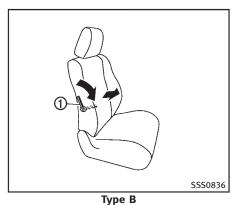
Type B Move the lever (1) up or down to adjust the seatback lumbar area.
