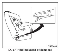
The child restraint top tether strap must be used when installing child restraints with the LATCH lower anchor attachments or
