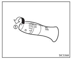
The autolight system can turn on the headlights automatically when it is dark and turn off the headlights when it is light. If the ignition switch is pushed to the OFF position and one of the doors is opened and this condition is continued, the headlights remain on for 5 minutes.
