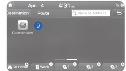
Press **[NAV]** button in the navigation head unit, and find a destination by using the **[Destination]** menu.
