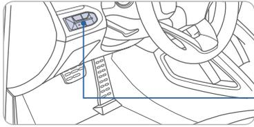
Push +/- on the control switch to adjust the brightness.
