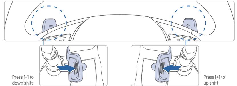
The paddle shifters operate when the shift lever is in the D position or the Sport Mode.
