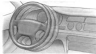
*A collapsible steering column, smooth or recessed controls, and energy-absorbing materials are part of a car's occupant protection system.*
