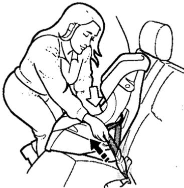
To install a forward-facing child seat in the center back seat with the lap belt, follow instruction number 1 on page 32 for routing and latching the seat belt. Then pull hard on the loose end of the belt to remove any slack (it may help to put weight on the child seat while pulling on the belt).
