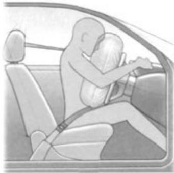
*When sensors detect a severe frontal collision, the airbags instantly inflate to provide extra protection for an occupant's head and chest.*
