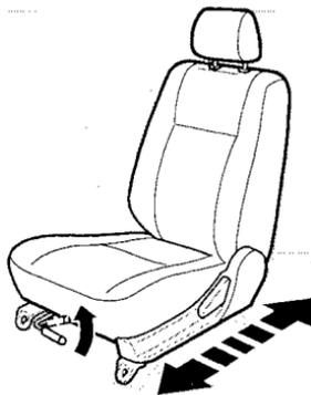
Let go of the lever and the seat will lock into the desired position.
