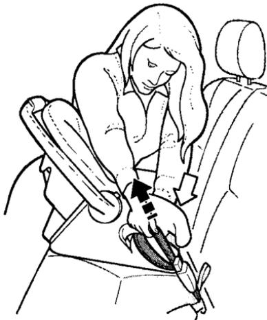
To install a rear-facing child seat in the center back seat with the lap belt, follow instruction number 1 on page 28 for routing and latching the seat belt. Then pull hard on the loose end of the
