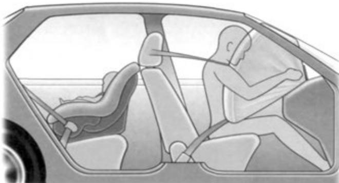
*To avoid the possibility of an infant being seriously injured or killed by an inflating passenger airbag, a rear-facing child seat should always be secured in the back seat, never in the front.*
