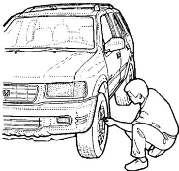
Off-road driving can be hard on a vehicle, requiring extra attention to maintenance. Before driving off-road, be sure all scheduled maintenance and service has been done, and that you have also inspected your vehicle. Pay special attention to the condition of the tires and use a gauge to check the tire pressures.
