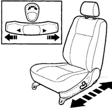
Push the horizontal switch forward or backward to move the seat forward or backward.
