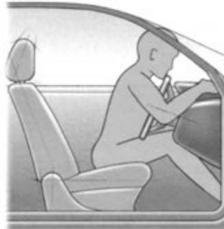
*Without a seat belt or an airbag, the occupant will continue forward at 30 mph until they strike the car's interior, and potentially suffer very serious injuries.*
