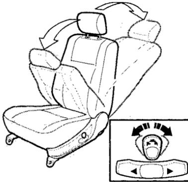
Adjust the seat-back angle by pushing the vertical switch in the direction you want to move.
