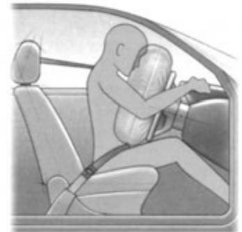
*However, if the occupant is wearing a seat belt, the belt will restrain them and reduce the chance of injury. An airbag can further reduce the risk of injuries to the occupant's head and chest.*
