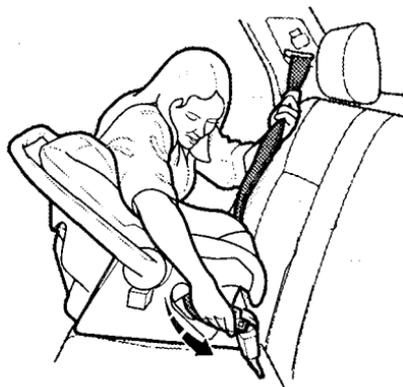
1. With the child seat in the desired back seating position, route the belt through the child seat according to the seat maker's instructions, then insert the latch plate into the buckle.
