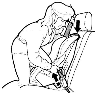
2. To activate the lockable retractor, slowly pull the shoulder part of the belt all the way out until it stops, then let the belt feed back into the retractor (you might hear a clicking noise as the belt retracts).
