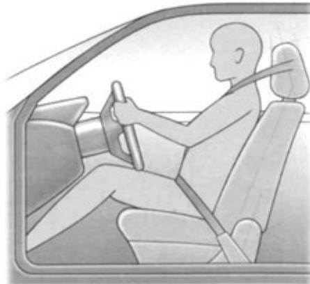
*Wearing a seat belt, and sitting up, well back from the steering wheel or dashboard, reduces the chance of injuries caused by a crash or an inflating airbag.*
