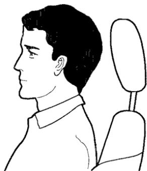
They are most effective when you adjust them so the back of the occupant's head rests against the center of the restraint. A taller person should adjust the restraint as high as possible.
