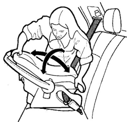
5. Push and pull the child seat forward and from side to side to verify that it is secure enough to stay upright during normal driving maneuvers. If the child seat is not secure, unlatch the belt, allow it to retract fully, then repeat these steps.
