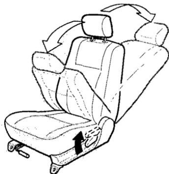
Raise the lever and use body pressure to move the seat-back to the desired position. Let go of the lever and the seat-back will lock into the desired position.
