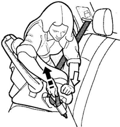
4. After confirming that the belt is locked, grab the shoulder part of the belt near the buckle and pull up to remove any slack from the lap part of the belt.
