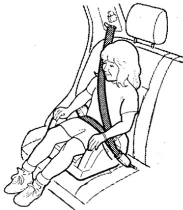
If a child needs a booster seat, we recommend choosing a style that allows the child to use the lap/shoulder belt directly, without a shield, as shown.
