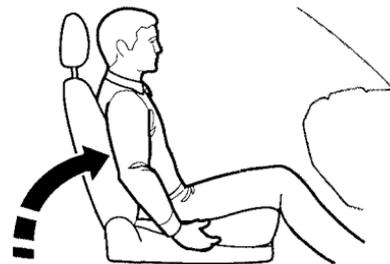
Adjust the driver's seat-back to a comfortable, upright position, leaving ample space between your chest and the airbag cover in the center of the steering wheel. If you sit too close to the steering wheel, you could be injured if the airbag inflates.
