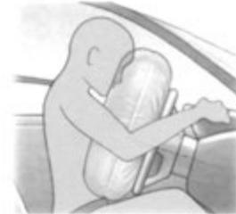
*Airbags are designed to give added protection for the head and chest in a severe frontal collision.*
