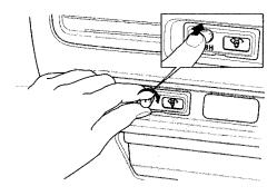
The knob on the dashboard to the left of the steering column controls the brightness of the instrument panel lights. Push the knob to get it to pop out. Turn the knob to adjust the brightness. Push the knob back in to lock your adjustment.
