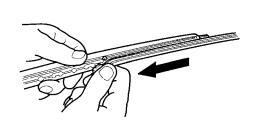
Slide the new blade into the holder. Make sure it is engaged in the slot along its full length.
