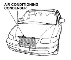
Run the air conditioning at least once a week during the cold weather months. Run it for at least ten minutes while you are driving at a steady speed with the engine at normal operating temperature. This circulates the lubricating oil contained in the refrigerant.
