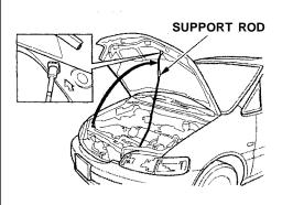
3. Pull the support rod out of its clip and insert the end into the hole on the left side of the hood.
