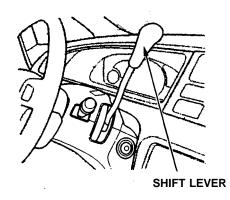
The shift lever has seven positions. It must be in Park or Neutral to start the engine. When you are stopped in D<sub>4</sub>, D<sub>3</sub>, 2, 1, N or R, press firmly on the brake pedal, and keep your foot off the accelerator pedal.
