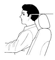
Head restraints can help protect you from whiplash and other injuries. For the best protection, adjust the top of the restraint so it is even with the tops of your ears, or as high as possible. For instructions on adjusting the head restraints, see page 56.
