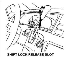
5. Remove the key from the Shift Lock Release slot. Depress the
