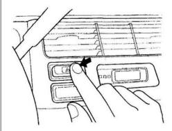
Push the red button to the left of the clock to turn on the hazard warning lights (four-way flashers). This causes all four outside turn signals and both indicators in the instrument panel to flash. Use the hazard warning lights if you need to park in a dangerous area near heavy traffic, or if your car is disabled.
