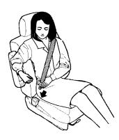
Pull the latch plate across your body and insert it into the buckle.
