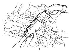
THREE WAY CATALYTIC CONVERTER
