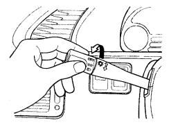
The rotating switch on the left lever controls the lights. Turning this switch to the "₹00€" position turns on the parking lights, taillights, instrument panel lights, side-marker lights, and rear license plate lights. Turning the switch to the " ≣○ " position turns on the headlights.
