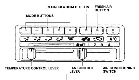
You should shut the system completely off only for the first few minutes of driving in cold weather, until the engine coolant warms up enough to operate the heater. Keep the fan on at all other times so stale air does not build up in the interior.
