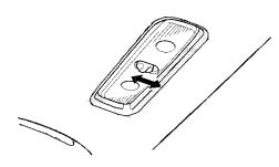
The tailgate light has a two position switch. In the OFF (down) position, the light does not come on. In the ON (up) position, the light comes on when you open the tailgate.
