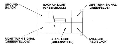
Your car has a trailer lighting connector. To use the connector, remove the left rear light cover. Refer to the drawing above for the wiring color code and purpose of each connector pin.
