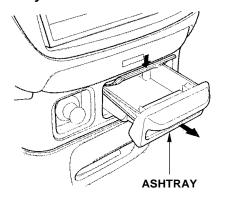
Open the front ashtray by pulling on the bottom edge. Push it in to close it. To remove the ashtray for emptying, push down on the metal plate inside, then pull the ashtray out completely.
