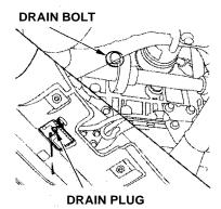
3. Loosen the drain plug on the bottom of the radiator. The coolant will drain through the splash guard. Remove the drain bolt and washer from the engine block.
