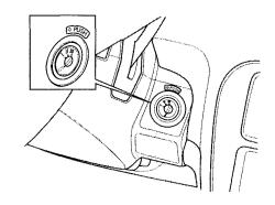
The ignition switch is on the right side of the steering column. It has four positions:
