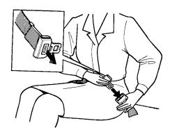
Pull the latch plate across your hips and insert it into the buckle marked CENTER.
