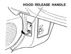
Shift to Park or Neutral and set the parking brake. Pull the hood release handle located under the lower left corner of the dashboard. The hood will pop up slightly.
