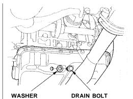
2. Open the hood and remove the engine oil fill cap. Remove the oil drain bolt and washer from the bottom of the engine. Drain the oil into an appropriate container.
