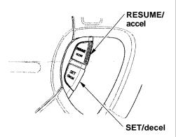
Press and hold the SET/decel button on the steering wheel until the CRUISE CONTROL light on the instrument panel comes on. This shows the system is now activated.
