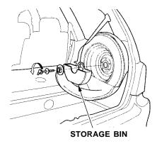
8. Unscrew the wing bolt. Remove the storage bin and spare tire.
