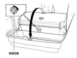
Turn the knob on the back of the seat cushion while you pull the entire seat towards you. Pivot the seat into the floor recess.
