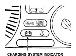
This indicator should come on when the ignition is ON (II), and go out after the engine starts. If it comes on brightly when the engine is running, it indicates that the charging system has stopped charging the battery.
