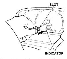
Your dealer will reset the indicator when he performs the scheduled maintenance. If someone else performs the maintenance, reset the indicator by inserting your key in the slot beside the indicator.
