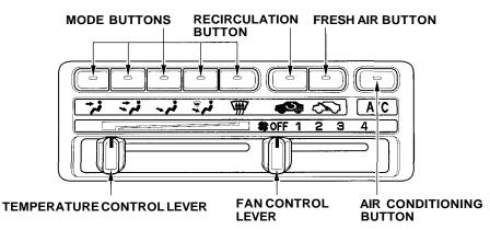
When the interior has cooled down to a more comfortable temperature, close the windows and set the controls as described for normal cooling.
