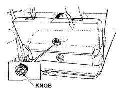
Unlock the seat-back by turning the knob. Push the seat-back forward.
