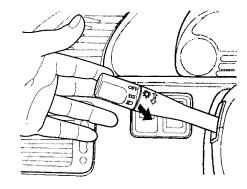
To change between low beams and high beams, pull the turn signal lever until you hear a click, then let go. The blue high beam indicator will light (see page 36).
