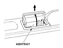
The rear ashtray is in the armrest on the left rear door. To use the rear ashtray, swing the lid open. To remove the rear ashtray, open the lid and pull it straight up.
