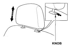
The head restraints are designed to help reduce the risk of neck injuries. Your Honda has adjustable head restraints in all the outside seating positions. Adjust the head restraint so the top is even with the tops of your ears.
