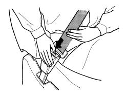
To unlatch the seat belt, push the red PRESS button on the buckle. Guide the belt across your body to the door pillar.
