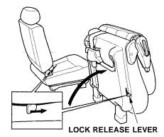
Pull the seat-back angle adjustment lever on the second row seat to tilt the seat-back forward. Pull the lock release lever and pivot the seat up out of the way.
