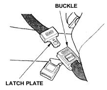
The lap belt has one manuallyadjusted belt that fits across the hips. It is similar to safety belts used in airplanes.
