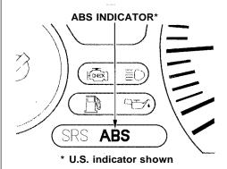
The ABS is self-checking. You may feel a slight movement of the brake pedal just after you start the engine. This is the ABS performing a check. It also checks itself whenever you use the brakes.
