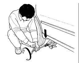
15.Lower the car to the ground and remove the jack.
