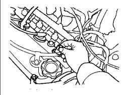
4. Put the new spark plug into the socket; then screw it into the hole. Screw it in by hand so you do not crossthread it.
