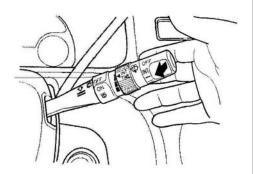
To clean the windshield, pull back on the wiper control lever. The washers spray until you release the lever. The wipers run at low speed while you're pulling the lever, then complete one more sweep of the windshield after you release it.
