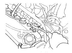
Torque the spark plug. (If you do not have a torque wrench, tighten the spark plug two-thirds of a turn after it contacts the cylinder head.)
