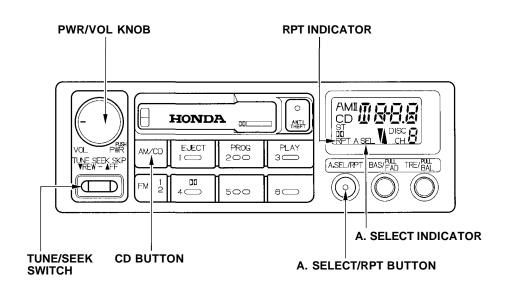
Press the CD button until "CD" appears in the display. The system will start to play the first track of the first disc in the magazine. When that disc ends, the next disc in the magazine is loaded and played. After the last disc finishes, the system returns to disc 1.
