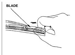
Remove the blade from its holder by grasping the tabbed end of the blade. Pull firmly until the tabs come out of the holder.
