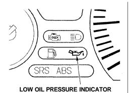
This indicator should light when the ignition is ON (II), and go out after the engine starts. It should never come on when the engine is running. If it starts flashing, it indicates that the oil pressure dropped very low for a moment, then recovered. If the indicator stays on with the engine running, it shows that the engine has lost oil pressure and serious engine damage is possible. In either case, you should take immediate action.
