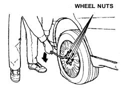
9. Loosen the five wheel nuts 1/2 turn with the wheel wrench.
