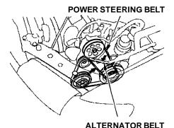
Check the condition of the two drive belts. Examine the edges of each belt for cracks or fraying. Check the tension of each belt by pushing on it with your thumb midway between the pulleys. The belts should have the following "play" or deflection.
