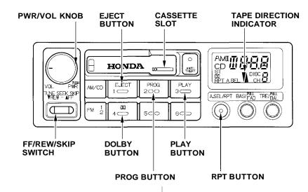
When the system reaches the end of the tape, it will automatically reverse direction and play the other side. If you want to remove the cassette from the drive, press the EJECT button.
