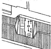
5. Check the vertical angle gauge. The bubble should be centered underneath the longest scribe mark on the gauge.
