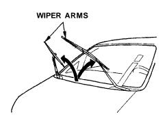
Check the condition of the windshield wiper blades at least every six months. Look for signs of cracking in the rubber, or areas that are getting hard. Replace the blades if you find these signs, or they leave streaks and unwiped areas when used.
