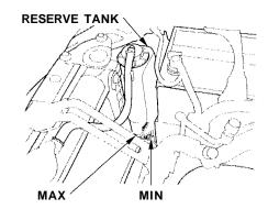
Look at the coolant level in the radiator reserve tank. Make sure it is between the MAX and MIN lines. If it is below the MIN line, see Adding Engine Coolant on page 152 for information on adding the proper coolant.
