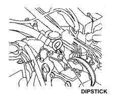
Check the engine oil level every time you fill the car with fuel. Wait at least two minutes after turning the engine off before you check the oil.
