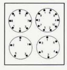
Tighten the nuts firmly in a criss-cross sequence as shown by rotating the wheel wrench clockwise.
