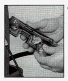
Pull the old bulb straight out of the socket.
