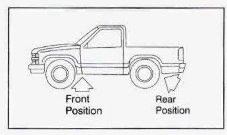
With UP on the ratchet facing you, raise the vehicle by rotating the ratchet and wheel wrench clockwise. Raise the vehicle far enough off the ground so there is enough room for the spare tire to fit.
