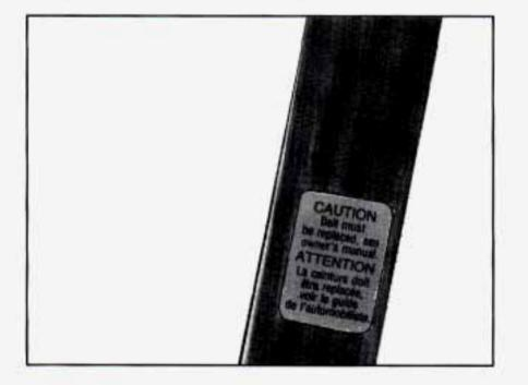
If you ever see a label on the right front passenger's safety belt in an Extended Cab model that says to replace the belt, be sure to do so. Then the new belt will be there to help protect you in a collision. You would see this label on the belt near the door opening.
