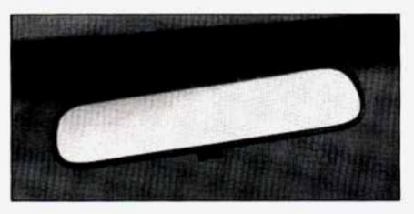
Press or pull the tab under the mirror to reduce glare from headlamps behind you after dark.
