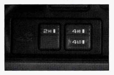
If your four-wheel-drive vehicle has the electronic transfer case, the transfer case switches are below and to the left of the climate control system.
