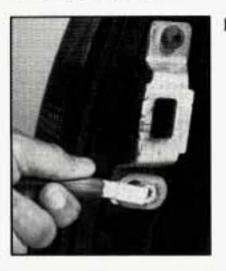
Raise the tailgate slightly and release both retaining cable clips. To release the cable clips, lift the cable so it points straight out and push the cable clips forward.
