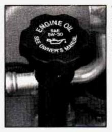
The engine oil fill cap for the 4.3L, 5.0L and the 5.7L engine is located on the driver's side engine valve cover.
