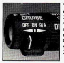
With cruise control, you can maintain a speed of about 25 mph (40 km/h) or more without keeping your foot on the accelerator. This can really help on long trips. Cruise control does not work at speeds below about 25 mph (40 km/h). When you apply your brakes, the cruise control shuts off.
