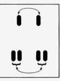
If your vehicle has dual rear wheels and the load range or tread design for your front tires is different from your rear tires, always use the correct rotation pattern shown here when rotating your tires.
