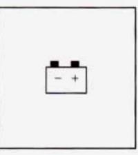
This light should come on briefly when you turn on the ignition, before starting the engine, as a check to show you it is working.
