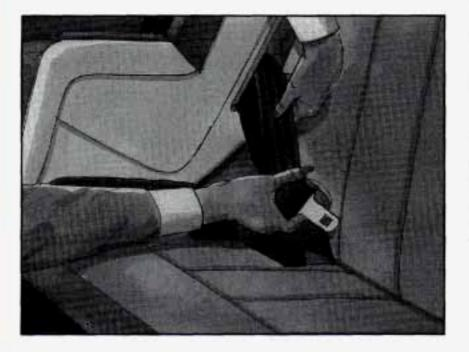
Tilt the latch plate to adjust the belt if needed. If the shoulder belt goes in front of the child's face or neck, put it behind the child restraint.
