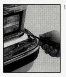
Squeeze the tab on the side of the lamp socket while turning the socket counterclockwise.
