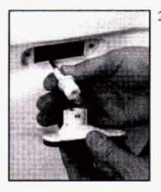
Turn the bulb socket counterclockwise and remove it from the lens assembly.
