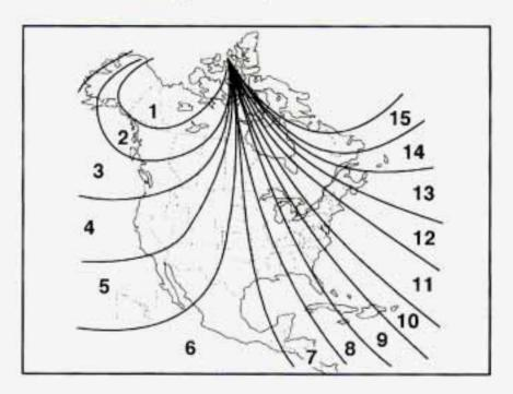
Press the CAL switch on the bottom of the mirror until the new zone number appears in the display. After you stop pressing the button in, the display will show a compass direction within a few seconds.
