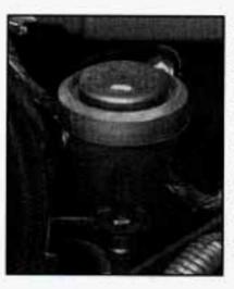
Refer to the Maintenance Schedule, Owner Checks and Services, to determine how often you should check the fluid level in your clutch master cylinder reservoir and for the proper fluid. See "Owner Checks and Services" and "Recommended Fluids and Lubricants" in the Index.
