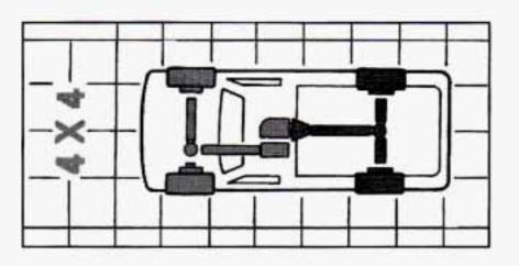
The front axle portion of the indicator diagram will light up when you shift into four-wheel drive.
