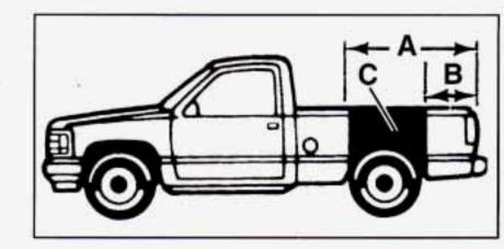
Refer to the Truck Camper Loading Information label in glove box for A and B dimensions.
