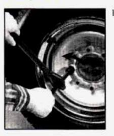
Use the ratchet and wheel wrench to loosen all the wheel nuts. Turn the wheel wrench counterclockwise, with DOWN facing you, to loosen the wheel nuts. Don't remove the wheel nuts yet.
