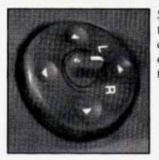
Select the mirror you want to move by moving the center of the switch, located on the driver's door armrest, to R (right) or L (left).
