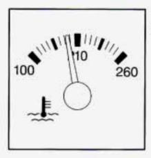
This gage shows the engine coolant temperature.
