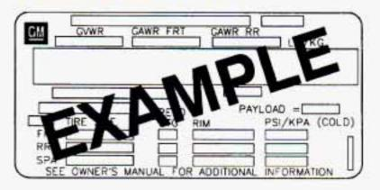
The Certification/Tire label is found on the rear edge of the driver's door or in the Incomplete Vehicle Document in the cab.
