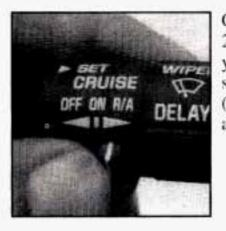
Once you're going about 25 mph (40 km/h) or more, you can move the cruise switch from ON to R/A (Resume/Accelerate) for about a 1/2 second.
