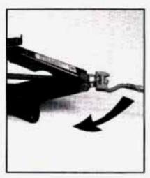
With the UP marking on the ratchet facing you, rotate the ratchet clockwise. That will lift the jack head a little.
