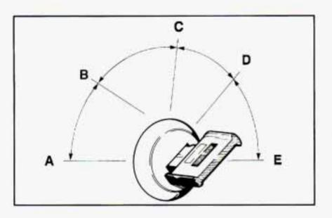
ACCESSORY (A): This position lets you use things like the radio, power windows and the windshield wipers when the engine is off. Push in the key and turn it toward you. Your steering wheel will remain locked, just as it was before you inserted the key. LOCK (B): This position locks your ignition, steering wheel and transmission. It's a theft-deterrent feature. You will only be able to remove your key when the ignition is turned to LOCK.
