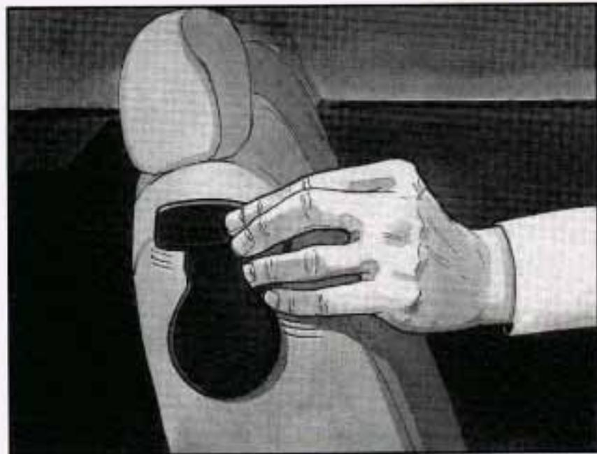
1. Remove the guide from its storage clip on the side of the seatback.
