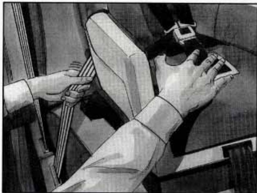
6. To tighten the belt, feed the lap belt back into the retractor while you push down on the child restraint. If you're using a forward-facing child restraint, you may find it helpful to use your knee to push down on the child restraint as you tighten the belt.
