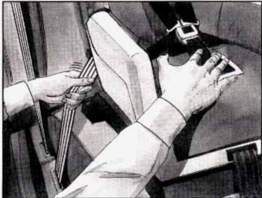
5. To tighten the belt, feed the lap belt back into the retractor while you push down on the child restraint. You may find it helpful to use your knee to push down on the child restraint as you tighten the belt.
