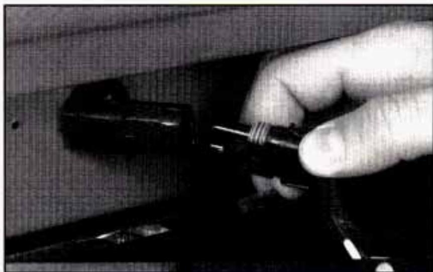
1. Remove the screws and lamp assembly.
