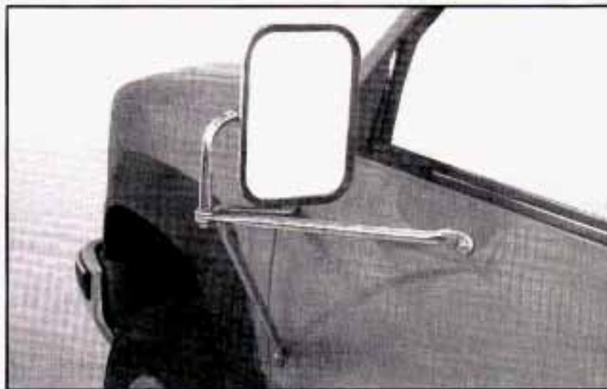
If your vehicle is equipped with the camper type mirrors, they can be adjusted so you can have a clear view of objects behind you.
