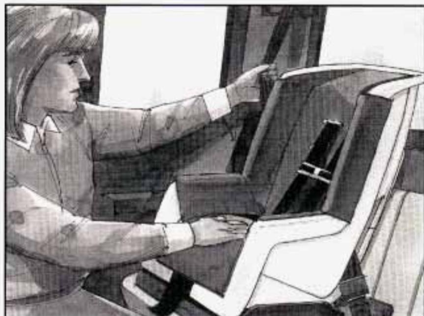
4. To tighten the belt, pull up on the shoulder belt while you push down on the child restraint. If you're using a forward-facing child restraint, you may find it helpful to use your knee to push down on the child restraint as you tighten the belt.
