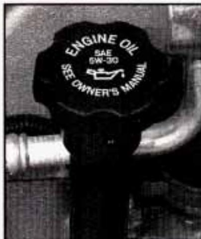
The engine oil fill cap for the "VORTEC" 4300, 5000 and 5700 engines are located on the driver's side engine valve cover.
