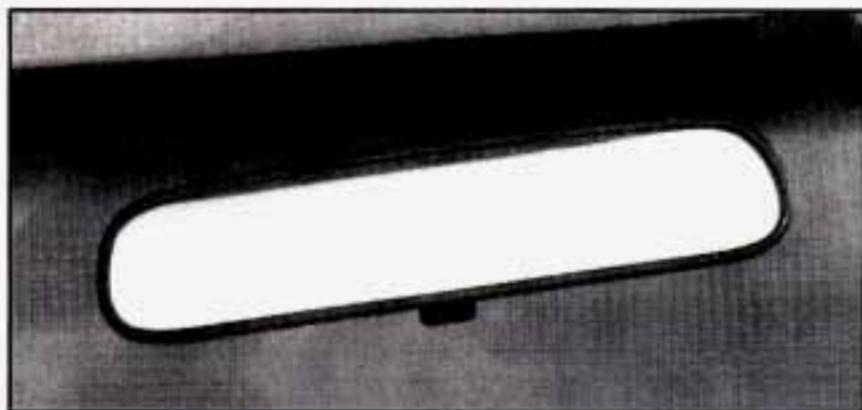
Pull the tab under the mirror rearward to reduce glare from headlamps behind you after dark. Push the tab forward for normal daytime operation.
