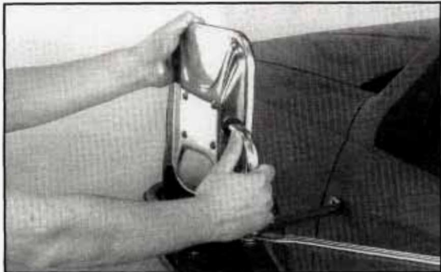
1. To adjust the mirrors when hauling a slide-in camper or towing a trailer, rotate the mirror by pushing the mirror head toward the front of the vehicle.
