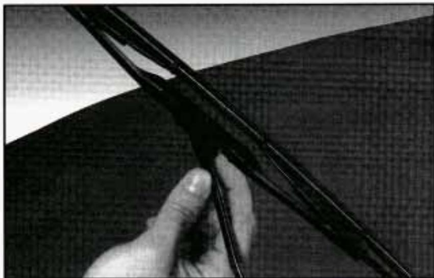
To replace the windshield wiper blade assembly:
