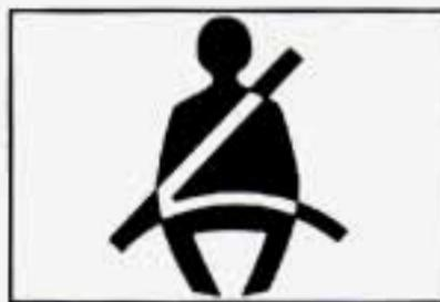
The safety belt light will also come on and stay on for about 20 seconds, then it will flash for about 55 seconds. If the driver's belt is already buckled, neither the tone nor the light will come on.
