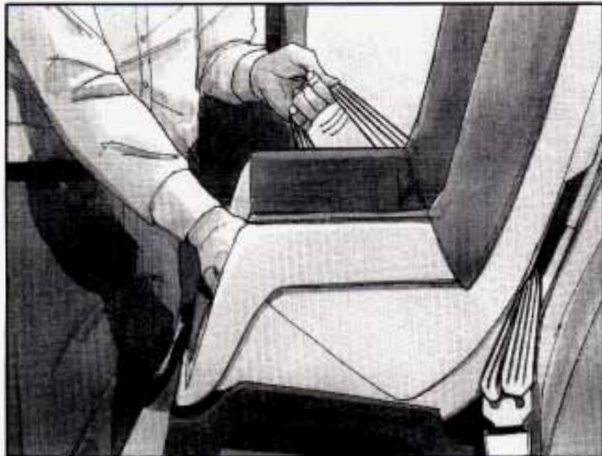
4. Pull the rest of the lap belt all the way out of the retractor to set the lock.
