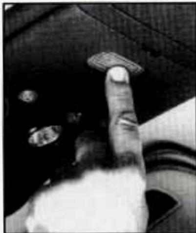
5. Now, with the compartment door closed, press the button marked **PUSH** again to make sure the garage door opener operates properly.
