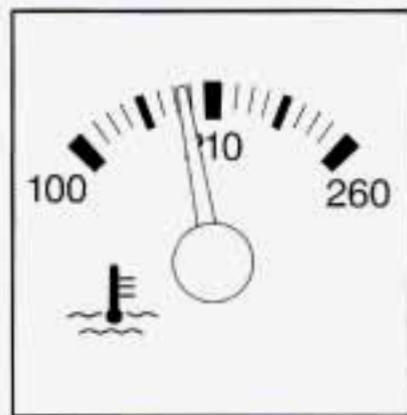
This gage shows the engine coolant temperature.
