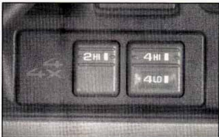
If your four-wheel-drive vehicle has the electronic transfer case, the transfer case switches are below and to the left of the climate control system.
