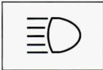
When the high beams are on, this light on the instrument panel also will be on.
