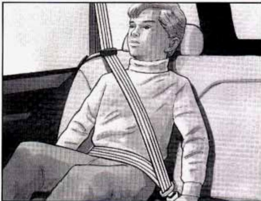
To remove and store the comfort guides, squeeze the belt edges together so that you can take them out from the guides. Slide the guide onto the storage clip.
