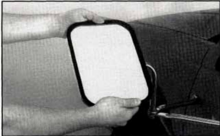
2. Rotate the mirror head, so that the mirror surface faces the rear of the vehicle.
