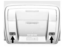
There are reading lamps in the overhead console and the headliner, if equipped. To operate, the ignition must be on or in ACC/ACCESSORY or using Retained Accessory Power (RAP).
