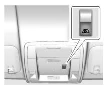
If equipped, the power sliding rear window works when the ignition has been turned on or to ACC/ ACCESSORY, or Retained Accessory Power (RAP) must be active. See Retained Accessory Power (RAP) ⇒ 260.
