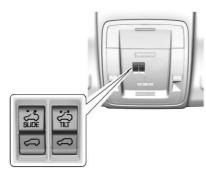
If equipped, the sunroof operates when the ignition is on or in ACC/ACCESSORY, or when Retained Accessory Power (RAP) is active. See *Retained Accessory Power* (RAP) ⇒ 260.
