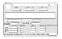
A vehicle-specific Certification/ Tire label is label is attached to the center pillar (B-pillar). The label may show the size of the vehicle's original tires and the inflation pressures needed to obtain the gross weight capacity of the vehicle. This is called Gross Vehicle Weight Rating (GVWR). The GVWR includes the weight of the vehicle, all occupants, fuel, and cargo.
