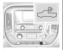
The cargo lamp provides more light in the cargo area or on the sides of the vehicle, if needed. The lights inside the pickup box and/or on the outside mirrors also turn on, if equipped.
