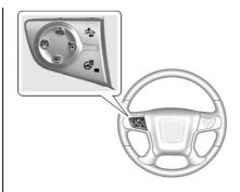
: Press to turn the system on or off. A white indicator comes on in the instrument cluster when cruise control is on and turns off when cruise control is off.
