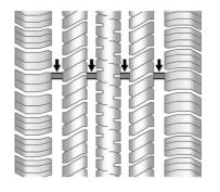
Treadwear indicators are one way to tell when it is time for new tires. Treadwear indicators appear when the tires have only 1.6 mm (1/16 in) or less of tread remaining. Some commercial truck tires may not have treadwear indicators. See *Tire Inspection* ♀ 404 and *Tire Rotation* ♀ 405 for additional information.
