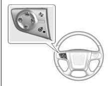
(iii): Press to turn the system on or off. A white indicator comes on in the instrument cluster when cruise control is on and turns off when cruise control is off.
