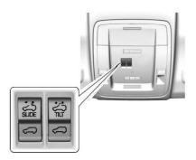
If equipped, the sunroof operates when the ignition is on or in ACC/ACCESSORY, or when Retained Accessory Power (RAP) is active. See Retained Accessory Power (RAP) ⇒ 260.
