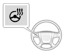
(Heated Steering Wheel, If Equipped): Press to turn it on or off. A light next to the button displays when the feature is turned on.
