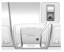
If equipped, the power sliding rear window works when the ignition has been turned on or to ACC/ ACCESSORY, or when Retained Accessory Power (RAP) is active. See Retained Accessory Power (RAP) ⇒ 260.
