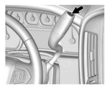
Vehicles with an automatic transmission have a Tow/Haul Mode. The Tow/Haul Mode adjusts the transmission shift pattern to reduce shift cycling. This provides
