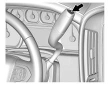
Pressing this button at the end of the shift lever turns on and off the Tow/Haul Mode.
