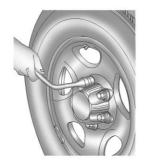
If the vehicle has wheel nut caps, loosen them by turning the wheel wrench counterclockwise. If the vehicle has a center cap with wheel nut caps, the wheel nut caps are designed to stay with the center cap after they are loosened. Remove the entire center cap.
