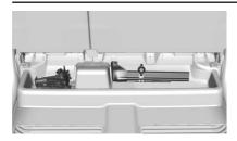
Return the jack and tools to their original location in the vehicle. See "Removing the Spare Tire and Tools."
