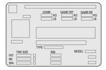
A vehicle-specific Certification/ Tire label is label is attached to the center pillar (B-pillar). The label may show the size of the vehicle's original tires and the inflation pressures needed to obtain the gross weight capacity of the vehicle. This is called Gross Vehicle Weight Rating (GVWR). The GVWR includes the weight of the vehicle, all occupants, fuel, and cargo.
