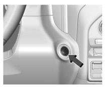
Vehicles equipped with Keyless Access have pushbutton starting.
