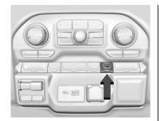
For vehicles without Driver Mode Control, press the Tow/Haul button on the center stack.
