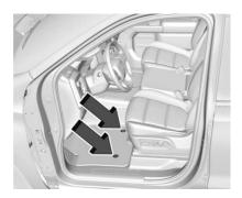
Reinstall by lining up the floor mat retainer openings over the carpet retainers and snapping into position. Make sure the floor mat is properly secured in place.
