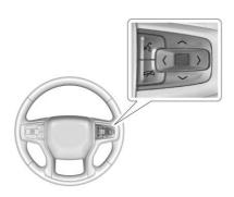
or >: Press to move left or right between the interactive display zones in the cluster. Press the thumbwheel to select.
