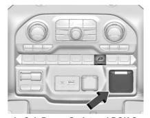
In Cab Power Outlet and DC/AC Switch
