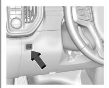
The vehicle has an Electric Parking Brake (EPB). The EPB can always be activated, even if the ignition is off. To prevent draining the battery, avoid repeated cycles of the EPB when the engine is not running.
