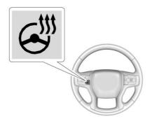
: Press to turn the heated steering wheel on or off. A light next to the button displays when the feature is turned on.
