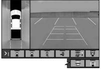
The Surround Vision (270 Degrees) can be accessed by selecting CAMERA in the infotainment display or when the vehicle is shifted into R (Reverse). To return to the previous screen sooner, press any button on the infotainment system,
