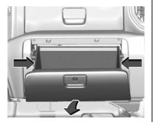
Press the sides of the glove box door inward and rotate the door downward to remove.
