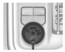
If equipped, task lighting projects light from the outside mirrors to the sides of the vehicle.
