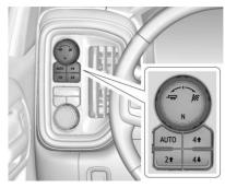
To activate modes, rotate the Drive Mode knob left or right to the desired mode.
