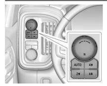
Vehicles without mode graphics on the knob will have a menu selection screen in the instrument cluster to select the desired mode. When the Drive Mode knob is rotated, the mode list will display the next available mode.
