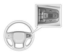
Use the right steering wheel control to open and scroll through the different items and displays.
