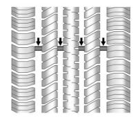
Treadwear indicators are one way to tell when it is time for new tires. Treadwear indicators appear when the tires have only 1.6 mm (1/16 in) or less of tread remaining. Some commercial truck tires may not have treadwear indicators. See *Tire Inspection* ⇒ 379 and *Tire Rotation* ⇒ 380 for additional information.
