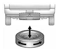
7. Make sure the tire is stored securely. Push, pull, and then try to turn the tire. If the tire moves, use the wheel wrench to tighten the cable.
