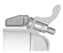
Contact your trailer service center or tire service center to have the pressure sensors installed inside the trailer tires. The technician should insert the sensor stem through the hole in the trailer wheel. When the sensor is correctly
