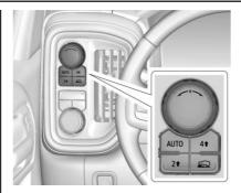
If equipped, select Terrain Mode by pressing the Terrain Mode button, below the 4 ↑ transfer case button.
