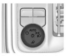
The exterior lamp control is on the instrument panel to the left of the steering wheel.
