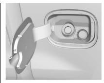
The fuel door is on the driver side of the vehicle. The vehicle has a capless refueling system and does not have a fuel cap. The filling nozzle must be fully inserted and latched prior to starting fuel flow.
