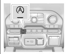
If equipped, the automatic engine Stop/Start feature can be disabled and enabled by pressing the switch with the A symbol. Auto Stop is enabled each time you start the vehicle.
