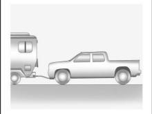
Only dinghy tow four-wheel-drive vehicles with a two-speed transfer case that have an N (Neutral) and a 4 \(\psi\) (Four-Wheel Drive Low) setting.
