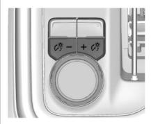
This feature controls the brightness of the steering wheel and instrument panel lights. The instrument panel illumination control is next to the exterior lamp control.
