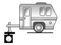
The Maximum Trailer Tongue Weight Rating for a conventional trailer hitch is shown on the Trailering Information Label. Do not exceed a maximum trailer tongue weight of 567 kg (1,250 lb) for a conventional trailer hitch.
