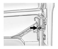
Remove the retaining wing bolt and lift it off of the mounting bracket.
