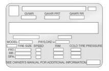
A vehicle specific Certification/ Tire label is attached to the center pillar (B-pillar). The label may show the size of the vehicle's original tires and the inflation pressures needed to obtain the gross weight capacity of the vehicle. This is called Gross Vehicle Weight Rating (GVWR). The GVWR includes the weight of the vehicle, all occupants, fuel, and cargo.
