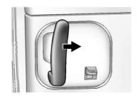
To open the sliding side door from the inside, pull the handle toward the rear of the vehicle. Then, slide the door toward the rear of the vehicle.
