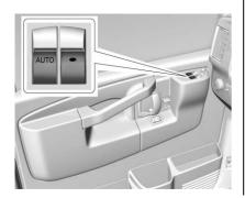
If equipped with power windows, press the switch to lower the window and pull the switch up to raise it.
