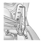
Lift the hood, release the hood prop from its retainer, and put the hood prop into the slot in the hood.
