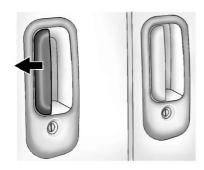
To open the sliding side door from the outside, pull the handle toward the rear of the vehicle and slide the door open.
