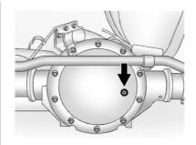
The proper level for the 2500 and 3500 Series is from 0 to 6 mm (1/4 in) below the bottom of the fill plug hole. Add only enough fluid to reach the proper level.
