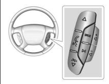
If equipped with audio steering wheel controls, some audio controls can be adjusted at the steering wheel.
