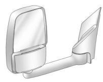
If equipped, towing mirrors can be adjusted manually for a clear view of the objects behind you.
