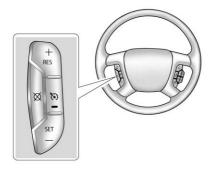
(On/Off): Press to turn cruise control on or off. The white indicator comes on in the instrument cluster when cruise control is turned on.
