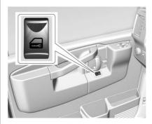
If equipped, press **a** to lock or unlock the doors.
