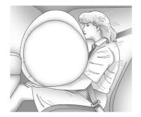
If the vehicle has a front outboard passenger frontal airbag, it is in the passenger side instrument panel.
