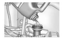
3. Fill the radiator with the proper DEX-COOL coolant mixture, up to the base of the filler neck. See Recommended Fluids and Lubricants ⇒ 302 for more information about the proper coolant mixture.
