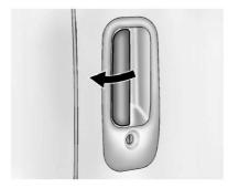
To open the front portion of a 60/40 door from the outside, pull out on the handle and open the door.
