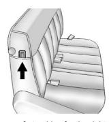
The comfort guides for the right rear outboard seating positions of three-passenger bench seats are stored in a pocket on the side of the seatback.
