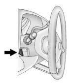
If equipped with a tilt steering wheel, the lever is on the left side of the steering column.
