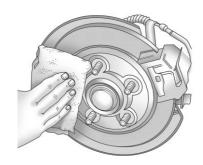
Remove any rust or dirt from the wheel bolts, mounting surfaces, and spare wheel.
