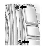
Remove the two inboard nuts from the inside of the taillamp assembly.
