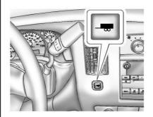
If equipped, Tow/Haul Mode adjusts the transmission shift pattern to reduce shift cycling, providing increased performance, vehicle control, and transmission cooling when towing or hauling heavy loads.
