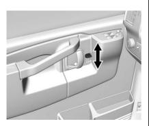
To lock the door from the inside, slide the manual lever on the door down. To unlock the door, slide the manual lever up.
