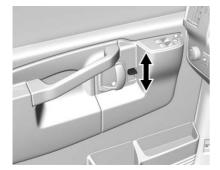
Lock and unlock the door from the outside using the key or the Remote Keyless Entry (RKE) transmitter,
