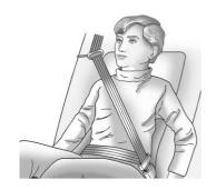
4. Buckle, position, and release the safety belt as described previously in this section. Make sure the shoulder portion of the belt is on the shoulder and not falling off of it. The belt should be close to, but not contacting, the neck. To remove and store the comfort guide, squeeze the belt edges together so that the safety belt can be removed from the guide. Slide the guide into its storage pocket on the side of the seatback.
