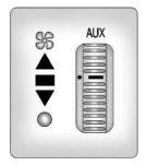
**AUX:** The thumbwheel for this system is on the instrument panel below the audio system.
