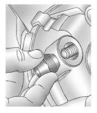
9. Put the wheel nuts back on with the rounded end of the nuts toward the wheel. Tighten each wheel nut by hand until the wheel is held against the hub
