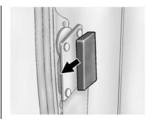
To open the driver side rear door, pull the latch release at the inside edge of the door.
