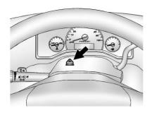
(Hazard Warning Flashers): Press this button to make the front and rear turn signal lamps flash on and off. This warns others that you are having trouble. Press again to turn the flashers off.
