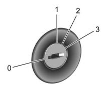
The ignition switch has four different positions.
