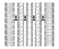
Treadwear indicators are one way to tell when it is time for new tires. Treadwear indicators appear when the tires have only 1.6 mm (1/16 in) or less of tread remaining.
