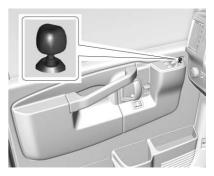
Select each mirror by turning the knob clockwise for the passenger side mirror or counterclockwise for the driver side mirror. The center position is neutral.
