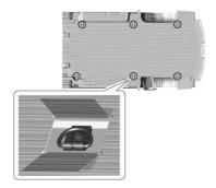
If equipped, there are six cargo tie-downs in the cargo area that can be used to secure cargo.
