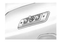
To adjust a power seat, if available, use the controls on the front of the seat:
