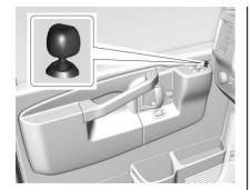
If equipped with power mirrors, select each mirror by turning the knob clockwise for the passenger side mirror or counterclockwise for the driver side mirror. Adjust the mirror angle by moving the knob in the desired direction.
