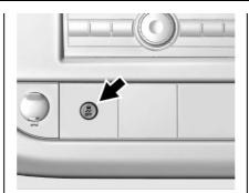
Press the StabiliTrak button on the instrument panel once to turn off the TCS. The appropriate message is displayed in the DIC. See *Ride Control System Messages* \$\dip 114.
