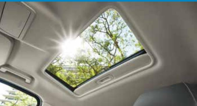
The moonroof controls are on the overhead console and have a one-touch open and close feature. To stop its movement during one-touch operation, press the control a second time.
