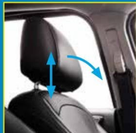
Tilt the head restraint forward for additional comfort by gently pulling the top of the head restraint. Once it is in the forward-most position, tilting it forward again releases it to the upright position.
