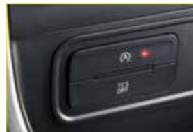
The system helps reduce fuel consumption by automatically stopping and restarting the engine when your vehicle has stopped. The engine restarts automatically when you release the brake pedal.
