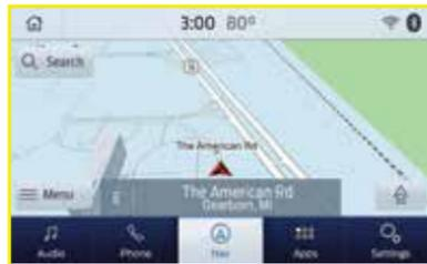
You can adjust the map to display in two-dimensional or three-dimensional mode. You can also zoom in or out on the map by using a pinching gesture. During route guidance, you will see a turn indicator, points of interest on the map, your current road and an option to mute the guidance prompts. You can press the button in the top left-hand corner of the main map to display estimated time of arrival, remaining travel time or distance to destination.
