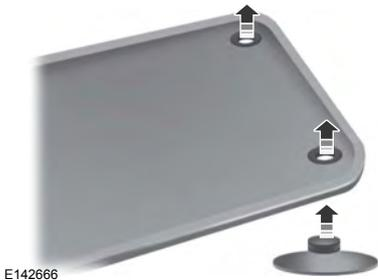
To install the floor mats, position the floor mat eyelet over the retention post and press down to lock in position.
