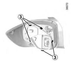
Unclip the bulb holder using tabs 3.
