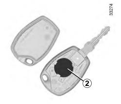
Replace battery **2** according to the direction marked on the cover.
