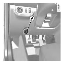
Control  $\boldsymbol{A}$  is used to adjust the height of the headlight beams according to the load.
