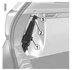
**Hubcap tool 2**Removes the wheel hubcaps.
