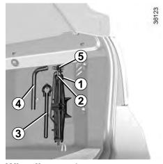
**Wheelbrace 4**Allows the wheel bolts to be locked/unlocked.
