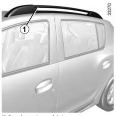
If fitted on the vehicle, you can transport luggage or additional equipment (bike racks, ski racks, etc):
