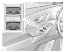
Power windows work when the ignition is on, in ACC/ACCESSORY, or when Retained Accessory Power (RAP) is active. See *Retained Accessory Power (RAP)* ⇒ 230.
