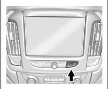
If equipped with storage behind the radio, press ☐; and hold to open. There is a charging only USB port inside. See *USB Port* ⇒ 185.
