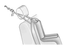
If the position you are using has an adjustable head restraint and you are using a dual tether, raise head restraint and route the tether around the head restraint posts.
