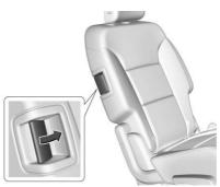
Pull the handle on the top or side of the seat forward and pull the seat forward.
