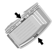
Lift up on the handles on both sides to remove the cargo management system to access the spare tire.
