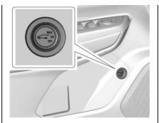
If equipped with a power liftgate, the power liftgate switch is on the driver door. The vehicle must be in P (Park).
