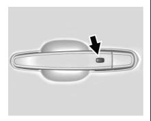
If equipped, press the button on the driver door handle when the RKE transmitter is within 1 m (3 ft) of the driver door handle. When unlocking from the driver door, the first press unlocks that door; press again within five seconds to unlock all passenger doors. See Remote Keyless Entry (RKE) System Operation ⇒ 30.
