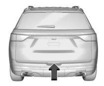
To unlock the liftgate, press on the power door lock switch or press on the Remote Keyless Entry (RKE) transmitter twice to unlock all doors. Press the touch pad on the underside of the liftgate handle and lift up. See Remote Keyless Entry (RKE) System Operation ♀ 30.
