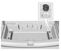
Remove the four wing nuts.
