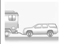
For vehicles being dinghy towed, the vehicle should be run at the beginning of each day and at each
