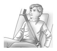
Buckle, position, and release the seat belt as described previously in this section. Make sure that the shoulder belt crosses the shoulder. The belt should be close to, but not contacting, the neck.
