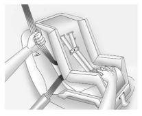
i. To tighten the belt, push down on the child restraint, pull the shoulder portion of the belt to tighten the lap portion of the belt, and feed the shoulder belt back into the retractor. When installing a forward-facing child restraint, it may be helpful to use your knee to push down on the child restraint as you tighten the belt.
