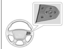
If equipped, some audio controls can be adjusted at the steering wheel.
