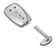
Press the button on the side of the RKE transmitter to remove the key. Never pull the key out without pressing the button. The key can be used for all locks.
