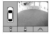
If equipped, a view of the area in front of the vehicle displays. The view displays after shifting from R (Reverse) to a forward gear, or by touching CAMERA in the infotainment display, and when the vehicle is moving forward slower than 8 km/h (5 mph).
