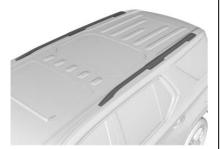
To prevent damage or loss of cargo when driving, check to make sure crossrails and cargo are securely fastened. Loading cargo on the roof
