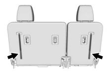
6. Pull the release strap located on the seatback.
