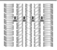
Treadwear indicators are one way to tell when it is time for new tires. Treadwear indicators appear when the tires have only 1.6 mm (1/16 in) or less of tread remaining. See *Tire Inspection* ⇒ 338 and *Tire Rotation* ⇒ 338.
