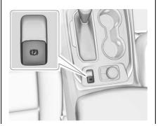
The vehicle has an Electric Parking Brake (EPB). The EPB can always be activated, even if the ignition is off. To prevent draining the battery, avoid repeated cycles of the EPB system when the engine is not runnina.
