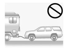
Notice: If the vehicle is towed with all four wheels on the ground, the drivetrain components could be damaged. The repairs would not be covered by the vehicle warranty. Do not tow the vehicle with all four wheels on the ground.
