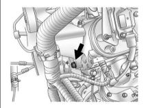
If the vehicle has a remote positive (+), it is located under a red plastic cover at the positive battery post. To uncover the remote positive (+) terminal, open the red plastic cover.
