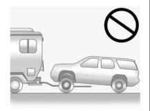
Notice: If a two-wheel-drive vehicle is towed with the rear wheels on the ground, the transmission could be damaged. The repairs would not be covered by the vehicle warranty. Never tow the vehicle with the rear wheels on the ground.
