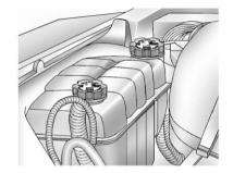
The coolant level should be at or above the FULL COLD mark with the vehicle parked on a level surface. If it is not, there might be a leak at the DMCM cooler core, DMCM pressure cap, DMCM cooler hoses, DMCM cooling pump or somewhere else in the DMCM cooling system.
