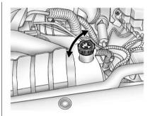
1. Park the vehicle on a level surface and turn the vehicle off. Remove the DMCM coolant surge tank pressure cap when the DMCM cooling system, including the DMCM coolant surge tank pressure cap and DMCM cooling hoses, are no longer hot. Turn the DMCM coolant surge tank pressure cap slowly counterclockwise (left) about one full turn. Wait 30 seconds.
