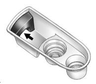
Remove the tray by pulling up on the finger depression to access the tire sealant and compressor kit.
