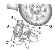
When using the tire sealant and compressor kit during cold temperatures, warm the kit in a heated environment for five minutes. This will help to inflate the tire faster.
