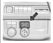
The brightness of the instrument cluster display, infotainment display and controls, steering wheel controls, and all other illuminated controls, as well as feature status indicators can be adjusted.
