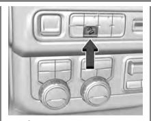
Press at to enable or disable HDC. Vehicle speed must be below 60 km/h (37 mph).
