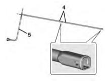
3. Assemble the jack handle extensions (4) and wheel wrench (5).
