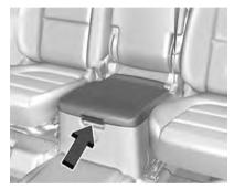
If equipped with front center seat storage, unlock with the mechanical key inside the remote key. See  $\textit{Keys} \Leftrightarrow 7$ .
