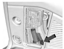
2. Turn the jack knob counterclockwise to release the jack and wheel blocks from the bracket. If equipped, remove the wheel blocks from the jack and place the wheel blocks on both sides of the tire at the opposite corner of the tire being changed. See If a Tire Goes Flat
