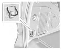
There are two cargo tie-downs in the rear cargo area. These can be used to strap cargo down and keep it from moving inside the vehicle.
