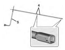
3. Assemble the jack handle extensions (4) and wheel wrench (5), as shown.
