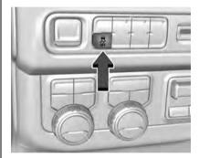
The button for TCS and StabiliTrak/ESC is on the instrument panel to the left of the steering wheel.
