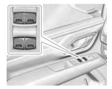
The power windows work when the ignition is on, in ACC/ACCESSORY, or when Retained Accessory Power (RAP) is active. See Retained Accessory Power (RAP) ⇒ 229.
