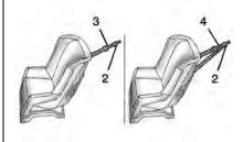
A top tether (3,4) is used to secure the top of the child restraint to the vehicle. A top tether anchor is built into the vehicle. The top tether attachment hook (2) on the child restraint connects to the top tether anchor in the vehicle in order to reduce the forward movement and rotation of the child restraint during driving or in a crash.
