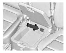
3. Place the new remote key into the backup pocket in the lower console bin.
