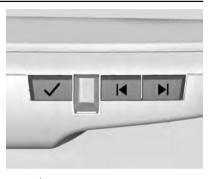
Press  $\checkmark$  to scroll through the adjustment options.
