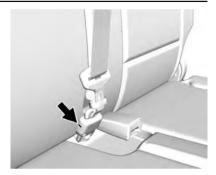
Disconnect the rear seat belt mini-latch, using a key in the slot on the mini-buckle, and let the belt retract into the headliner.
