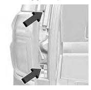
4. Remove the two rear lamp assembly screws.
