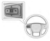
🟵 : Press to turn cruise control on or off. A white indicator comes on or off in the instrument cluster. **+RES**: If there is a set speed in memory, press the control up briefly to resume to that speed or press and hold to accelerate. If cruise control is already engaged, use to increase vehicle speed.
