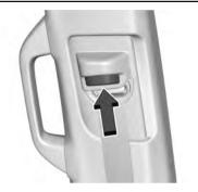
Push the release button to move the height adjuster to the desired position.
