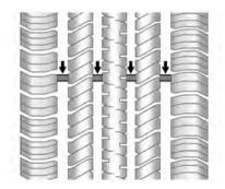
Treadwear indicators are one way to tell when it is time for new tires. Treadwear indicators appear when the tires have only 1.6 mm (1/16 in) or less of tread remaining. See *Tire Inspection* \$351 and *Tire Rotation* \$352 for additional information.
