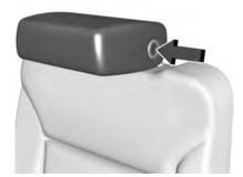
The head restraint will fold forward automatically.
