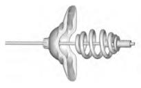
Tilt the retainer and pull it and the cable and spring through the center of the wheel.
