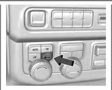
If equipped, select Terrain Mode by pressing the below the 4 1 transfer case button.
