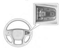
or > : Press to move left or right between the interactive display zones in the cluster. Press the thumbwheel to select.  $\wedge$  or  $\vee$ : Use the thumbwheel to scroll up or down in a list. Press the thumbwheel to open a menu or select a menu item. Press and hold to reset values on certain screens.
