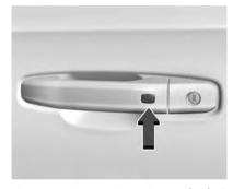
The remote key must be within 1 m (3 ft) of the trunk or door being opened or locked. Press the button on the door handle to open. See "Keyless Access Operation" in Remote Keyless Entry (RKE) System Operation ⇒ 8.
