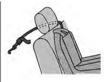
If the position you are using has a fixed headrest or head restraint and you are using a single tether, route the tether around the inboard side of the headrest or head restraint.
