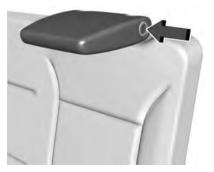
The head restraint will fold forward automatically.
