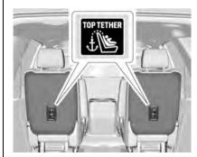
For models with bucket second row seating, the top tether anchors are on the rear of the seatback for each seating position in the second row. Be sure to use an anchor located directly behind the seating position where the child restraint will be placed.
