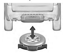
Make sure the tire is stored securely. Push, pull, and then try to turn the tire. If the tire moves, use the wheel wrench to tighten the cable.
