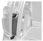
Remove the lower taillamp closeout cover from the taillamp assembly by pulling rearward from the top and bottom to disengage the clips.
