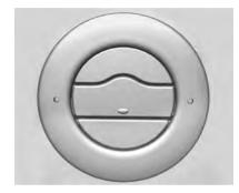
Press on the center vane rear edge to open the round outlet. Use the center vane to rotate the outlet and change the direction of the airflow. Press on the center vane leading edge to shut off the air flow.
