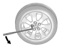
Turn the wheel wrench counterclockwise to loosen the wheel nuts. Do not remove them yet.
