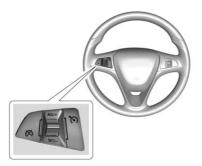
revise : Press to turn the cruise control system on and off. A white indicator comes on in the instrument cluster when cruise is turned on. **RES/+**: If there is a set speed in memory, move the thumbwheel up briefly to resume to that speed or hold upward to accelerate. If cruise control is already active, use to increase vehicle speed.
