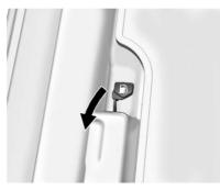
The tethered fuel cap is behind a hinged fuel door on the passenger side of the vehicle. To open the fuel filler door, lift the fuel door release lever. The lever is on the floor, on the left front side of the driver seat. The fuel door is unlocked when the vehicle is unlocked. Locking the vehicle locks the fuel door.
