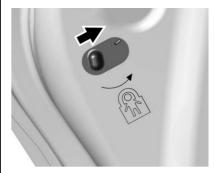
The vehicle has rear door safety locks on each rear door that prevent passengers from opening the rear doors from the inside.
