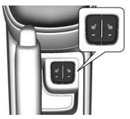
If available, the buttons are below the climate control system. To operate, the engine must be running.
