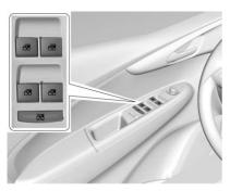
The driver power window switches control all the windows. The passenger switch controls only that window.
