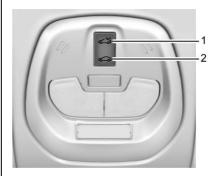
**Vent/Open :** Press and hold the switch (1) to vent. Press and hold the switch (1) again to open the sunroof. Release the switch to stop
