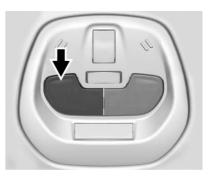
The reading lamps are in the overhead console.
