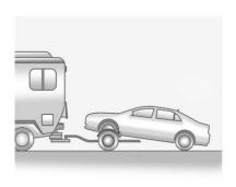
To tow the vehicle with the two rear wheels on the ground and the front wheels on a dolly:
