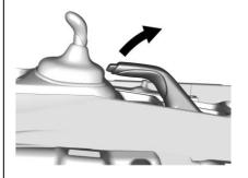
To set the parking brake, hold the brake pedal down and pull up on the parking brake lever. If the ignition is on, the brake system warning light will come on. See *Brake System Warning Light*  $\Rightarrow$  103.
