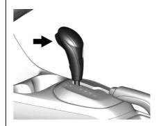
**P** : This position locks the front wheels. Select P (Park) only when the vehicle is stationary and the parking brake is applied.
