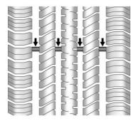
Treadwear indicators are one way to tell when it is time for new tires. Treadwear indicators appear when the tires have only 1.6 mm (1/16 in) or less of tread remaining. See *Tire Inspection*  $\Rightarrow$  251 and *Tire Rotation*  $\Rightarrow$  251.
