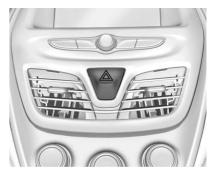
The hazard warning flasher button is on the center stack.
