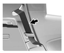
1. Move the safety belt out of the way by putting the safety belts into the belt guide on the trim.
