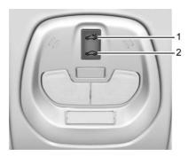
**Vent/Open :** Press and hold the switch (1) to vent. Press and hold the switch (1) again to open the sunroof. Release the switch to stop movement. The sunshade automatically opens with the sunroof, but must be closed manually.
