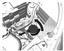
2. Remove the washer funnel by turning it counterclockwise.
