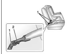
Lower anchors (1) are metal bars built into the vehicle. There are two lower anchors for each LATCH seating position that will accommodate a child restraint with lower attachments (2).
