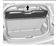
To remove, pull the cargo cover upward.
