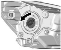
3. Remove the headlamp bulb socket.
