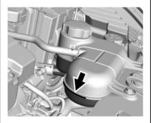
If coolant is visible but the coolant level is not at or above the mark pointed to, add a 50/50 mixture of clean drinkable water and DEX-COOL coolant.
