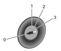
The ignition switch has four different positions.
