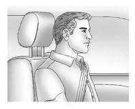
Adjust the head restraint so that the top of the restraint is at the same height as the top of the occupant's head. This position reduces the chances of a neck injury in a crash.
