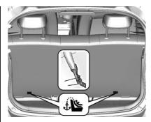
The top tether anchors are located on the rear seatbacks. Be sure to use an anchor on the same side of the vehicle as the seating position where the child restraint will be placed.
