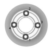
Tighten the wheel nuts firmly with the wheel wrench in a crisscross sequence, as shown.
