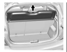
To remove, pull the cargo cover upward.
