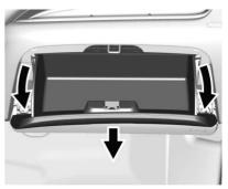
Open the glove box completely and loosen the bolts on the outboard side. 2. Push in both sides of the glove box and pull to remove.
