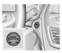
The vehicle may be equipped with an electronic keyless ignition with pushbutton start. Pressing the button cycles it through three modes: ACC/ACCESSORY, ON/RUN/START, and Stopping the Engine/OFF.
