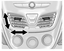
Move the slats to change the direction of the airflow. The center air vent does not close completely.
