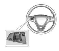
cellist: Press to turn the cruise control system on and off. A white indicator comes on in the instrument cluster when cruise is turned on.
