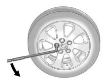
Turn the wheel wrench counterclockwise to loosen the wheel nuts. Do not remove them yet.
