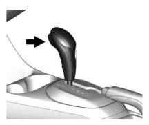
**P**: This position locks the front wheels. Select P (Park) only when the vehicle is stationary and the parking brake is applied.
