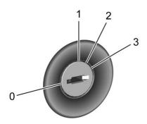
The ignition switch has four different positions.
