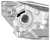
3. Remove the headlamp bulb socket.
