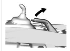
To set the parking brake, hold the brake pedal down and pull up on the parking brake lever. If the ignition is on, the brake system warning light will come on. See *Brake System Warning Light* \$\phi\$ 105.
