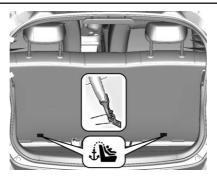
The top tether anchors are located on the rear seatbacks. Be sure to use an anchor located directly behind the seating position where the child restraint will be placed.
