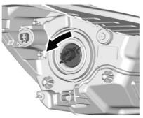
3. Remove the headlamp bulb socket.
