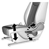
If available, move the lever up or down to manually raise or lower the seat.
