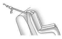
If you are using a single tether in an outboard seating position and the head restraint has been removed, route the tether over the seatback.
