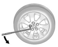
3. Turn the wheel wrench counterclockwise to loosen the wheel nuts. Do not remove them yet.
