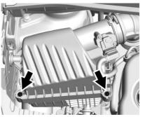
1. Remove the two screws and lift the cover out of the assembly.
