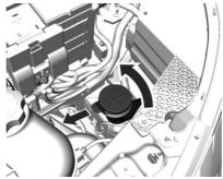
2. Remove the washer funnel by turning it counterclockwise and pulling it straight out.
