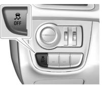
The button for TCS and StabiliTrak/ESC is on the lower instrument panel to the left of the steering wheel.
