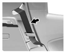
1. Move the seat belt out of the way by putting the seat belts into the belt guide on the trim.
