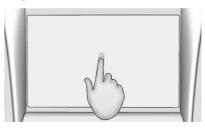
Nudge is used to move items a short distance on a list. To nudge, hold and move the selected item up or down to a new location.
