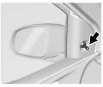
If equipped, controls for the outside manual mirrors are next to each mirror. Adjust to see a little of the side of the vehicle.
