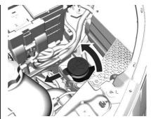
2. For the driver side bulb, remove the washer funnel by turning it counterclockwise and pulling it straight out.
