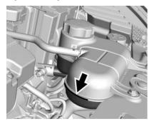
Check to see if coolant is visible in the coolant surge tank. If the coolant inside the coolant surge tank is boiling, do not do anything else until it cools down. See *Engine Overheating* ⇔ 173.
