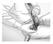
If the webbing locks in the latch plate before it reaches the buckle, tilt the latch plate to flat to unlock.
