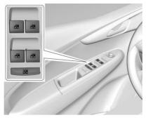
Power windows work when the ignition is on, in ACC/ACCESSORY, or when Retained Accessory Power (RAP) is active. See Retained Accessory Power (RAP)  $\Rightarrow$  140.
