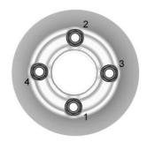
14. Tighten the wheel nuts firmly with the wheel wrench in a crisscross sequence, as shown.
