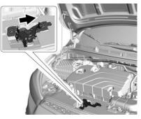
2. Go to the front of the vehicle and locate the secondary release lever under the front center of the hood. Push the secondary hood release lever to the right to release.
