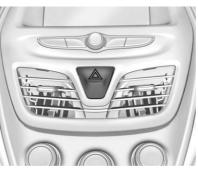
The hazard warning flasher button is on the center stack.
