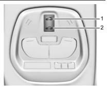
Express-Vent/Open : Press and release (1) to express-vent. Press and release (1) again to express-open the sunroof. Press the switch again to stop movement. The sunshade automatically opens with the sunroof, but must be closed manually.
