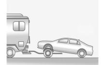
To tow the vehicle with the two rear wheels on the ground and the front wheels on a dolly:
