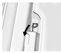
To open the fuel door, lift the fuel door release lever. The lever is on the floor, on the left front side of the driver seat.
