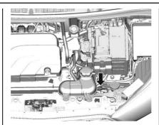
2. Open the hood and unwrap the electrical cord. The cord is in the driver side of the engine compartment, near the engine coolant surge tank. It is shipped from the factory with a tie holding it in place. Use care in removing the tie so that the cord is not damaged.
