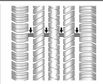
Treadwear indicators are one way to tell when it is time for new tires. Treadwear indicators appear when the tires have only 1.6 mm (1/16 in) or less of tread remaining. See *Tire Inspection*  $\Rightarrow$  *199* and *Tire Rotation*  $\Rightarrow$  *200* for additional information.
