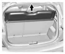
To remove, pull the cargo cover upward.
