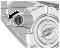
2. Remove the sidemarker lamp bulb socket from the headlamp assembly by turning counterclockwise.
