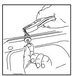
2. While continuing to pull downward on the push-pin, squeeze and rotate the expandable end of the push-pin with your fingers or a pair of pliers until it releases from the retainer.
