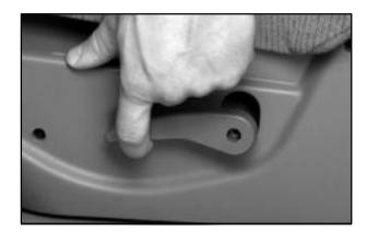
To adjust the front seatback, lift the lever upward. Release the lever to lock the seatback where you want it. Lift the lever again upward and the seatback will go to an upright position.
