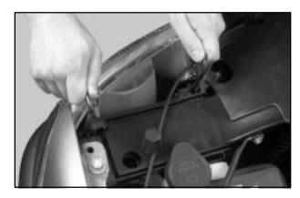
1. Remove the two pins on the top of the headlamp assembly. To remove the pins, turn the outer pin outward and pull it straight up. To remove the inner pin, turn it inward and pull it straight up.
