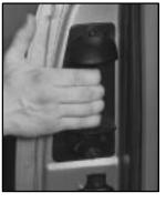
To open the rear access door from the outside, first open the passenger's side front door. Then, use the handle located on the front edge of the access door to open it.
