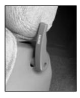
To operate the seat, pull forward on the top of this lever and tilt the seatback forward toward the front of the vehicle.
