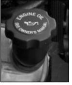
The engine oil fill cap for the VORTEC 4300 V6 engine is located on the driver's side engine valve cover.
