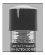
The air cleaner assembly has an indicator that lets you know when the air filter is dirty and needs to be serviced. The indicator is located on the air cleaner cover.
