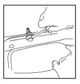
1. Insert the blade portion of a flat-blade screwdriver into the push-pin slot and pull downward until the push-pin snaps loose.
