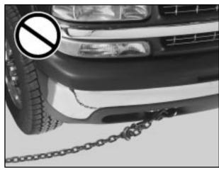
Your vehicle may be equipped with recovery hooks. The recovery hooks are provided at the front of your vehicle. You may need to use them if you're stuck off-road and need to be pulled to some place where you can continue driving.
