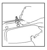
1. Line up each push-pin with it's intended retainer and push the washer portion of the push-pin towards the retainer until it locks into place.
