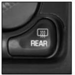
To turn on the rear window defogger, press this button next to the fan control knob.
