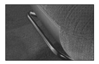
If your vehicle has a manual bucket or split bench seat, you can adjust it with this lever located at the front of the seat.
