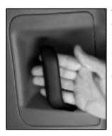
To open the rear access door from the inside, the passenger's side front door must be opened first. Then, use the handle located on the inside of the rear access door to open it.
