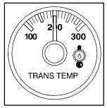
If your vehicle has a heavy duty automatic transmission, you will have a transmission temperature gage.
