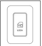
If your vehicle has this power door lock switch, press the bottom of the switch on either front door to lock all the doors at once.
