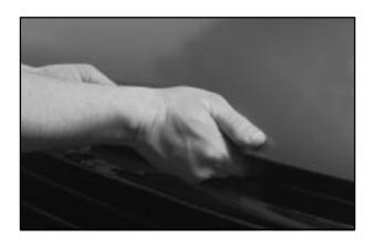
Then go to the front of the vehicle and pull up on the secondary hood release, located just to the passenger's side of the center of the grill.
