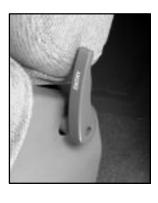
To fold a front seatback forward, pull this lever forward and fold the seatback forward.
