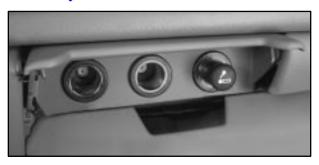
Two auxiliary power outlets are located near the cigarette lighter. Use these outlets to power mobile telephones or other devices designed to operate with vehicle electrical systems.
