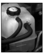
The coolant surge tank is located on the passenger's side of the engine compartment.
