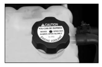
The coolant surge tank pressure cap must be fully installed on the coolant surge tank.
