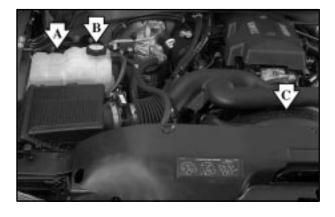
The coolant level should be at or above the FILL COLD mark.
