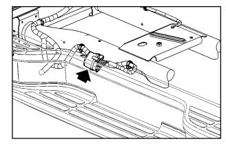
The trailer wiring harness with a seven-pin connector and separate Center High-Mounted Stoplamp (CHMSL) connector are located at the rear of the vehicle and are tied to the vehicle's frame.\* The harness connector can be plugged into a seven-pin universal heavy-duty trailer connector available through your GM dealer.
