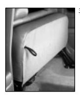
3. Push and pull on the seat to make sure the seat is secure.
