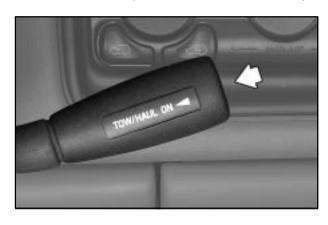
Your vehicle is equipped with a tow/haul mode. The selector switch is located on the end of the column shift lever. You can use this feature to assist when towing or hauling a heavy load. See "Tow/Haul Mode" in the Index for more information.
