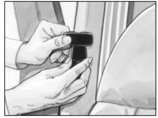
Remove the guide from its storage clip on the interior body.
