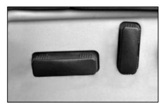
**Horizontal Control:** If your vehicle has a power seat, you can adjust it with this control located at the outside edge of the seat.
