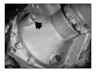
If the level is below the bottom of the filler plug hole, you may need to add some lubricant.
