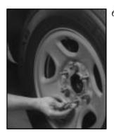
6. After mounting the spare, replace the wheel nuts with the rounded end of the nuts toward the wheel. Tighten each wheel nut by hand using the wheel wrench until the wheel is held against the hub.
