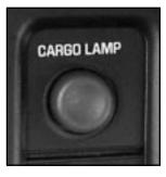
Press the button to turn the cargo lamp on. Press the button again to turn it off.
