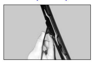
Windshield wiper blades should be inspected at least twice a year for wear and cracking. See "Wiper Blade Check" in Section 7 of this manual under Part B "Owner Checks and Services" for more information.
