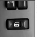
If your vehicle has this power door lock switch, press the raised side of the switch, marked "L" on either front door to lock all the doors at once.
