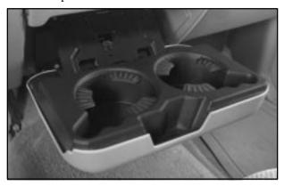
To use the cupholder, pull the cupholder out of the instrument panel.
