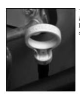
The engine oil dipstick has a yellow ring handle and is located on the passenger's side of the engine.
