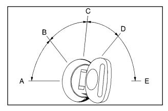
ACCESSORY (A): ACCESSORY lets you use things like the radio, power windows and the windshield wipers when the engine is off. Push in the key and turn it toward you. Your steering wheel will remain locked, just as it was before you inserted the key.
