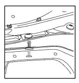
3. Pull the push-pins and lower air dam assembly away from the retainers until the lower air dam is free.
