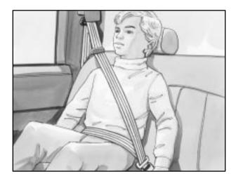
Buckle, position and release the safety belt as described in "Rear Seat Outside Passenger Positions (Extended Cab)" earlier in this section. Make sure that the shoulder belt crosses the shoulder.
