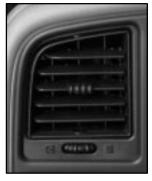
Your vehicle has air outlets in the center and on the sides of your instrument panel.
