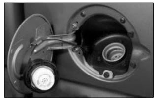
While refueling, hang the filler cap by the tether using the hook located on the inside of the filler door.
