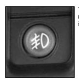
The fog lamp switch is on the left side of your instrument panel.
