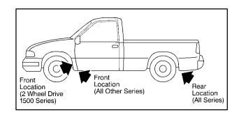
Position the jack under the vehicle. If the flat tire is on the front of the vehicle (2-Wheel Drive 1500 Series vehicles), position the jack under the bracket attached to the vehicle's frame, behind the flat tire. If the flat tire is on the front of the vehicle (All other models), position the jack on the frame behind the flat tire.
