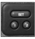
The memory function controls the driver's seat cushion and recliner positions.
