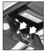
4. Add one peg at a time until the PUSH button on the compartment door will operate the garage door opener, with the compartment door closed, when you press the button marked PUSH.
