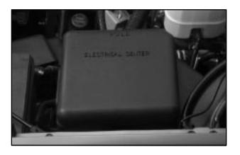
The underhood electrical center is located on the driver's side of the engine compartment near the battery. Lift the cover for access to the fuse/relay block.
