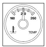
This gage shows the engine coolant temperature.
