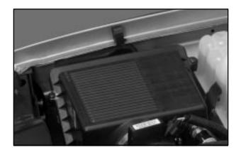
Your air cleaner is located in the passenger's side front corner of the engine compartment.
