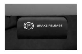
To release the parking brake, hold the regular brake pedal down. Pull the bottom edge of the lever, located just above the parking brake pedal, marked BRAKE RELEASE, to release the parking brake.
