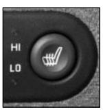
If your vehicle has heated front seats, the ignition must be in RUN for them to operate.
