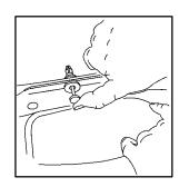
2. Push the flat end of the push-pin towards the retainer until it locks into place, making sure each is secure.
