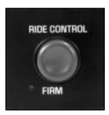
This button is on the center of the instrument panel near the radio. Press it to activate the selectable ride setting as desired. An indicator light near the button will illuminate whenever the system is active.
