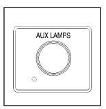
This switch includes wiring provisions for a dealer or a qualified service center to install an auxiliary roof lamp. This switch is located on the center of the instrument panel near the comfort controls.
