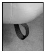
1. Pull forward on the release strap under the rear seat cushion, on the passenger's side.
