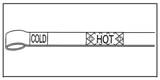
Safe operating level is within the HOT cross hatch band on the dipstick. If the fluid level is not within the HOT band, and the transmission temperature is between 71°C and 93°C (160°F and 200°F), add
