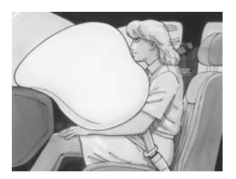
The right front passenger airbag is in the instrument panel on the passenger's side.
