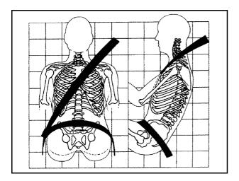
Sit up straight and always keep your feet on the floor in front of you. The lap part of the belt should be worn low and snug on the hips, just touching the thighs. In a crash, this applies force to the strong pelvic bones and you would be less likely to slide under the lap belt.
