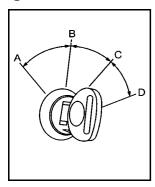
The ignition switch has four different positions.
