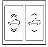
There are two sunroof switches located in the overhead console above the rearview mirror. **Vent:** From the closed position, press the rear of the passenger side switch to vent the sunroof.
