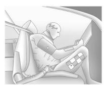
When riding in a vehicle, you travel as fast as the vehicle does. If the vehicle stops suddenly, you keep going until something stops you. It could be the windshield, the instrument panel, or the safety belts!
