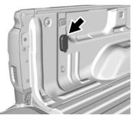
For vehicles with the 5th wheel/ gooseneck trailer package, the harness connector is mounted on the inside of the pickup bed behind the rear wheel.
