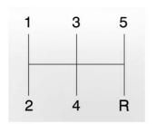
If equipped with a manual transmission, this is the shift pattern.
