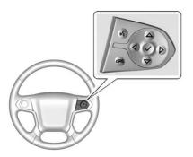
If equipped, some audio controls can be adjusted at the steering wheel. Information
