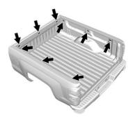
The vehicle may be equipped with cargo tie-downs.
