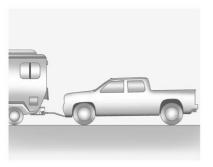
Only dinghy tow four-wheel-drive vehicles with a two-speed transfer case that have an N (Neutral) and a Four-Wheel Drive Low (4 ( $\downarrow$ ) setting.
