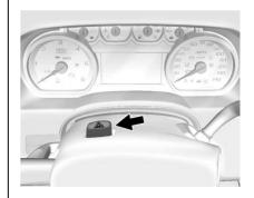
(Hazard Warning Flashers) : Press this button to make the front and rear turn signal lamps flash on and off. Press again to turn the flashers off.
