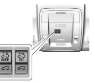
If equipped, the sunroof only operates when the ignition is in ACC/ACCESSORY or ON/RUN, or when Retained Accessory Power (RAP) is active. See *Retained Accessory Power* (*RAP*) ⇔ 284.
