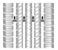
Treadwear indicators are one way to tell when it is time for new tires. Treadwear indicators appear when the tires have only 1.6 mm (1/16 in) or less of tread remaining. Some commercial truck tires may not have treadwear indicators. See *Tire Inspection* ⇔ 422 and *Tire Rotation* ⇔ 422 for additional information.
