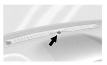
The solar sensor, located in the defrost grille in the middle of the instrument panel, monitors the solar heat. Do not cover the solar sensor or the system will not work properly.
