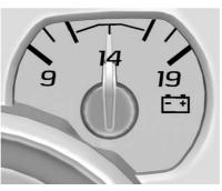
When the ignition is on, this gauge indicates the battery voltage.
