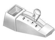
This transfer case shift lever is on the floor to the right of the driver.
