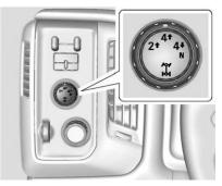
Use the transfer case knob, next to the steering wheel, to shift into and out of four-wheel drive for extra traction.
