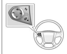
(On/Off) : Press to turn the system on or off. The indicator light is white when cruise control is on and turns off when cruise control is off.
