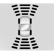
The instrument cluster may have a parking assist display with bars that show "distance to object" and object location information for the Parking Assist system. As the object gets closer, more bars light up and the bars change color from yellow to amber to red.
