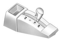
Move the lever to shift into and out of four-wheel drive.
