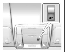
If equipped, the power sliding rear window works when the ignition has been turned to ACC/ACCESSORY or ON/RUN, or when Retained Accessory Power (RAP) is active. See Retained Accessory Power (RAP) ⇔ 284.
