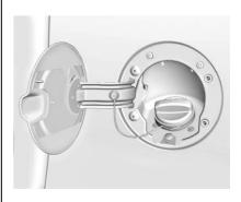
The fuel cap is behind a hinged fuel door on the driver side of the vehicle. Vehicles that have a FlexFuel badge and a yellow fuel cap can use either unleaded gasoline or ethanol fuel containing up to 85% ethanol (E85). See *E85* or *FlexFuel*  $\Rightarrow$  324.
