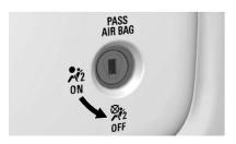
To turn off the front outboard passenger frontal airbag, insert the ignition key into the switch, push in, and move the switch to the off position.
