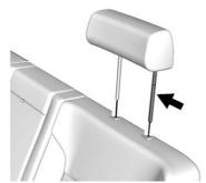
Insert the headrest posts into the holes in the top of the seatback with the longer chrome plated post toward the driver side of the vehicle. 2. Push the headrest all the way down until it contacts the top of the seatback.
