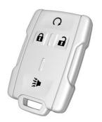
**1**: Press to unlock the driver door. Press **1** again within three seconds to unlock all remaining doors and the tailgate.
