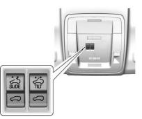
If equipped, the sunroof operates when the ignition is in ACC/ ACCESSORY or ON/RUN, or when Retained Accessory Power (RAP) is active. See *Retained Accessory Power (RAP)* ⇔ 284.
