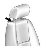
The height of the head restraint can be adjusted. Pull the head restraint up to raise it. Try to move the head restraint to make sure that it is locked in place.
