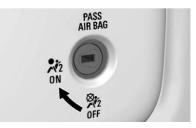
To turn the front outboard passenger frontal airbag on again, insert the ignition key into the switch, push in, and move the switch to the on position.
