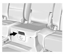
If equipped with front seat floor console storage, unlock with the ignition key, press the button, and lift to open.
