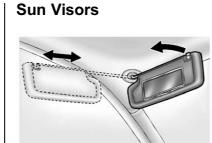
Pull the sun visor down to block glare. Detach the sun visor from the center mount to pivot to the side window or, if equipped, extend along the rod. Sunroof
