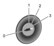
The ignition switch has four different positions.
