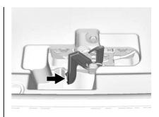
2. Go to the front of the vehicle to find the secondary hood release. The handle is under the front edge of the hood near the center. Push the handle to the right and at the same time raise the hood.
