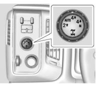
Use the transfer case knob next to the steering wheel to shift into and out of four-wheel drive.
