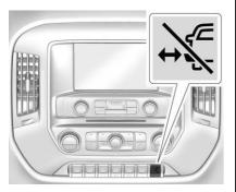
The power assist steps can be extended and extended to the tire by pressing . When extending the steps with , the kick switch is disabled.
