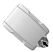
1. Separate and remove the back cover of the transmitter with a flat, thin object, such as a coin.
