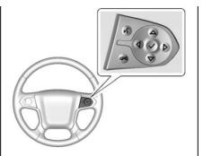
$\triangle$  or  $\nabla$ : Press to move up or down in a list. In the main view, you can press up and down to move between different info app pages.
