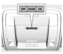
There are dome lamps in the overhead console and the headliner, if equipped.
