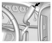
Vehicles with an automatic transmission have a Tow/Haul Mode. The Tow/Haul Mode adjusts the transmission shift pattern to reduce shift cycling. This provides increased performance, vehicle control, and enhanced transmission and engine cooling when driving down steep hills or mountain grades, towing, or hauling heavy loads.
