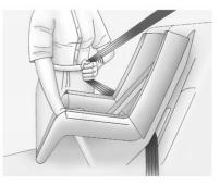
5. Pull the shoulder belt all the way out of the retractor to set the lock. When the retractor lock is set, the belt can be tightened but not pulled out of the retractor.
