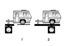
Trailer tongue weight (1) should be 10-15% and fifth-wheel or gooseneck kingpin weight should be 15-25% of the loaded trailer weight (2) up to the maximums for vehicle series and hitch type.
