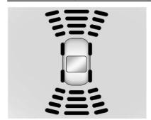
The instrument cluster may have a Park Assist display with bars that show "distance to object" and object location information for the Park Assist system. As the object gets closer, more bars light up and the bars change color from yellow to amber to red.
