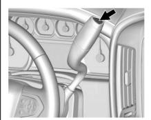
The Tow/Haul Mode adjusts the transmission shift pattern to reduce shift cycling. This provides increased performance, vehicle control, and enhanced transmission
