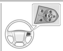
$\triangle$  or  $\nabla$ : Press to move up or down in a list. In the main view, press up and down to move between different info app pages.
