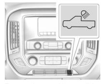
The cargo lamp provides more light in the cargo area or on the sides of the vehicle, if needed. The lamps inside the pickup box and/or on the outside mirrors also turn on, if equipped.
