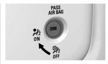
To turn the front outboard passenger frontal airbag on again, insert the ignition key into the airbag on-off switch, push in, and move the switch to the ON position.
