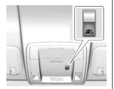
If equipped, the power sliding rear window works when the ignition has been turned on or to ACC/ ACCESSORY, or when Retained Accessory Power (RAP) is active. See Retained Accessory Power (RAP) ⇒ 251.
