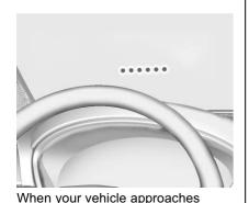
another detected vehicle too rapidly, the red FCA display will flash on the windshield. Also, eight rapid high-pitched beeps will sound from the front, or both sides of the Safety Alert Seat will pulse five times. When this Collision Alert occurs, the brake system may prepare for driver braking to occur more rapidly which can cause a brief, mild deceleration. Continue to apply the brake pedal as needed. Cruise control may be disengaged when the Collision Alert occurs.
