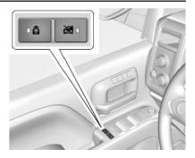
Press to activate the safety locks on the rear doors. The indicator light comes on when activated. Press again to deactivate. The vehicle must be on, in ACC/ACCESSORY, or in Retained Accessory Power (RAP). See Retained Accessory Power (RAP) ⇒ 251.
