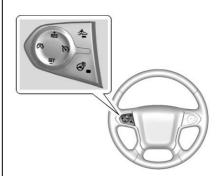
: Press to turn the system on or off. The indicator light is white when cruise control is on and turns off when cruise control is off.
