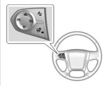
Fress to turn the system on or off. The indicator light is white when cruise control is on and turns off when cruise control is off.
