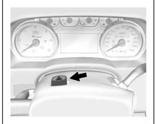
: Press this button to make the front and rear turn signal lamps flash on and off. Press again to turn the flashers off.
