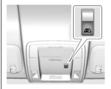
If equipped, the power sliding rear window works when the ignition has been turned on or to ACC/ ACCESSORY, or Retained Accessory Power (RAP) must be active. See *Retained Accessory Power (RAP)*
