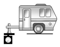
The Maximum Trailer Tongue Weight Rating for a conventional trailer hitch or a fifth wheel/gooseneck hitch is shown on the Trailering Information Label.
