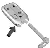
Press the button on the RKE transmitter to remove the key. Never pull the key out without pressing the button.
