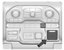
In Cab Power Outlet and DC/AC Switch
