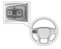
S: Press to turn cruise control on or off. A white indicator comes on or off in the instrument cluster.
