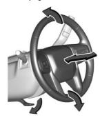
To adjust the tilt and telescoping steering wheel, if equipped:
