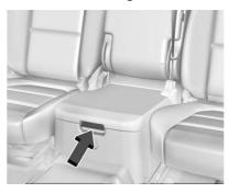
If equipped with front center seat storage, unlock with the ignition key, press the latch, and lift to open.
