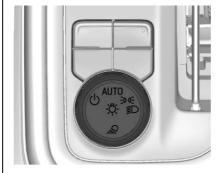
The exterior lamp control is on the instrument panel to the left of the steering wheel.
