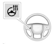
: If equipped, press to turn it on or off. A light next to the button displays when the feature is turned on.
