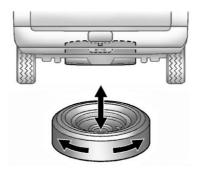
Make sure the tire is stored securely.Push, pull, and then try to turn the tire.If the tire moves, use the wheel wrench to tighten the cable.
