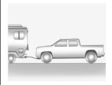
Only dinghy tow four-wheel-drive vehicles with a two-speed transfer case that have an N (Neutral) and a  $4 \downarrow$  (Four-Wheel Drive Low) setting.
