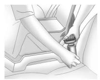
Push the latch plate into the buckle until it clicks. Position the release button on the buckle, away from the child restraint, so that the seat belt could be quickly unbuckled if necessary.
