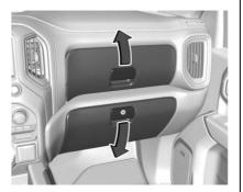
To access the upper glove box, pull up on the handle.
