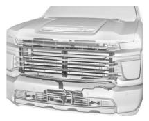
The vehicle may have a shutter system designed to help improve fuel economy. Keep the shutter system clear of debris, snow and ice. If the check engine light is activated, please check to see if the shutter system is clear of debris, snow or ice.
