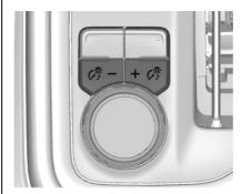
This feature adjusts the brightness of all illuminated controls. The instrument panel illumination control is next to the exterior lamp control.
