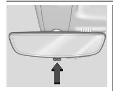
Pull the tab to turn on the display. Push the tab to turn it off. When off the mirror is automatic dimming. Adjust the mirror for a clear view of the area behind the vehicle while the display is off.
