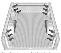
This vehicle is equipped with 12 fixed cargo tie-downs.
