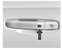
If equipped, the remote key must be within 1 m (3 ft) of the tailgate or door being opened or locked. Press the button on the door handle to open. See "Keyless Access Operation" in Remote Keyless Entry (RKE) System Operation (Key Access) \$\Displays 10\$ or Remote Keyless Entry (RKE) System Operation (Keyless Access) \$\Displays 13.
