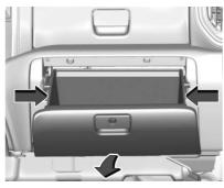
Press the sides of the glove box door inward and rotate the door downward to remove.
