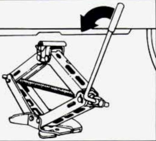
11. Lower the vehicle by turning the wheel wrench to the left. Lower the jack completely.
