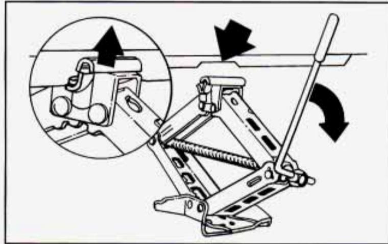
6. Raise the vehicle by turning the wheel wrench to the right. Raise the vehicle far enough off the ground so there is enough room for the spare tire to fit.
