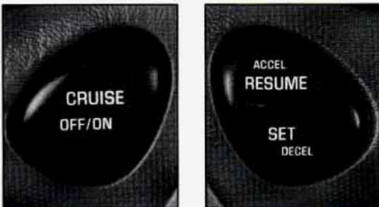
With cruise control, you can maintain a speed of about 25 mph (40 km/h) or more without keeping your foot on the accelerator. This can really help on long trips. Cruise control does not work at speeds below 25 mph (40 km/h).
