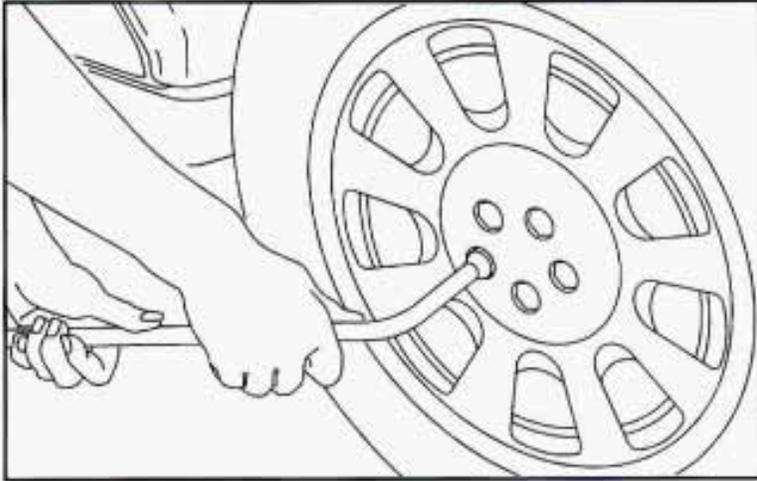
4. Then use the wheel wrench to *loosen* all the wheel nuts. Don't remove them yet.
