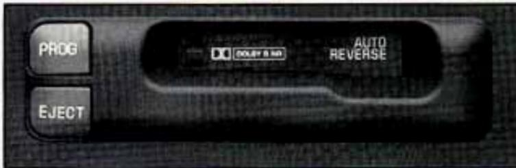
With this option, the remote single cassette player is mounted near the bottom of the instrument panel, above the ashtray and below the HVAC controls.
