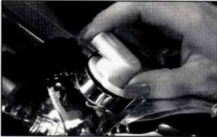
5. For the turn signal bulb, press the tab on the white bulb socket and twist it less than one-quarter of a turn to the left.
