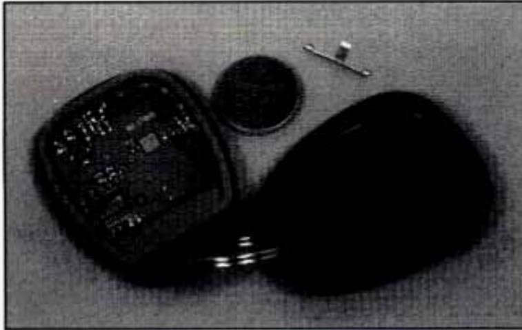
To replace the battery in the Keyless Entry System:
