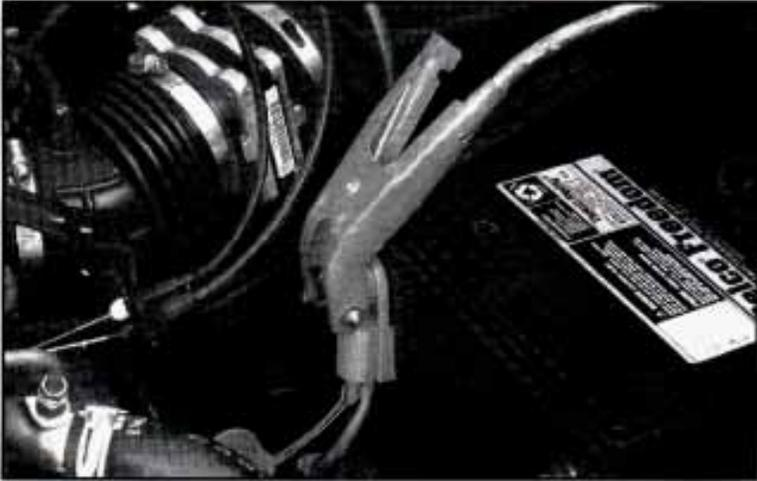
7. Connect the positive (+) cable to the positive (+) terminal of the vehicle with the dead battery. Use a remote positive (+) terminal if the vehicle has one.
