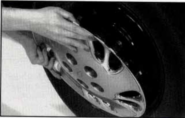
2. Give the cover a sharp pull or gently pry on the edge of the cover to remove it from the wheel.
