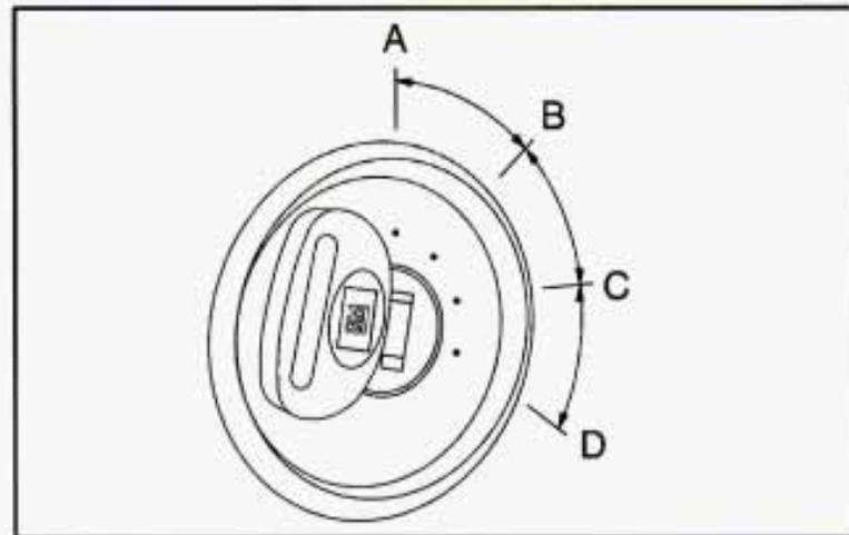
With the ignition key in the ignition switch, you can turn the switch to four positions.
