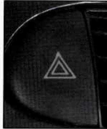
Press the switch once to turn your hazard flashers on. The switch will flash when activated.
