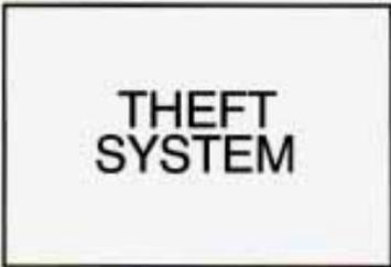
This light will come on briefly when you turn the ignition to ON. The light will stay on until the engine starts.
