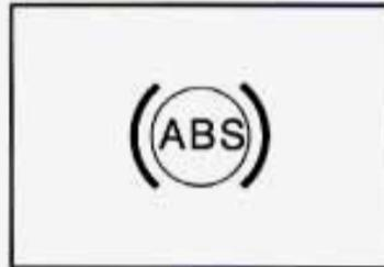
With the anti-lock brake system, this light will come on when you turn your ignition on or start your engine and it will stay on for three seconds. That's normal.
