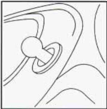
Adjust the driver's side outside mirror with the control lever on the driver's door.
