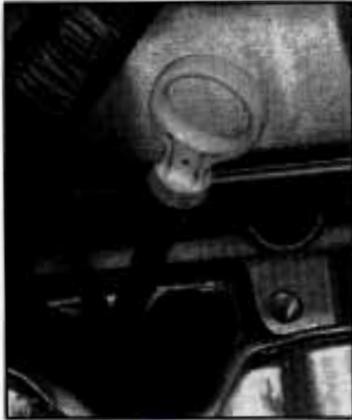
The engine oil dipstick on the 3100 engine is located in front of the engine.
