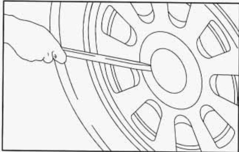
3. Some models are equipped with aluminum wheels. Remove the cover plate to find the wheel nuts. Carefully use the wedge end of the wheel wrench to pry it off.
