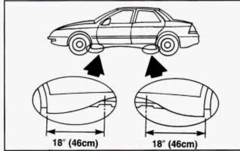
5. Position the jack and raise the jack head until it fits firmly into the notch in the vehicle's frame nearest the flat tire. Put the compact spare tire near you.
