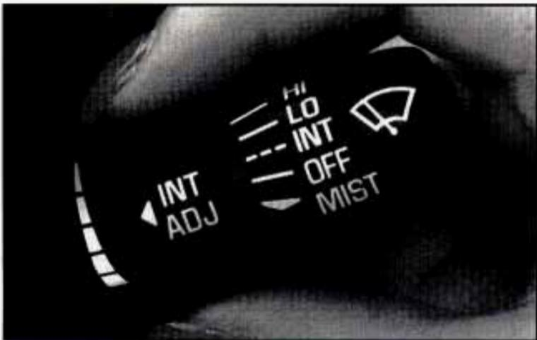
Remember that damaged wiper blades may prevent you from seeing well enough to drive safely. To avoid damage, be sure to clear ice and snow from the wiper blades before using them. If they're frozen to the windshield, carefully loosen or thaw them. If your blades do become damaged, get new blades or blade inserts.
