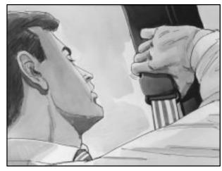
To move it down, squeeze the release button and move the height adjuster to the desired position. You can move the adjuster up just by by pushing up on the shoulder belt guide. After you move the adjuster to where you want it, try to move it down without squeezing the release button to make sure it has locked into position.
