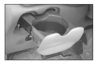
The instrument panel cupholder is located to the left of the steering wheel. To use it, pull it out until the rubber insert is revealed. The insert is removable for easy cleaning.
