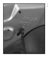
3. Lift the hood, release the hood prop rod from its retainer and put the hood prop into the slot marked PROP ROD.
