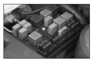
The engine compartment fuse block is located on the driver's side of the engine compartment, near the air cleaner filter.
