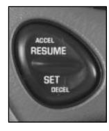
With cruise control, you can maintain a speed of about 25 mph (40 km/h) or more without keeping your foot on the accelerator. This can really help on long trips. Cruise control does not work at speeds below 25 mph (40 km/h).
