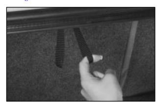
To open the folding rear seat, open the trunk and pull one or both of the tethers located on the left side of the trunk. The left-hand tether will open the larger side of the seatback. The right-hand tether will open the smaller side of the seatback. Once a tether is pulled, the seatback can be pushed open through the trunk, or pulled open from inside the vehicle.
