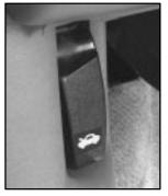
1. To open the hood, first pull the hood release handle inside the vehicle.
