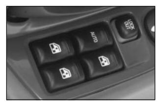
The power window switches are located on the armrest of the driver's door. In addition, each passenger door has a switch for its own window.
