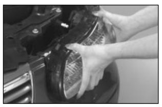
3. Remove the lamp assembly from the vehicle by pulling forward. Use care not to scratch the vehicle with the lamp or the lamp with the fender.
