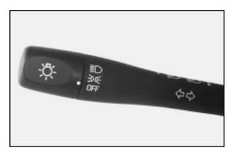
Turn the turn signal lever end cap up one position to turn on:
