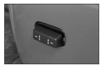
The power seat button is located on the lower left side of the driver's seat. This button allows you to move the seat up, down, forward and backward. It will also move the front of the seat up or down and the rear of the seat up or down. Move the seat higher by lifting and holding the bottom of the button. Lower the seat by pushing and holding the top of the button.
