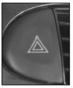
Press the button once to turn your hazard flashers on. The button will flash when activated.
