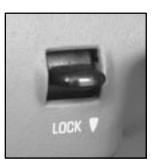
With the power door locks, you can unlock or lock all of the doors of your vehicle from the driver or front passenger door lock switch.
