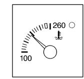
This gage shows the engine coolant temperature. If the gage pointer moves into the red area, the light comes on and you hear a chime, your engine is too hot! It means that your engine coolant has overheated.
