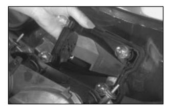
5. Carefully remove the backplate by gently pulling up on the two upper and two lower tabs.
