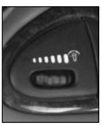
You can brighten or dim the instrument panel cluster lights by rotating the switch, located on the instrument panel, to the left of the steering wheel.
