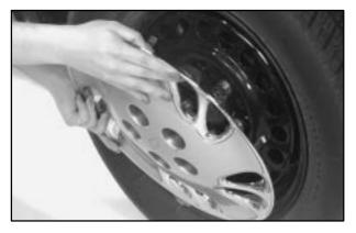
2. Give the cover a sharp pull or gently pry on the edge of the cover to remove it from the wheel.
