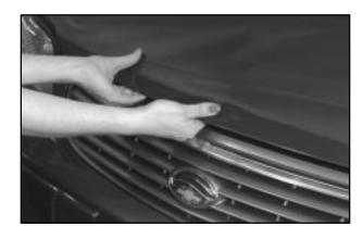
2. Then go to the front of the vehicle and lift the secondary hood release handle before lifting the hood.
