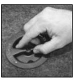
The equipment you'll need is in the trunk. Turn the center retainer nut on the compact spare cover counterclockwise to remove it.
