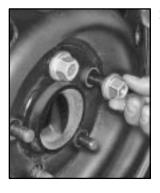
10. Install the compact tire spare. Replace the wheel nuts with the cone end of the nuts toward the wheel. Tighten each nut by hand or with the jack handle until the wheel is held against the hub.
