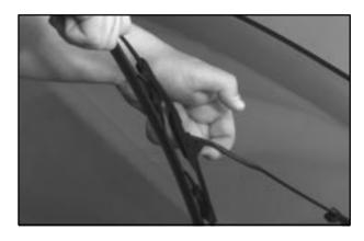
Windshield wiper blades should be inspected at least twice a year for wear and cracking. See "Wiper Blade Check" in Section 7 of this manual under "Owner Checks and Services" for more information. Replacement blades come in different types and are removed in different ways. For the proper type and length, see "Capacities and Specifications" in the Index. Here's how to remove the Shepherd's Hook type:
