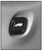
Press the remote trunk release button, located on the lower left side of the instrument panel, to release the trunk lid.
