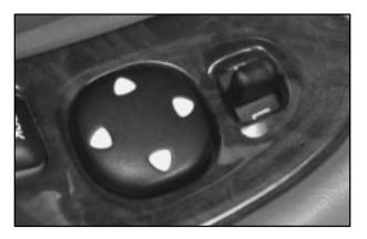
This switch is located on the armrest of the driver's door. Move this switch to the left or right depending on which mirror you need to adjust (center is the off position.) Then adjust the direction of the mirror using the pad marked with arrows just below the selector switch.
