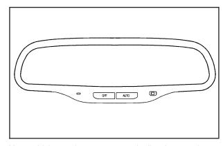
Your vehicle may have an automatic dimming rearview mirror with a compass. This feature enables the mirror to sense nighttime glare from vehicle headlamps from behind and automatically dim to reduce the glare to a safe level.
