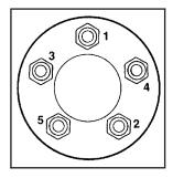
Tighten the wheel nuts firmly in a crisscross sequence, as shown, with the wheel wrench.
