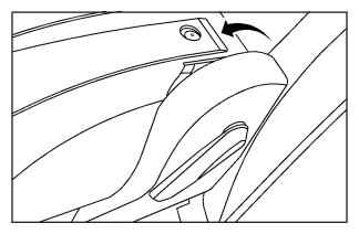
2. Once a lever is pulled, the seatback can be pushed into the down position.
