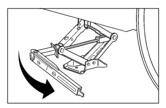
12. Lower the vehicle by turning the wrench counterclockwise. Lower the jack completely.
