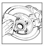
Remove any rust or dirt from the wheel bolts, mounting surfaces and spare wheel. 10. Install the compact spare tire.
