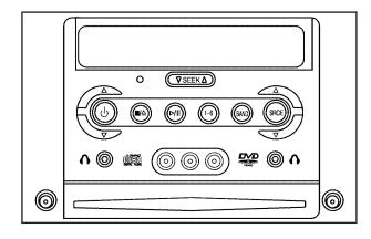
(Power): Press this button to turn the RSE system on and off. The rear speakers will be muted when the RSA power is turned on.
