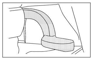
To tilt and telescope the wheel, pull down the lever. Then move the wheel to a comfortable position, pull up the lever to lock the wheel in place. The wheel can be adjusted up and down as well as forward and backward.
