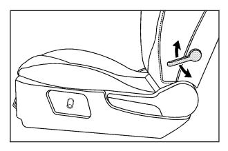
If your vehicle has this feature, the handle is located on the outboard side of the driver's seat. Your vehicle may also have manual lumbar on the front passenger's seat. Move the handle up repeatedly to increase lumbar support. Move the handle down repeatedly to decrease lumbar support.
