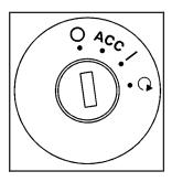
With the key in the ignition switch, you can turn it to four different positions.
