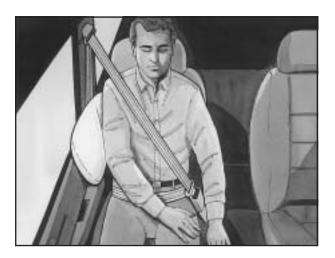
If your vehicle has a seat-mounted side impact airbag for the right front passenger, it is in the side of the passenger's seatback closest to the door.
