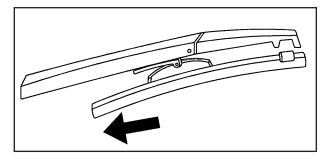
4. Remove clip A, shown above, and slide it into the claw of the wiper blade assembly.
