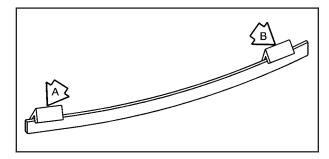
Hold the wiper blade refill with the curved side facing downward.
