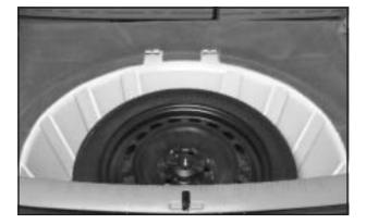
3. Turn the wing nut counterclockwise and remove it. Then remove the compact spare tire. See *Compact Spare Tire on page 5-73* for more information.
