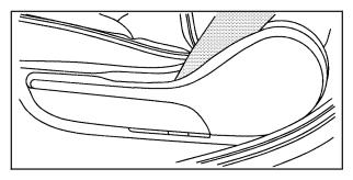
To adjust the seatback, lift the lever located on the outboard side of the seat and move the seatback to the desired position. Release the lever to lock the seatback in place. Push and pull on the seatback to make sure it is locked in place.
