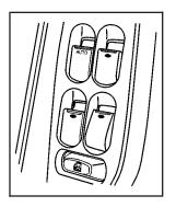
The power window switches are located on the armrest on the driver's door. In addition, each passenger door has a switch for its own window.
