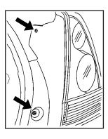
Remove the two fasteners located on the inside of the trunk at the rear of the vehicle.
