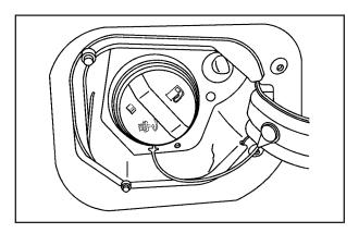
The tethered fuel cap is located behind a hinged fuel door on the passenger's side of the vehicle. To open the door, insert your finger into the finger depression next to the fuel door.
