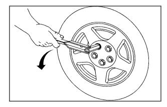
3. Use the wrench to loosen all the wheel nuts. Do not remove them yet.
