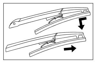
2. Pull the wiper blade out of the wiper blade assembly, as shown.
