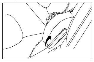
Pull up on and hold the lever located on the side of either rear seat.
