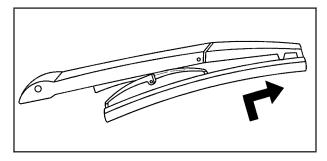
5. Remove clip B, shown above, and slide it into the remaining claw of the wiper blade assembly.
