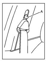
To move it down, push down the release button (A) and move the height adjuster to the desired position. You can move the adjuster up by pushing the release button up. After you move the adjuster to where you want it, try to move it without pushing the release button to make sure it has locked into position.
