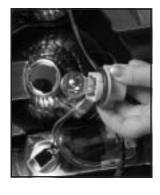
Pull the bulb to remove it from the socket. Replace the old bulb with a new one.
