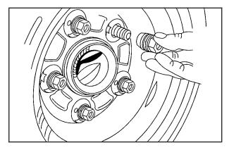
11. Put the wheel nuts back on with the rounded end toward the wheel. Tighten each nut by hand or with the wrench until the wheel is held against the hub.
