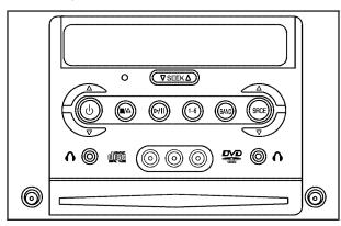
( (Power): Press this button to turn the RSE system on and off.
