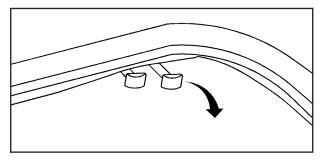
Open the trunk and pull one or both of the gray handles located on the upper part of the trunk opening. The driver's side handle will open the larger side of the seatback. The passenger's side handle will open the smaller side of the seatback. Once a handle is pulled, the seatback can be pushed open through the trunk, or pulled open from inside the vehicle.
