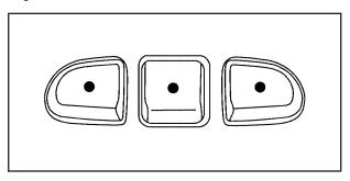
HomeLink, a combined universal transmitter and receiver, provides a way to replace up to three hand–held transmitters used to activate devices such as gate operators, garage door openers, entry door locks, security systems and home lighting. Additional HomeLink information can be found on the Internet at www.homelink.com or by calling 1-800-355-3515.
