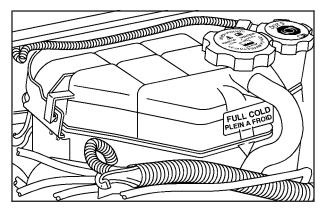
The engine coolant surge tank is located in the rear of the engine compartment. See *Engine Compartment Overview on page 5-12* for more information on location.
