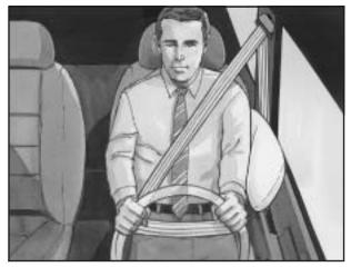
If your vehicle has a seat-mounted side impact airbag for the driver, it is in the side of the driver's seatback closest to the door.
