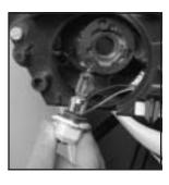
Remove the bulb from the socket. Replace the old bulb with a new bulb.
