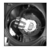
Unclip the wiring harness and twist the socket less than one-quarter turn counterclockwise and remove it.
