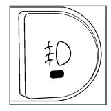
If your vehicle has this feature, the button for the fog lamps is located on the instrument panel, to the left of the steering wheel.
