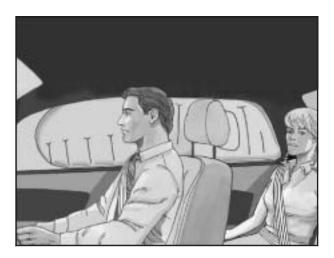
If your vehicle has a roof-mounted side impact airbag for the right front passenger and the person seated directly behind that passenger, it is in the ceiling above the side windows.
