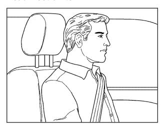
The head restraints on both the front and rear seats are adjustable. Press the button on the side of the post to adjust the head restraint. Slide the head restraint up or down so that the top of the restraint is closest to the top of your head. This position reduces the chance of a neck injury in a crash.
