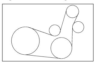
The engine drive belt on this hybrid vehicle is under a higher tension than the engine drive belt on a non-hybrid vehicle and requires the use of a special kind of tool to service. See your dealer/retailer for service.
