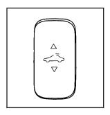
On vehicles with a sunroof, the switch is located on the headliner between the map lamps.
