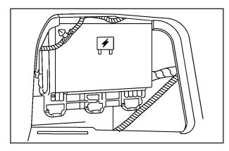
The rear compartment fuse block is located in the trunk of the vehicle. Access the fuse block through the trunk panel on the driver side of the rear cargo area.
