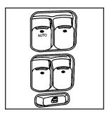
On vehicles with power windows, the switches are on the driver door armrest. Each passenger door has a switch that controls only that window.
