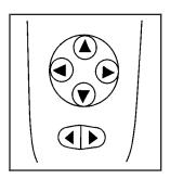
Controls for the outside power mirrors are located on the driver door.
