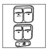
The power window switches are located on the armrest on the driver's door. In addition, there is a switch on each passenger door.
