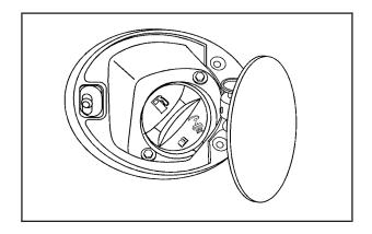
Turn the tethered fuel cap counterclockwise to remove. While refueling, hang the tethered fuel cap from the hook on the fuel door.
