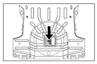
Turn the retainer clockwise and remove the tire sealant and compressor kit.
