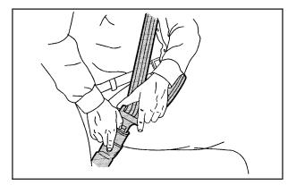
To unlatch the belt, push the button on the buckle. The belt should return to its stowed position. Slide the latch plate up the safety belt webbing when the safety belt is not in use. The latch plate should rest on the stitching on the safety belt, near the guide loop on the side wall.
