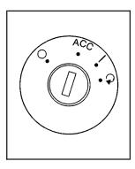
The ignition switch has four different positions.
