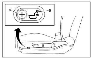
On seats with power lumbar, the control is located on the outboard side of the seat cushion.
