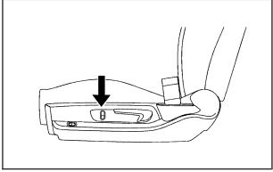
On vehicles with a power lift seat, press the top or bottom of the switch to raise or lower the seat.
