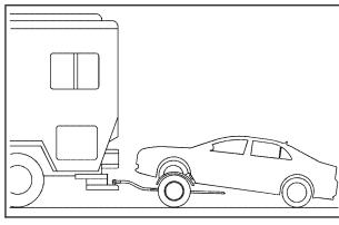
Tow the vehicle with the two rear wheels on the ground and the front wheels on a dolly:
