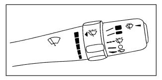
The windshield wiper lever is located on the right side of the steering column.
