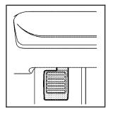
To set the parking brake, push down the parking brake pedal with your left foot. If the ignition is on, the brake system warning light will come on. See Brake System Warning Light on page 4-30.
