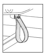
There is an assist handle located on the inside of the trunk.
