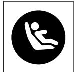
To assist you in locating the lower anchors, each rear anchor position has a label, near the crease between the seatback and the seat cushion.
