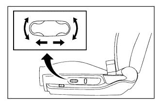
If the vehicle has power seats, the controls used to operate them are located on the outboard side of the seats.
