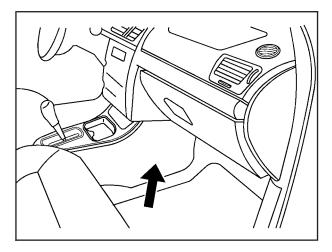
The instrument panel fuse block is located on the instrument panel near the floor on the passenger side of the vehicle.
