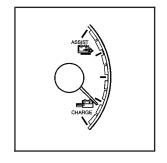
The CHARGE/ASSIST gage displays the charge, into and out of the hybrid battery.
