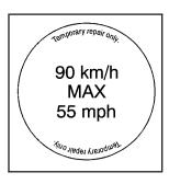
16. If the flat tire was able to inflate to the recommended inflation pressure, remove the maximum speed label from the sealant canister and place it in a highly visible location.
