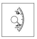
The CHARGE/ASSIST gage displays the charge, into and out of the hybrid battery.
