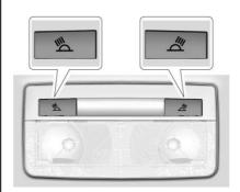
If equipped, the rear reading lamps are in the headliner.
