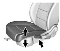
Move the lever on the outboard side of the seat up or down to manually raise or lower the seat.
