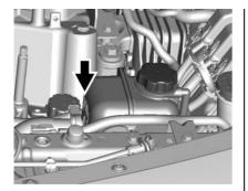
Check to see if coolant is visible in the power electronics coolant reservoir. If coolant is visible but the coolant level is below the cold fill line, there could be a leak in the cooling system.
