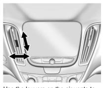
Use the louvers on the air vents to change the direction of the airflow, or to open and close off the airflow.
