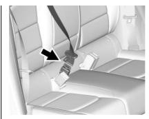
Disconnect the rear safety belt mini-latch, using a key in the slot on the mini-buckle.
