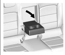
The rear seat has an armrest in the center of the seatback. Lower the armrest to access the two cupholders.
