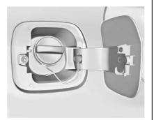
Turn the fuel cap counterclockwise to remove. While refueling, hang the fuel cap from the hook on the fuel door. Reinstall the cap by turning it clockwise until it clicks.
