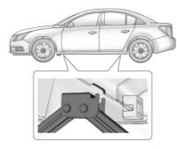
Position the jack lift head at the jack location nearest the flat tire. The location is indicated by a notch on the bottom edge of the body side. The notches in the jack must align with the notch in the rocker pinch weld. The jack lift head lifts on the inward side of the pinch weld flange.
