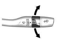
**INT**: Move the lever up to INT for intermittent wipes, then turn the band up for more frequent wipes or down for less frequent wipes.
