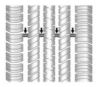
Treadwear indicators are one way to tell when it is time for new tires. Treadwear indicators appear when the tires have only 1.6 mm (1/16 in) or less of tread remaining. See *Tire Inspection* ⇔ 332 and *Tire Rotation* ⇔ 332.
