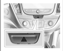
ightharpoonup : Press this button to make the front and rear turn signal lamps flash on and off. Press again to turn the flashers off.
