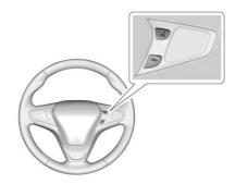
□É: If equipped with OnStar® or a Bluetooth® system, press to interact with those systems. See OnStar Overview ⇒ 399, Bluetooth (Overview) ⇒ 183 or Bluetooth (Infotainment Controls Radio with Touchscreen) ⇒ 189 or Bluetooth (Infotainment Controls Radio without Touchscreen) ⇒ 185, or "Bluetooth (Overview)" in the infotainment manual.
