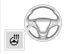
: If equipped with a heated steering wheel, press to turn on or off. A light on the button displays when the feature is turned on.
