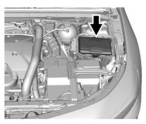
The engine compartment fuse block is on the driver side of the engine compartment.
