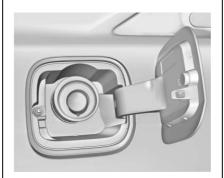
The hybrid vehicle has a capless refueling system and does not have a fuel cap. The filling nozzle must be fully inserted and latched prior to starting fuel flow.
