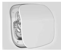
The fuel cap is behind a hinged fuel door on the passenger side of the vehicle. To open the fuel door, push and release the rearward center edge of the door.
