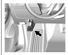
To set the parking brake, if equipped. Hold the regular brake pedal down, then push the parking brake pedal down.
