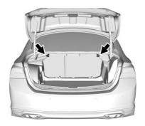
Open the trunk and pull the seatback release lever to fold the rear seat.
