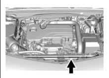
Lift the hood and pull the prop rod by the sleeve from the retainer, located above the radiator.
