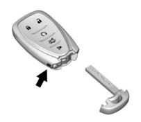
To remove the key, press the button near the bottom of the transmitter, and pull the key out. Never pull the key out without pressing the button.
