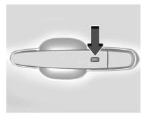
The RKE transmitter must be within 1 m (3 ft) of the trunk or door being opened. Press the button on the door handle to open. See "Keyless Access Operation" in *Remote Keyless Entry (RKE) System Operation* ⇒ 30.
