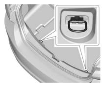
There are cargo tie-downs in the trunk. The cargo tie-downs can be used to secure small loads or the convenience net. See *Convenience Net* ▷ *106*.
