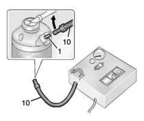
Attach the air only hose (10) to the sealant canister inlet valve (1) by turning it clockwise until tight.
