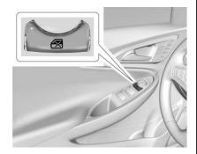
This feature stops the rear door passenger window switches from working.
