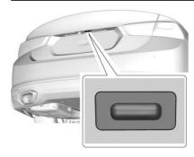
Press the touch pad on the rear of the trunk after unlocking all doors.
