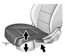
Move the lever on the outboard side of the seat up or down to manually adjust the seat height.
