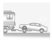
Tow the vehicle with the two rear wheels on the ground and the front wheels on a dolly.
