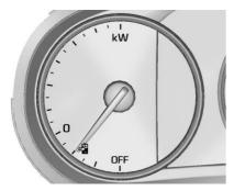
The power gauge indicates the vehicle's power usage in propelling or slowing the vehicle. The green area indicates regenerative braking. The white area indicates power provided by the engine and/or battery. The yellow area shows high power usage. Operating the vehicle
