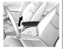
The center console has storage under the armrest. Pull up the latch and lift to open.
