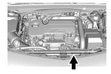
Lift the hood and pull the prop rod by the sleeve from the retainer, located above the radiator.
