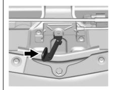
Go to the front of the vehicle to find the secondary release handle. The handle is under the front edge of the hood near the center. Slide the secondary hood release handle toward the driver side of the vehicle.
