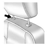
The height of the head restraint can be adjusted. Pull the head restraint up to raise it. Try to move the head restraint to make sure that it is locked in place.
