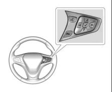
△ or ▽: Press to move up or down in a list, or on the main view press to cycle through the different Info app pages.
