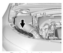
The electrical cord is on the passenger side of the engine compartment, between the fender and the air cleaner.
