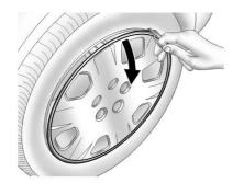
Take off the wheel cover or center cap, if the vehicle has one, to reach the wheel bolts.
