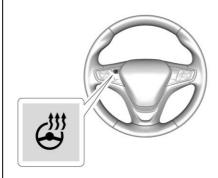
: If equipped with a heated steering wheel, press to turn on or off. A light on the button displays when the feature is turned on. The steering wheel takes about three minutes to start heating.
