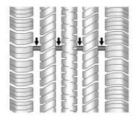
Treadwear indicators are one way to tell when it is time for new tires. Treadwear indicators appear when the tires have only 1.6 mm (1/16 in) or less of tread remaining. See *Tire Inspection* ♀ 291 and *Tire Rotation* ♀ 291.
