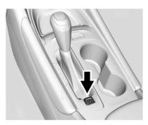
The vehicle may have an Electric Parking Brake (EPB). The EPB can always be activated, even if the ignition is off. To prevent draining the battery, avoid repeated cycles of the EPB system when the engine is
