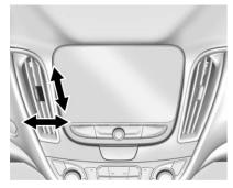
Use the louvers on the air vents to change the direction of the airflow.
