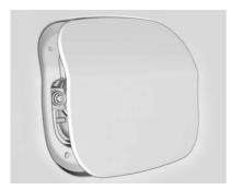
The fuel door is on the passenger side of the vehicle. To open the fuel door, push and release the rearward center edge of the door.
