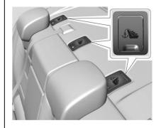
The top tether anchors are under the covers, behind the rear seat, on the filler panel. Be sure to use an anchor on the same side of the vehicle as the seating position where the child restraint will be placed.
