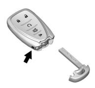
Press the button on the side of the RKE transmitter near the bottom and pull the key out. Never pull the key out without pressing the button.
