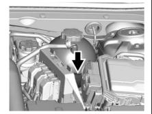
1.5L L4 Turbo and 2.0L L4 Turbo Coolant Surge Tank
