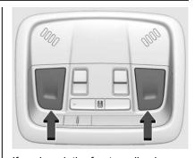
If equipped, the front reading lamps are in the overhead console.
