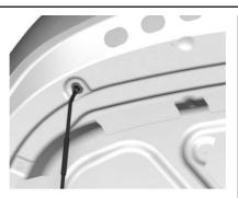
Securely place the hood prop rod into the slot on the underside of the hood.
