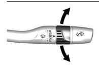
**INT:** Move the lever up to INT for intermittent wipes, then adjust the band to control the frequency of wipes.
