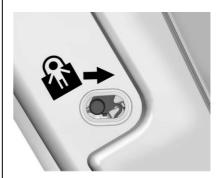
If equipped, the safety lock is on the inside edge of the rear doors. To use the safety lock:
