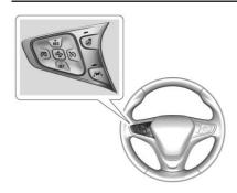
(S): Press to turn the system on or off. A white cruise control indicator comes on in the instrument cluster.
