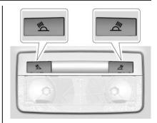
If equipped, the rear reading lamps are in the headliner.
