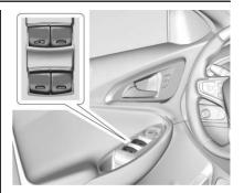
The power windows work when the vehicle is on, in ACC/ACCESSORY, or when Retained Accessory Power (RAP) is active. See Retained Accessory Power (RAP)
