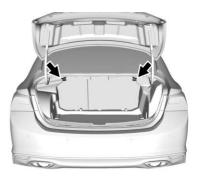
Open the trunk and pull the seatback release lever to fold the rear seat.
