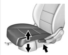
Move the lever on the outboard side of the seat up or down to manually raise or lower the seat.
