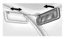
Pull the sun visor down to block glare. Detach the sun visor from the center mount to pivot to the side window, or to extend along the rod.
