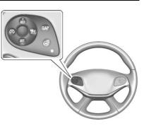
☆ : Press to turn the system on or off. A white Adaptive Cruise Control indicator comes on.
