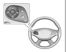
S: Press to turn cruise control on or off. A white indicator comes on in the instrument cluster when cruise is on. **+RES** : If there is a set speed in memory, press briefly to resume to that speed or press and hold to accelerate. If cruise control is already active, use to increase vehicle speed.
