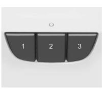
This system provides a way to replace up to three remote control transmitters used to activate devices such as garage door openers, security systems, and home automation devices.
