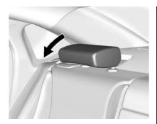
Always adjust the head restraint so that the top of the restraint is at the same height as the top of the occupant's head.
