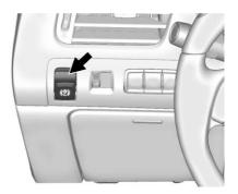
The Electric Parking Brake (EPB) switch is on the left side of the instrument panel. The EPB can always be activated, even if the ignition is off. To prevent draining the battery, avoid repeated cycles of the EPB when the engine is not running.
