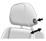
To adjust the head restraint forward or rearward, press the button located on the side facing of the head restraint and move it forward or rearward until the desired locking position is reached. Try to move the head restraint after the button is released to make sure that it is locked in place.
