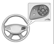
Some audio controls can be adjusted at the steering wheel.
