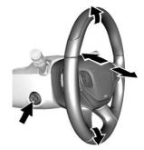
If equipped, press the control to move the steering wheel up and down or forward and rearward.
