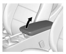
Press the button and lift to access. There is a removable tray on the top of the console. There is an auxiliary input jack, USB port(s), and accessory power outlet inside.
