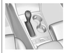
**P**: This position locks the front wheels. It is the best position to use when you start the engine because the vehicle cannot move easily.
