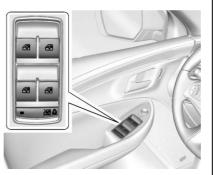
The power windows only operate with the ignition in ACC/ ACCESSORY or ON/RUN/START, or when Retained Accessory Power (RAP) is active. See *Retained Accessory Power* (*RAP*) ⇔ 209. Press or pull the switch to open or close the window.
