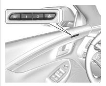
If equipped, the 1, 2, SET, and (Exit) buttons on the driver door are used to manually store and recall memory settings for the driver seat, outside mirrors, and power tilt and telescoping steering column, if equipped.
