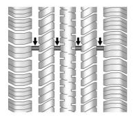
Treadwear indicators are one way to tell when it is time for new tires. Treadwear indicators appear when the tires have only 1.6 mm (1/16 in) or less of tread remaining. See *Tire Inspection*  $\Rightarrow$  297 and *Tire Rotation*  $\Rightarrow$  297.
