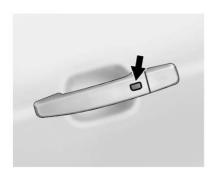
If equipped, use the Keyless Access system to lock and unlock the door. When the doors are locked and the Remote Keyless Entry (RKE) transmitter is within 1 m (3 ft) of the driver door handle, press the lock/ unlock button. When unlocking from the driver door, the first press unlocks that door; press again within five seconds to unlock all passenger doors. See *Remote Keyless Entry (RKE) System Operation* \$ 30.
