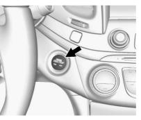
The vehicle may have an electronic keyless ignition with pushbutton start.
