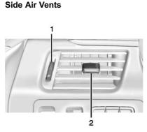
Move the thumbwheels (1) up or down to open or close off the airflow.
