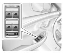
The windows work when the vehicle is in ON/RUN, ACC/ACCESSORY, or Retained Accessory Power (RAP). See *Retained Accessory Power (RAP)* ⇔ 209.
