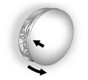
The fuel cap is behind the fuel door on the passenger side of the vehicle. To open the fuel door, push and release the rearward center edge of the door.
