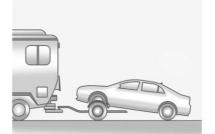
Tow the vehicle with the two rear wheels on the ground and the front wheels on a dolly.
