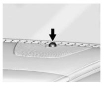
If equipped with the anti-theft alarm system, the indicator light, on the instrument panel near the windshield, indicates the status of the system.
