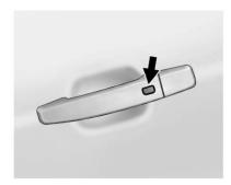
If equipped, use the Keyless Access system to lock and unlock the door. When the doors are locked and the Remote Keyless Entry (RKE) transmitter is within 1 m (3 ft) of the driver door handle, press the lock/ unlock button. When unlocking from the driver door, the first press unlocks that door; press again within five seconds to unlock all passenger doors. See *Remote Keyless Entry (RKE) System Operation*  $\Leftrightarrow$  30.
