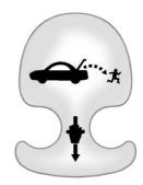
If equipped, there is a glow-in-the-dark emergency trunk release handle on the trunk lid. This handle will glow following exposure to light. Pull the release handle to open the trunk from the inside.
