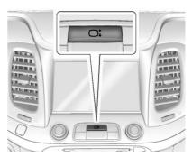
If equipped with storage behind the radio, press  $\bigcirc_{\bullet}^{\bullet}$  and hold to open. There is a USB port inside. See USB Port  $\Leftrightarrow$  165.
