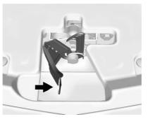
2. Go to the front of the vehicle to find the secondary hood release handle. The handle is under the front edge of the hood near the center. Push the handle to the right and at the same time raise the hood. To close the hood:
