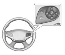
$\triangle$  or  $\nabla$ : Press to move up or down in a list, or on the main view press to cycle through the different Info app pages.
