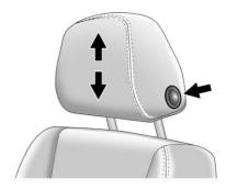
To raise or lower the head restraint, press the button located on the side of the head restraint, and pull up or push the head restraint down and release the button. Pull and push on the head restraint after the button is released to make sure it is locked in place.
