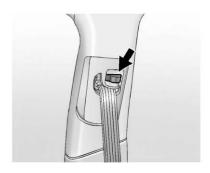
Push down on the release button and move the height adjuster to the desired position. The adjuster can be moved up by pushing the slider/ trim up. After the adjuster is set to the desired position, try to move it down without pushing the release button to make sure it has locked into position.
