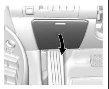
If equipped with storage behind the fuse box, push on the cover and release to open.
