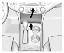
Push the cover down and release to access. To close, push the cover again and release. There is an accessory power outlet inside.
