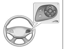
$\triangle$  or  $\nabla$ : Press to move up or down in a list, or on the main view press to cycle through the different Info app pages.
