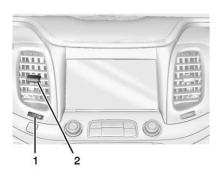
Move the thumbwheels (1) left or right to open or close off the airflow.
