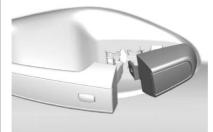
2. Insert the two tabs (7) at the back of the cap (8) between the seal (5) and the metal base (6).
